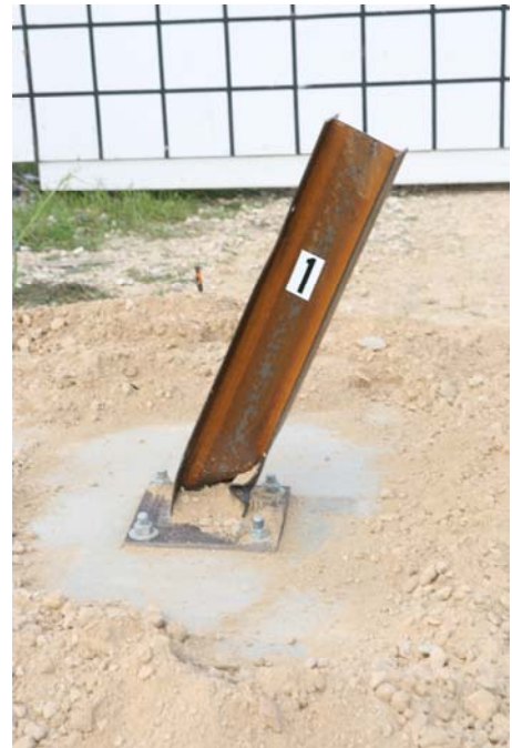
Figure D2. Steel posts over underground structure with 60-inch concrete footing after test 405160-12 P1.
