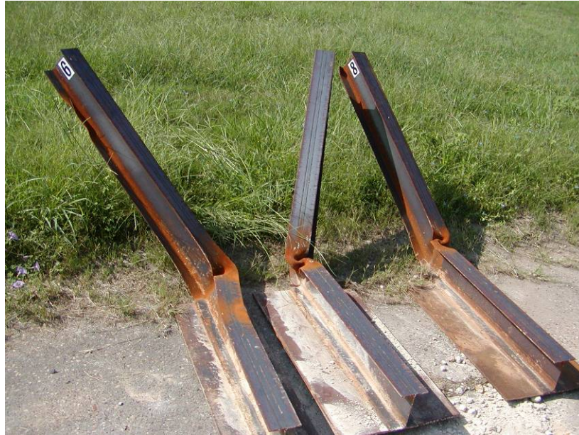
Figure 5 Deformed posts after test 6, 7 and 8.
