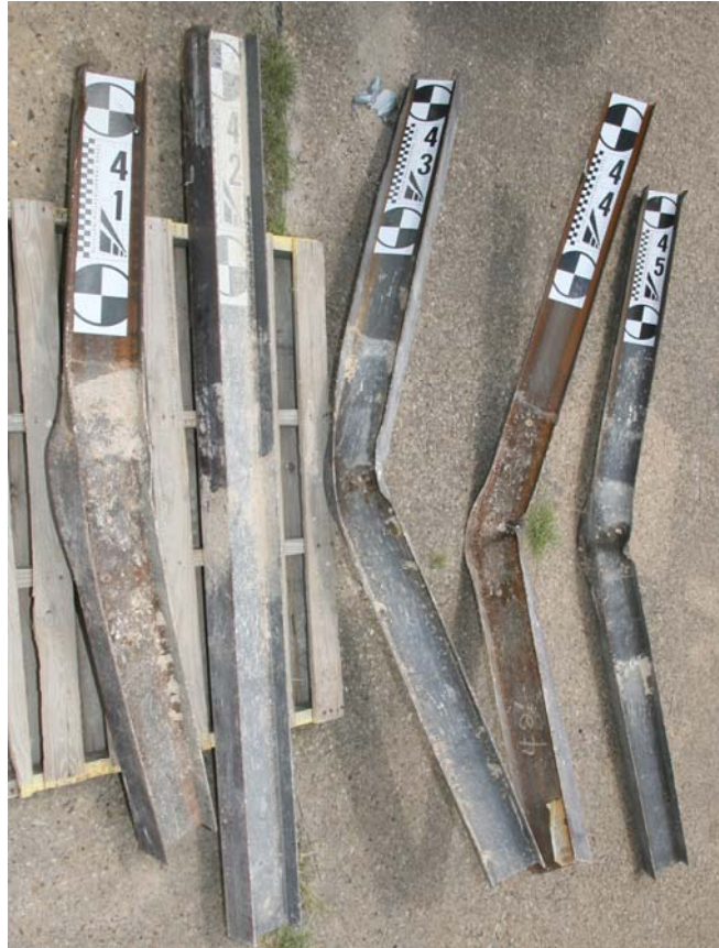
Figure 2 Extract posts after bogie tests
