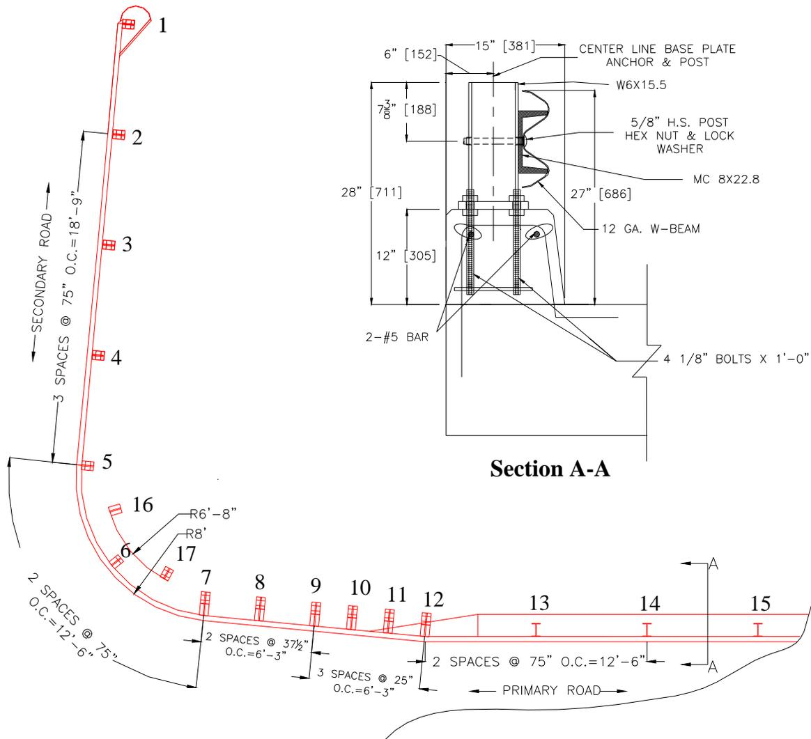
**Figure 2.2 Modified Yuma County test T-intersection installation for Test YC-4 through YC-7**
