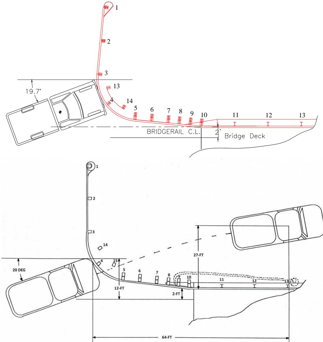
**Figure 2.9 Test YC-3 (1982 Chevrolet P/U, 5380 lb pickup, 44.8 mph, and 19.7 degrees)
