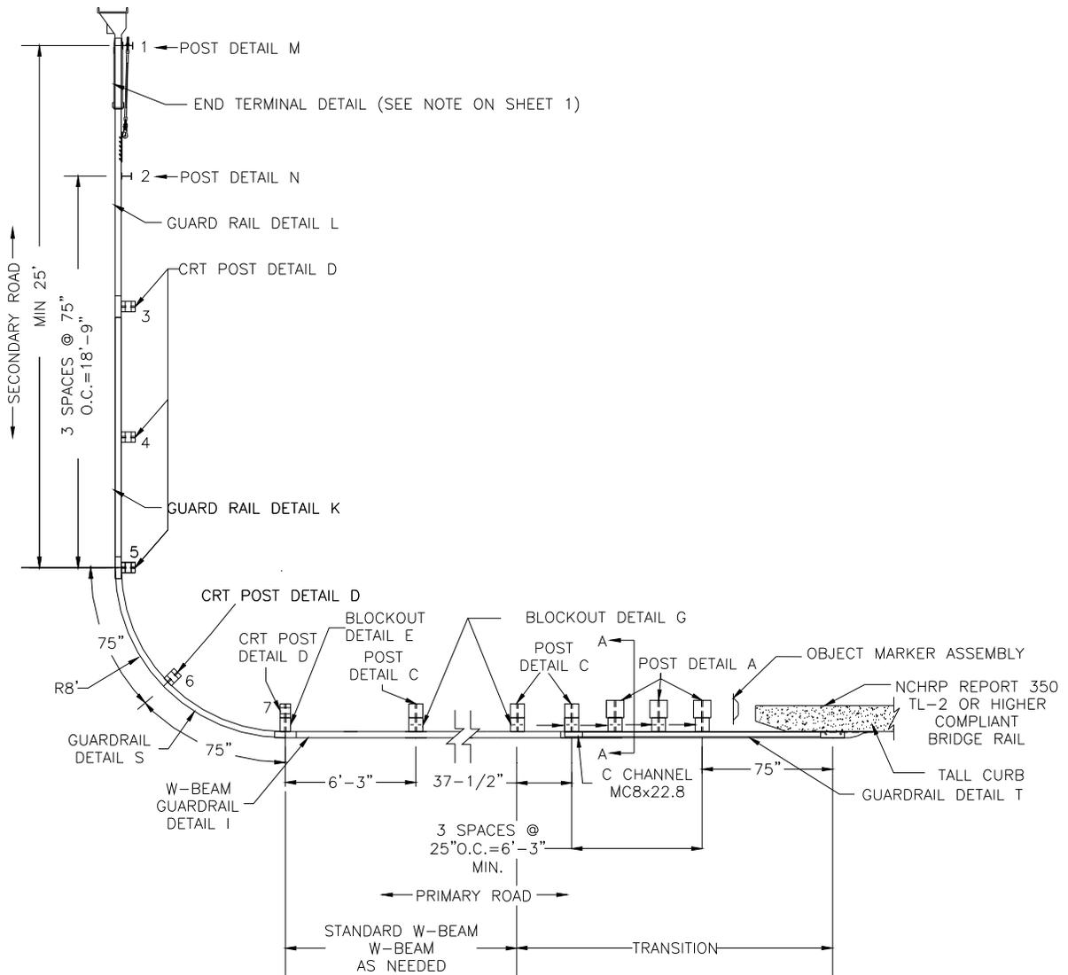
**Figure 6.2 Acceptable variation of the recommended T-intersection system**
