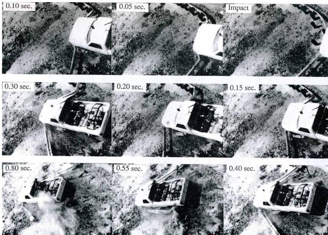
Figure 2.11 Overhead impact sequence photographs, Test YC-3 (3)
