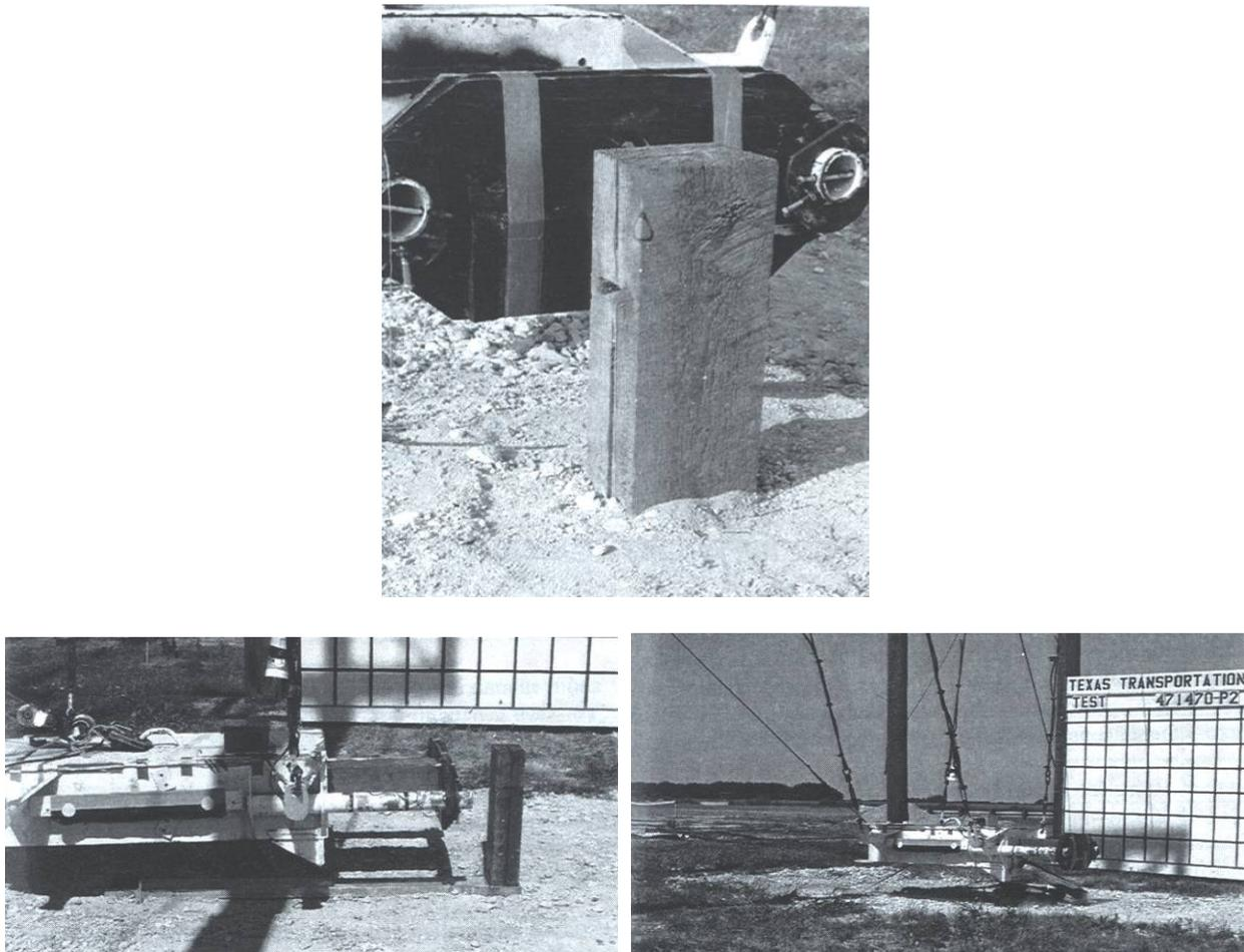
**Figure 4.1 Pendulum equipment used for impact test**
