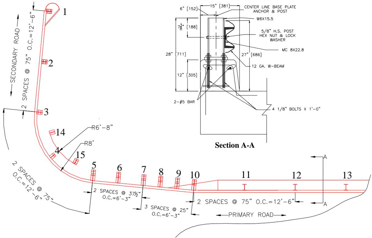
**Figure 2.1 Yuma County test T-intersection installation for Test YC-1 through YC-3**
