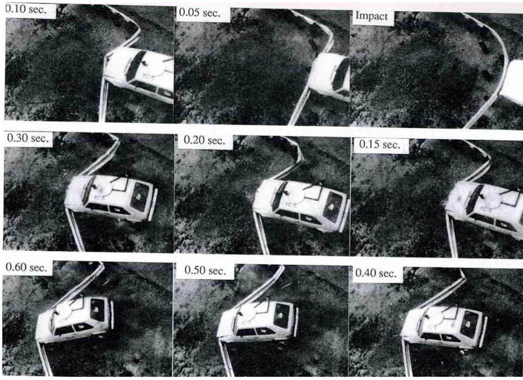
**Figure 2.17 Overhead impact sequence photographs, Test YC-5 (3)**
