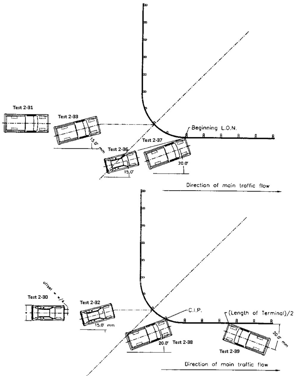
**Figure 1.1 Crash test matrix for short-radius guardrail based on NCHRP Report 350 Table 3.2 (6)**
