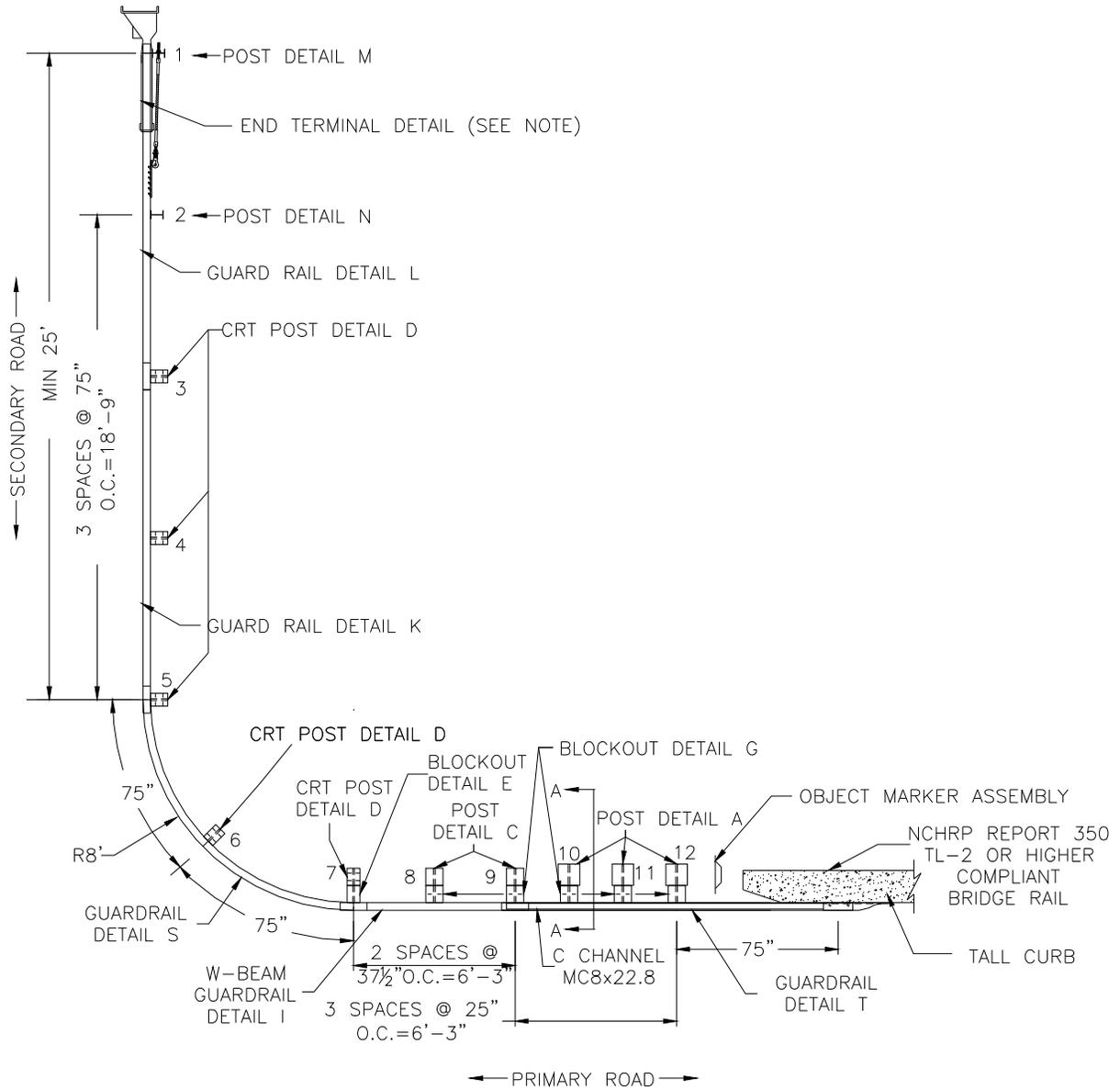
**Figure 6.1 Recommended T-intersection system**
