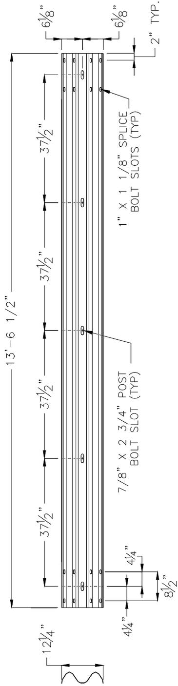
CURVED W-BEAM GUARDRAIL @ NODE SECTION
