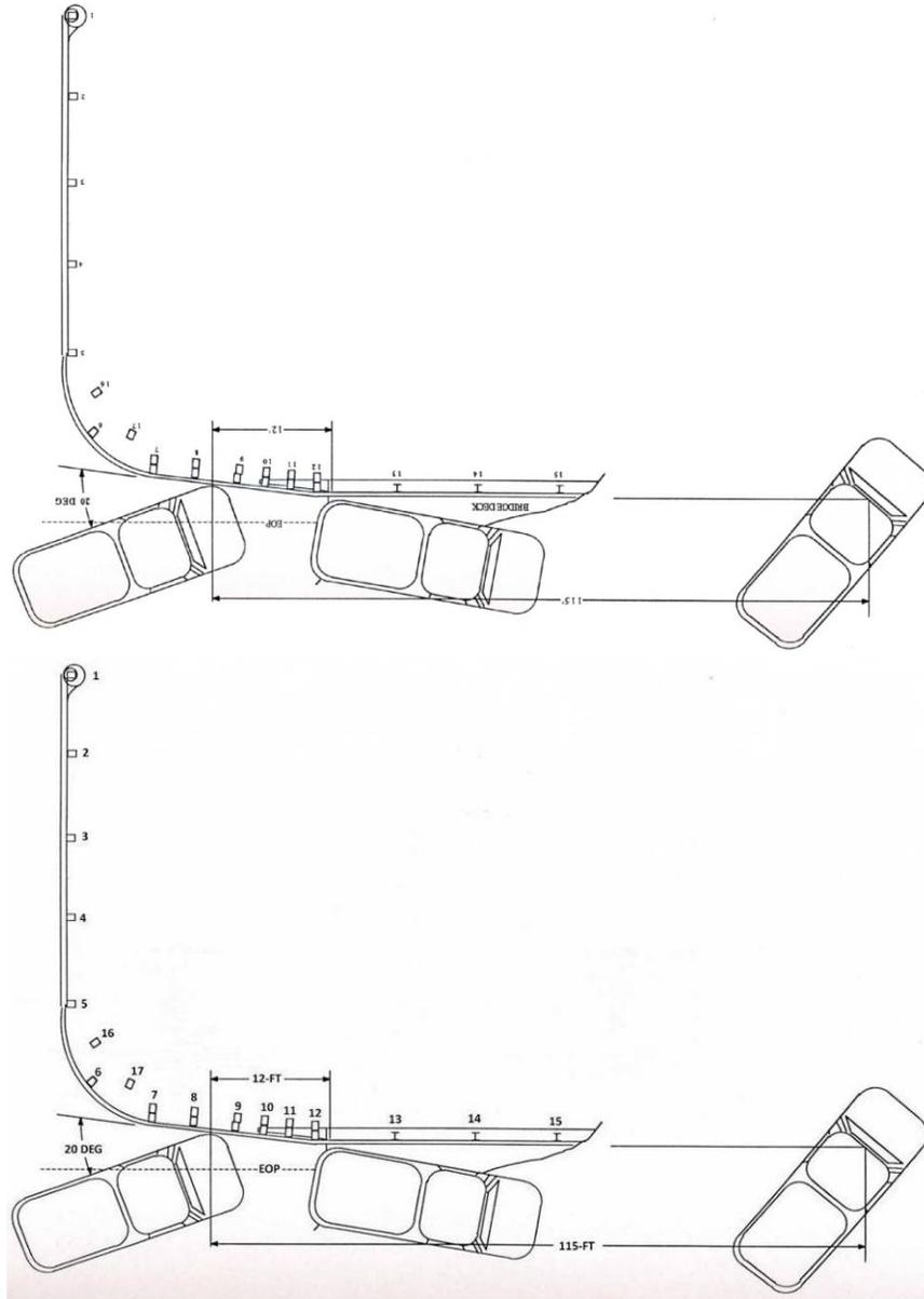
**Figure 2.21 YC-7 (1982 Chevrolet P/U, 5424 lb pickup, 45.2 mph, and 20.7 degrees)
