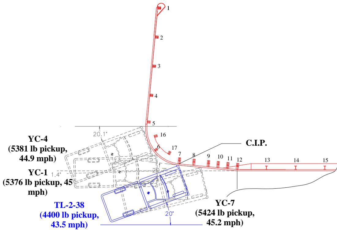
Figure 3.5 NCHRP Report 350 Test 2-38 along with YC-4 and YC-7 tests.
