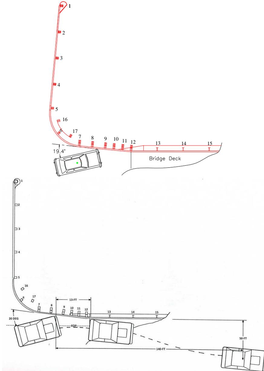
**Figure 2.18 YC-6 (1982 V.W. Rabbit, 1980 lb mini car, 51.1 mph, and 19.4 degrees) -passed for structural adequacy and vehicle trajectory -marginals for occupant risk (3)**
