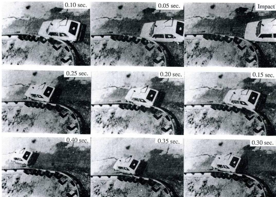
Figure 2.8 Overhead impact sequence photographs, Test YC-2 (3)
