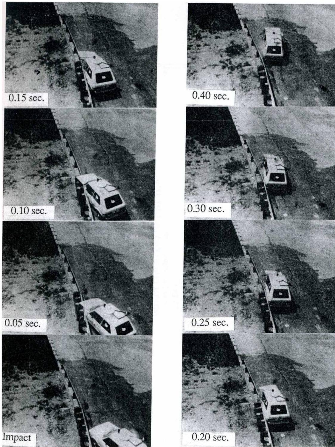
Figure 2.20 Overhead impact sequence photographs, Test YC-6 (3)
