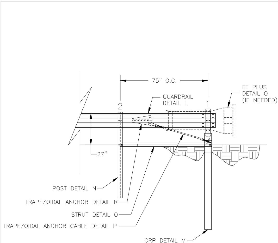
SINGLE SPAN WITH POSITIVE ANCHOR
