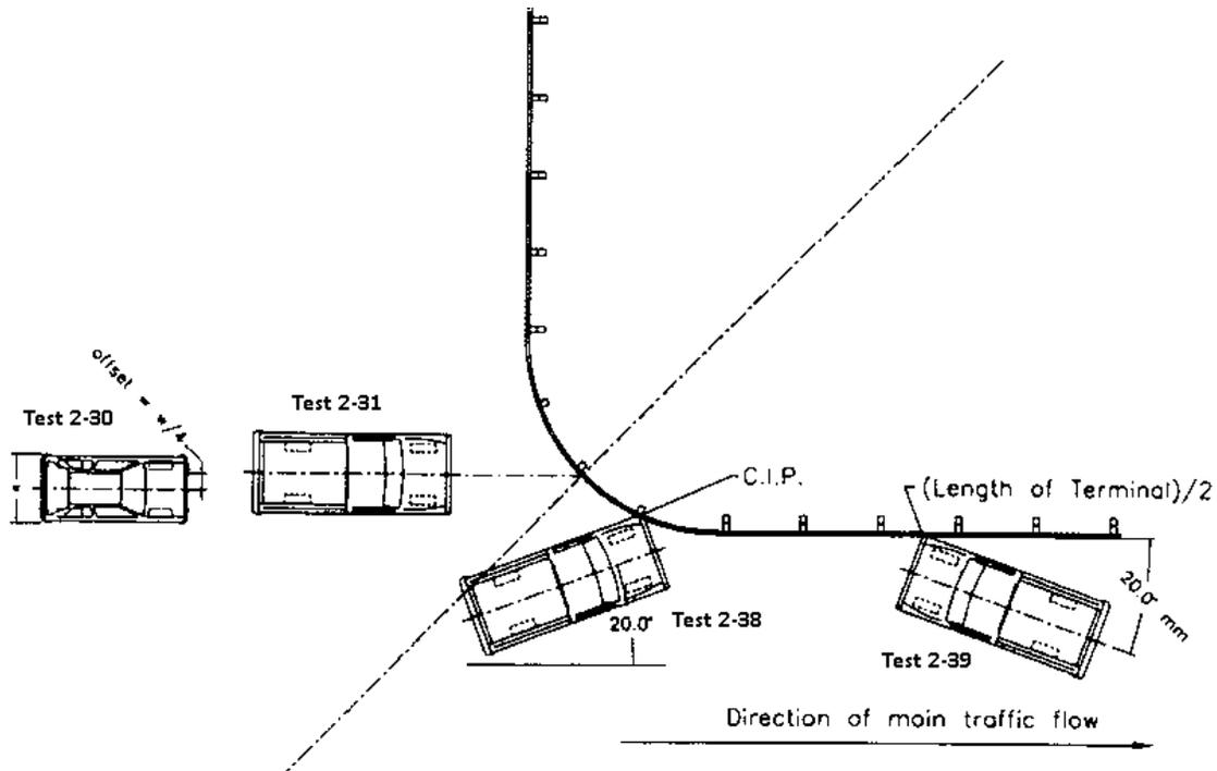
**Figure 3.2 Remaining NCHRP Report 350 test conditions**
