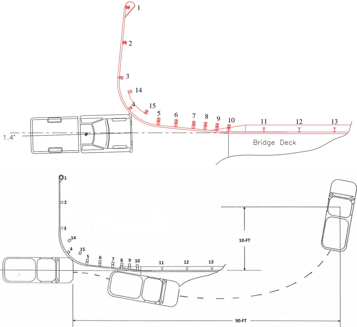
**Figure 2.3 Test YC-1 (1982 Chevrolet P/U, 5376 lb pickup, 45 mph, and 1.4 degrees)
