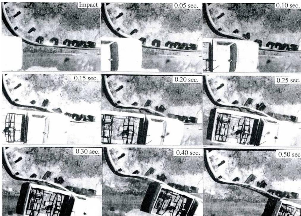
**Figure 2.5 Overhead impact sequence photographs, Test YC-1 (3)**
