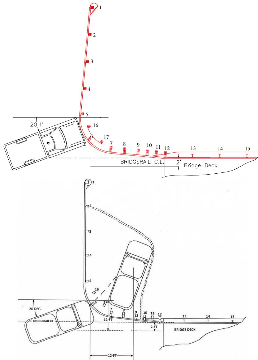
**Figure 2.12 YC-4 (1982 Chevrolet P/U, 5381 lb pickup, 44.9 mph, and 20.1 degrees) -passed for structural adequacy, occupant risk, and vehicle trajectory (H, I) (3)**
