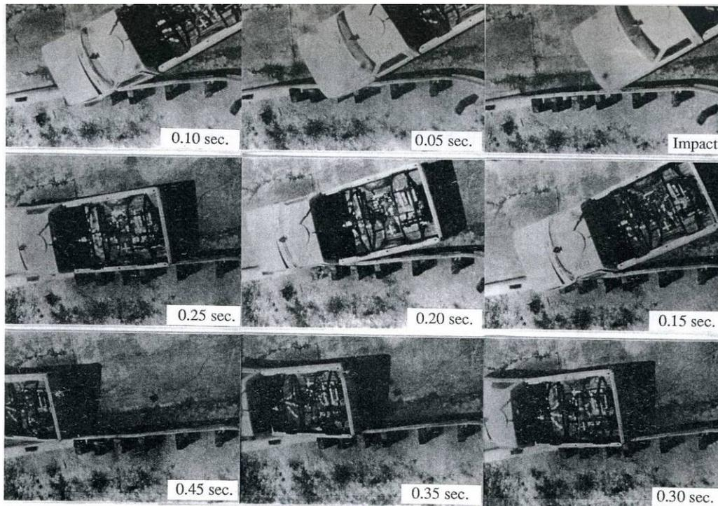
Figure 2.23 Overhead impact sequence photographs, Test YC-7 (3)
