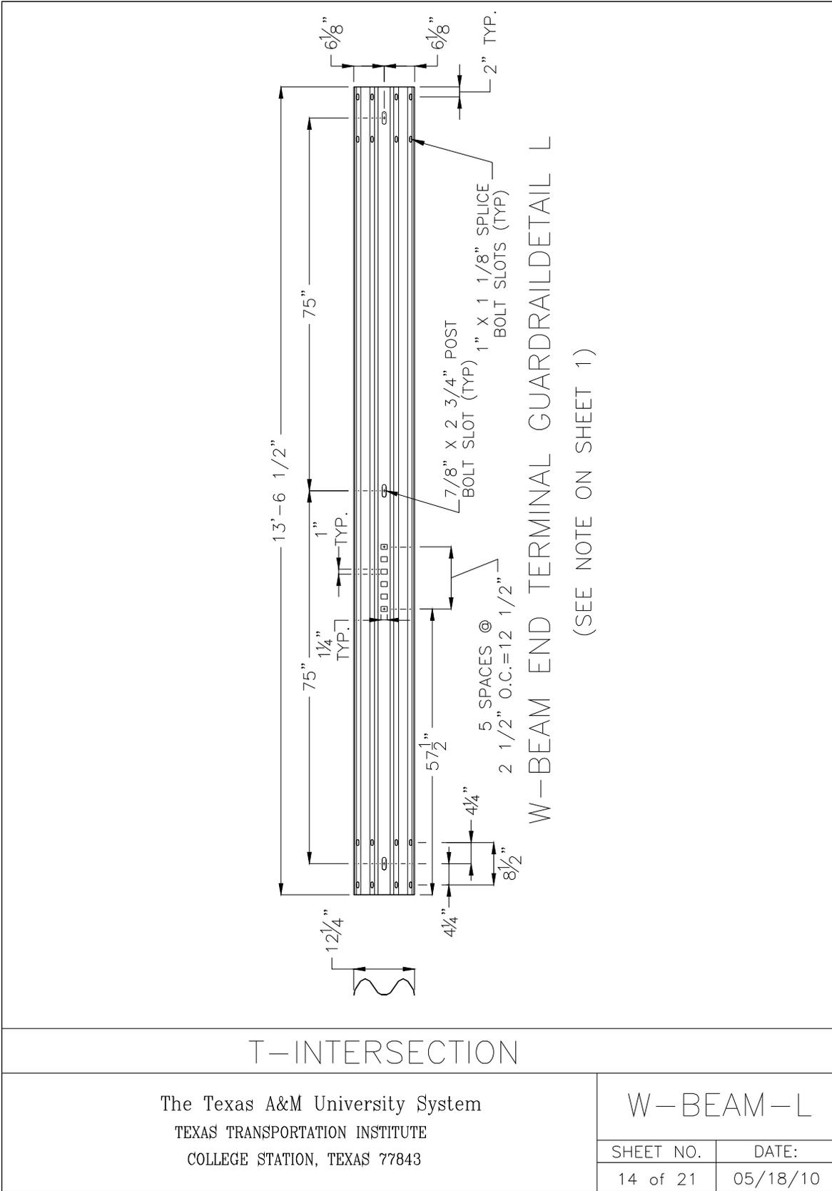
**Figure A 14 W-beam terminal guardrail L**
