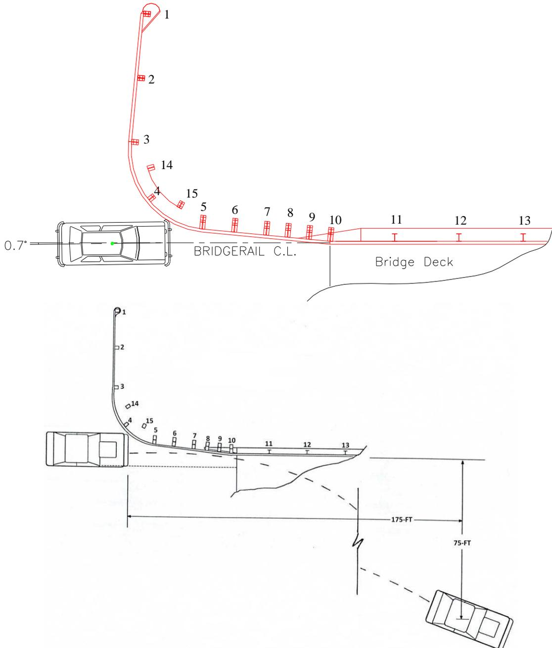
**Figure 2.6 Test YC-2 (1982 V.W. Rabbit, 1978 lb mini car, 50.3 mph, and 0.7 degrees) -passed for structural adequacy, occupant risk, and vehicle trajectory (3)**
