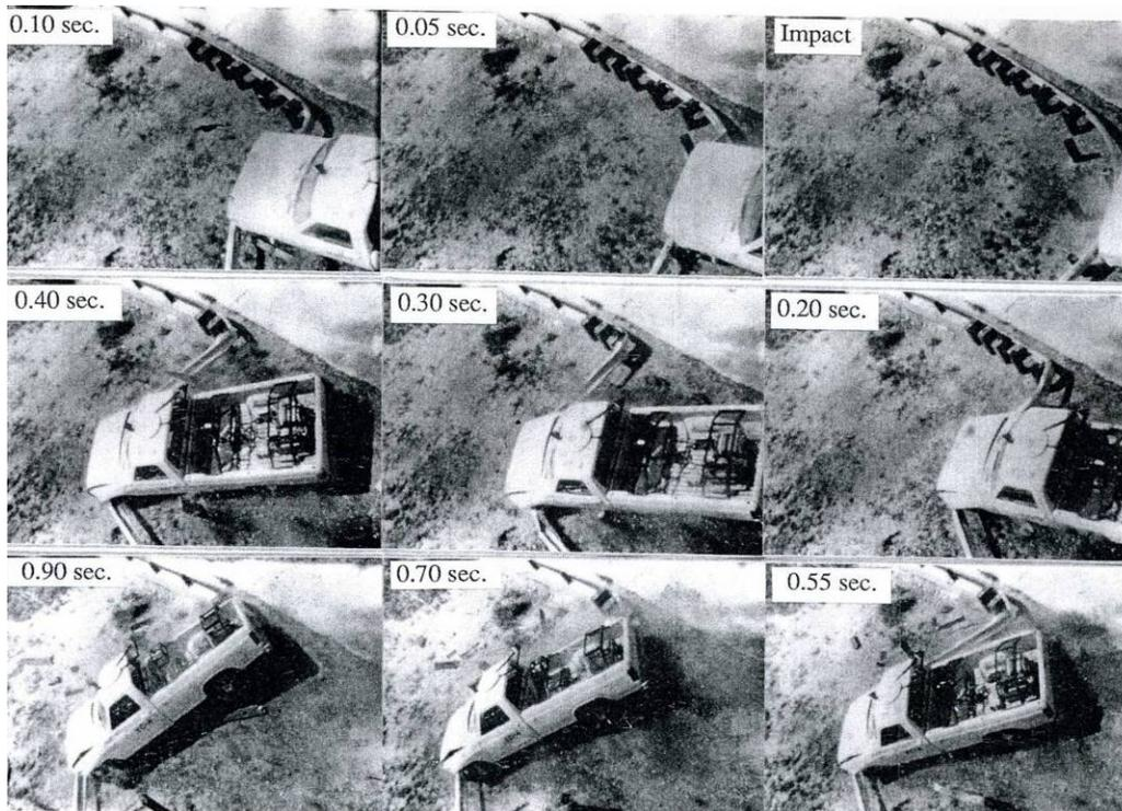
Figure 2.14 Overhead impact sequence photographs, Test YC-4 (3)
