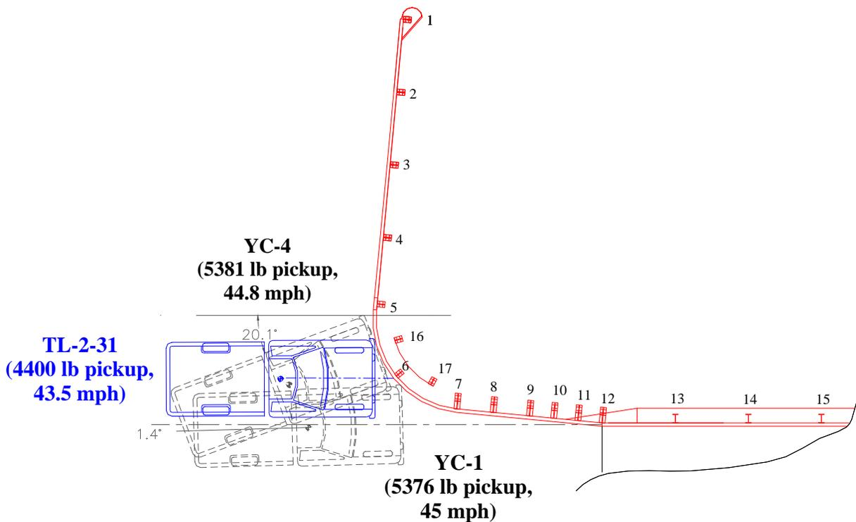
Figure 3.4 NCHRP Report 350 Test 2-31 along with YC-1 and YC-4 tests
