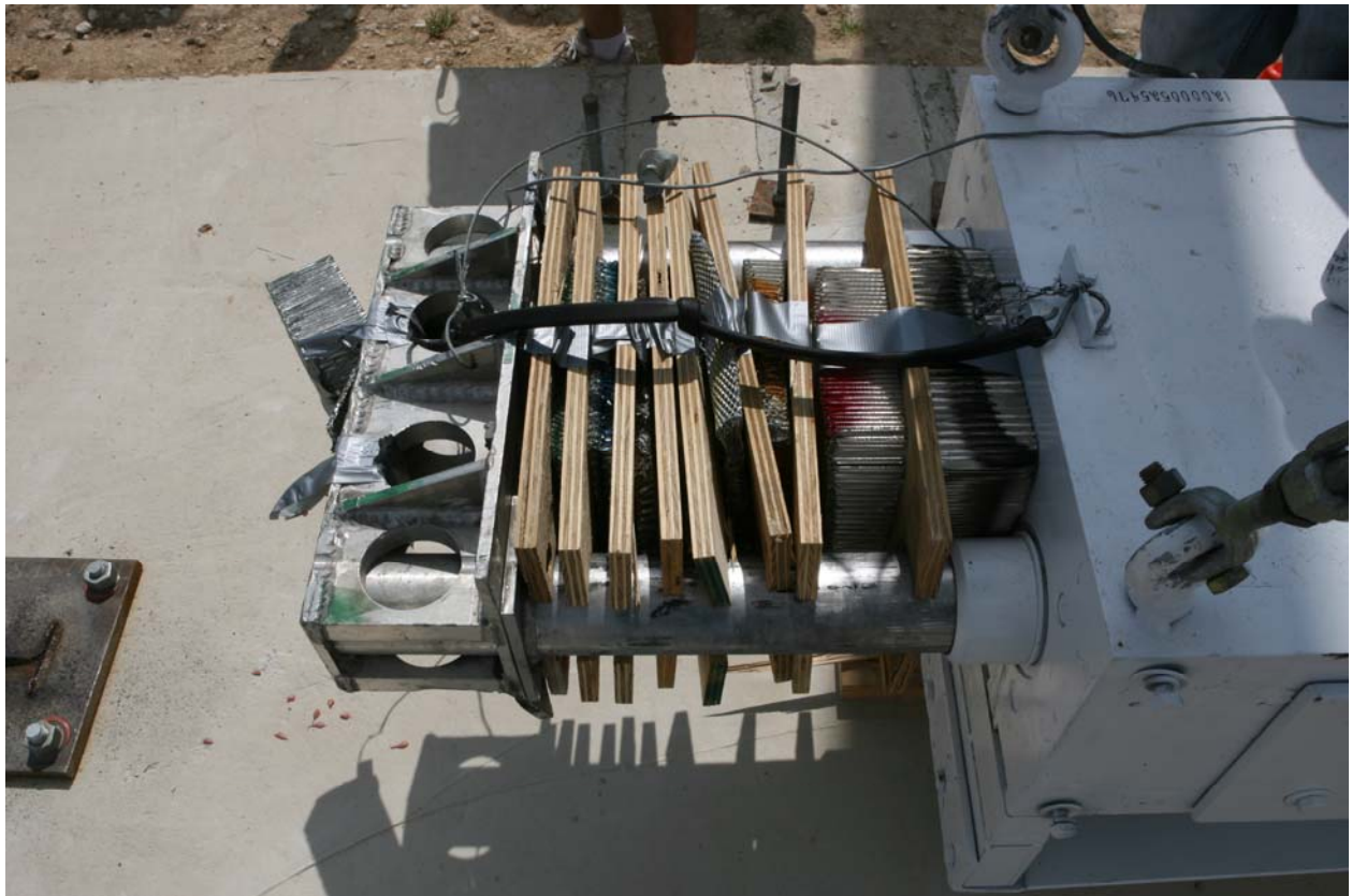
Figure E6. Pendulum bogie nose before and after test P2.
