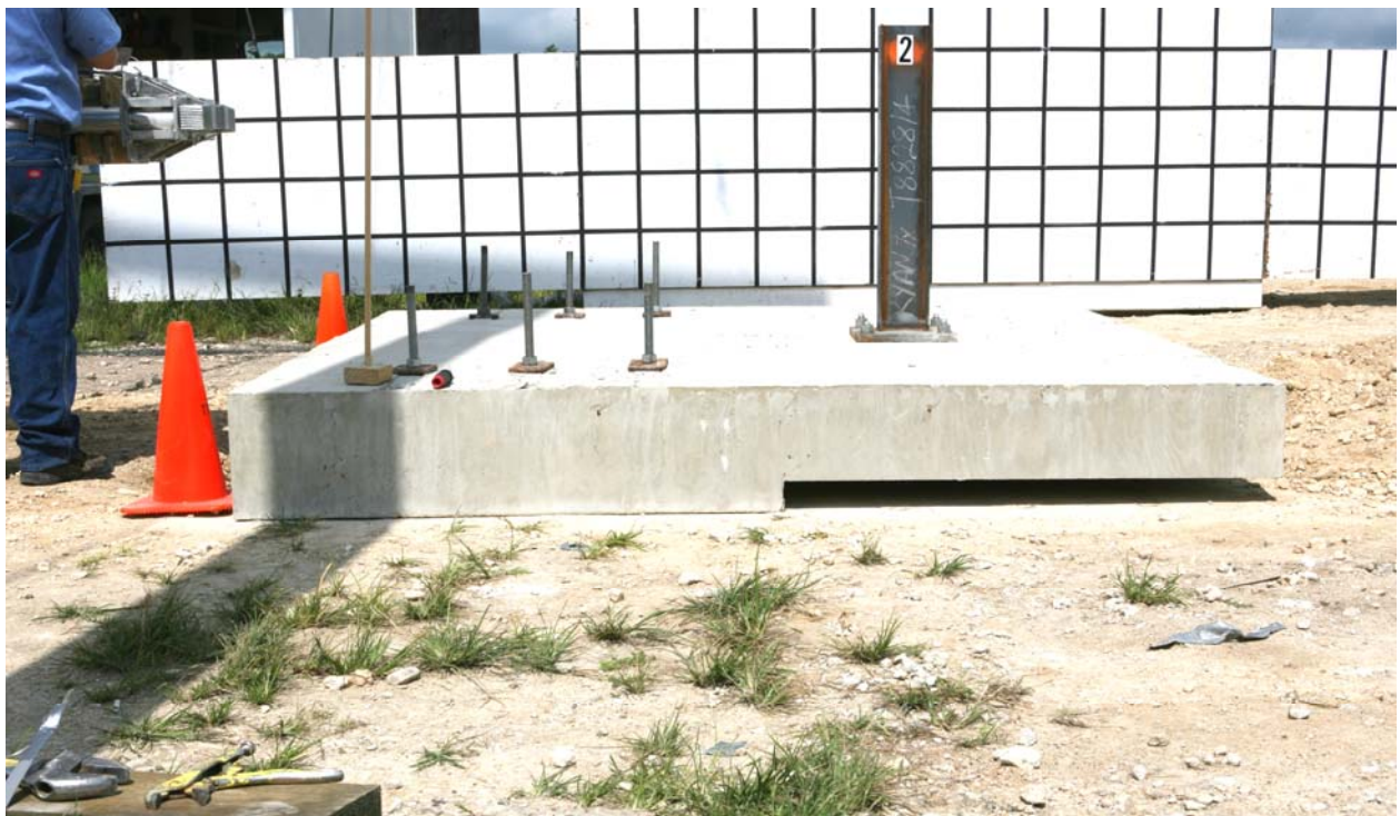
Figure D4. W6x9 post and deck sample before test P2.
