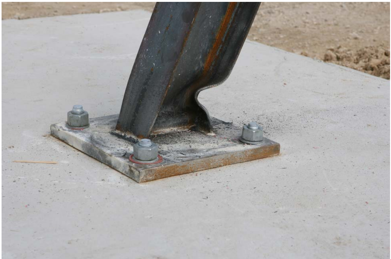
Figure E2. W6x9 post after test P1.
