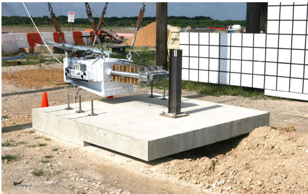
Figure E1. W6x9 post and deck sample before test P1.
