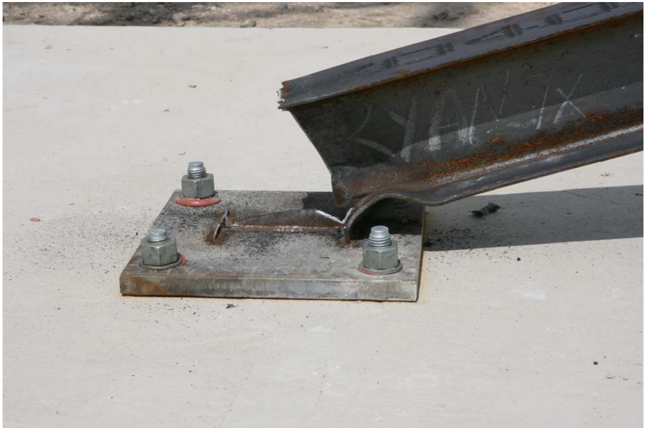
Figure E5. W6x9 post after test P2.
