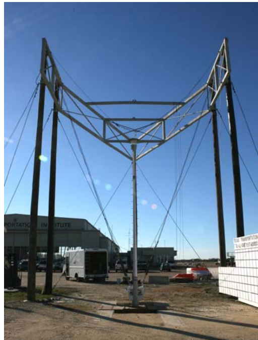
Figure B-1: Texas Transportation Institute Proving Ground's outdoor pendulum facility.
