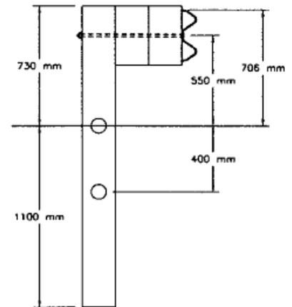
CRT wood posts, 1830 long w/ two 150x200x360 wood blockouts
