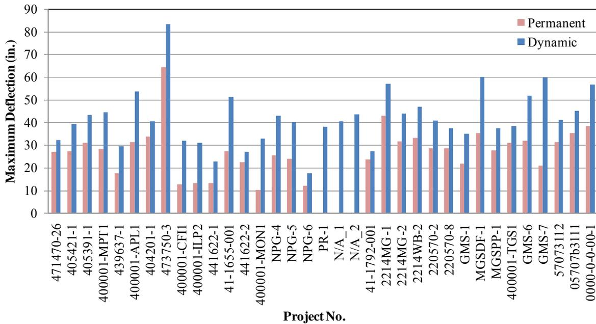
**Figure 3.4 Range of Maximum Deflection of 12 gauge W-Beam Guardrail Systems.**
