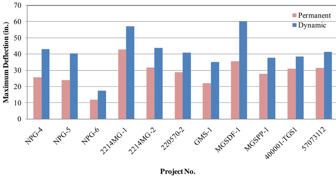
**Figure 3.6 Range of Maximum Deflection of 31-inch Tall W-beam Systems.**
