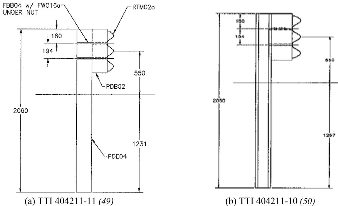
**Figure 3.7 Typical Thrie-beam Guardrail Cross Section.**
