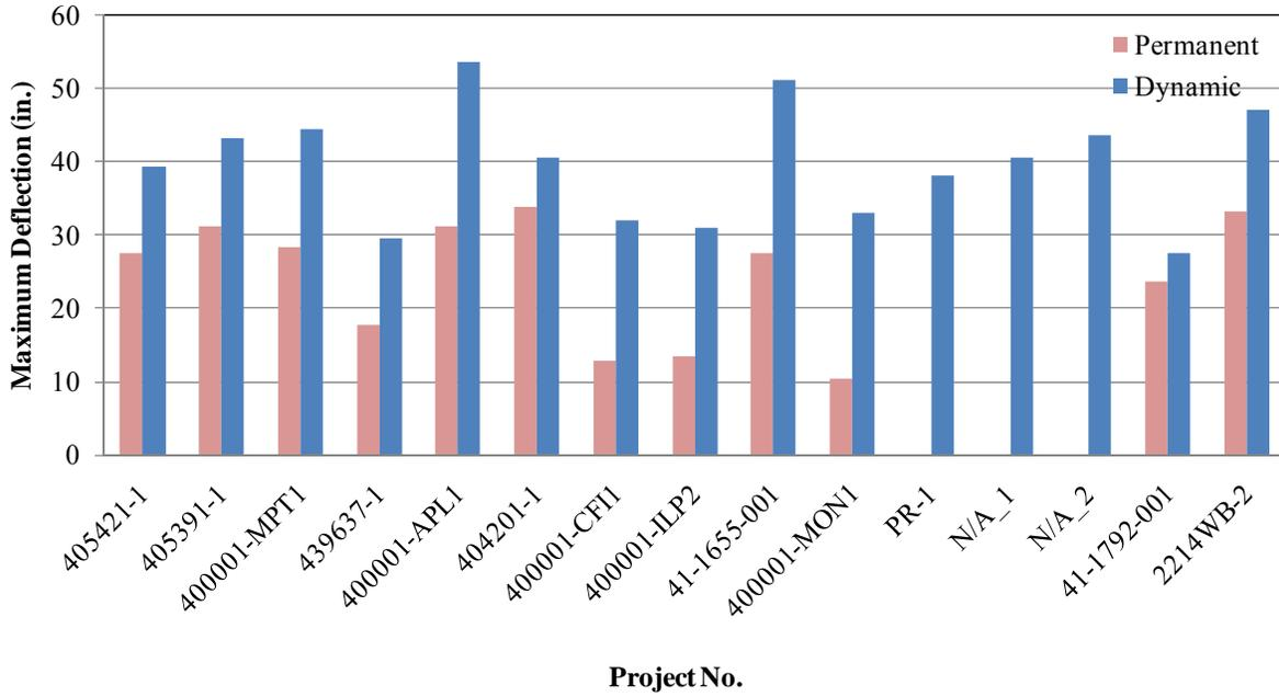
**Figure 3.5 Range of Maximum Deflection of 27.8-inch Tall W-beam Systems.**
