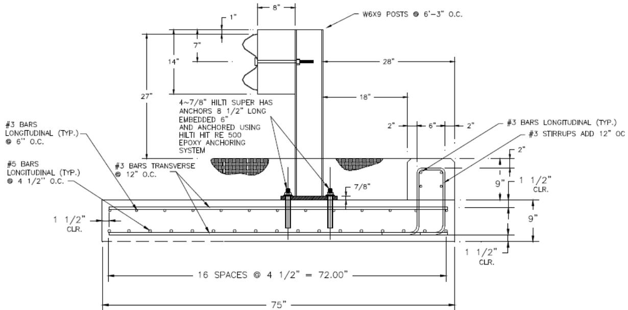
**Figure 3.13 W-beam guardrail on the simulated culvert application (MwRSF, KC-1)**
