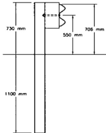
W6x9 steel posts, 1830 long w/ 150x200x360 routed wood blockouts
