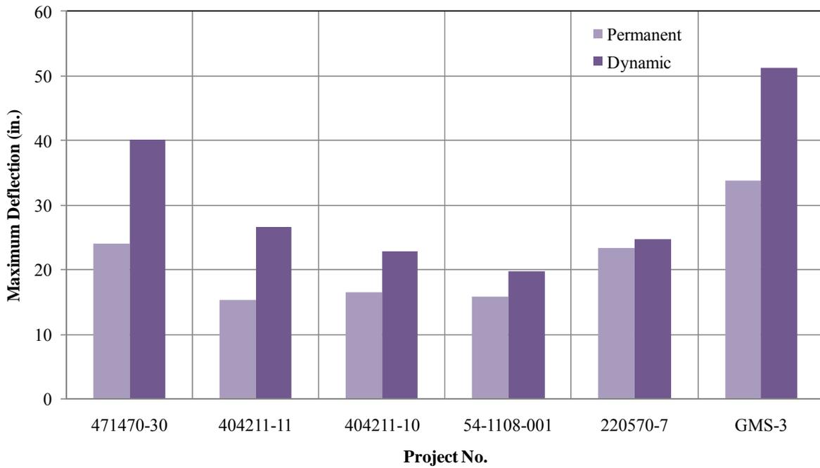
**Figure 3.9 Range of Maximum Deflection of Thrie-beam Guardrail Systems.**
