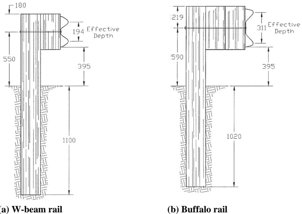
**Figure 3.10 Cross Section View of W-Beam and Buffalo Rail.**
