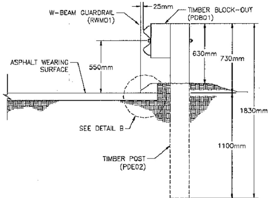
**Figure 3.2 12 gauge W-Beam Guardrail with Curb (TTI 404201-1, 2000) (24).**
