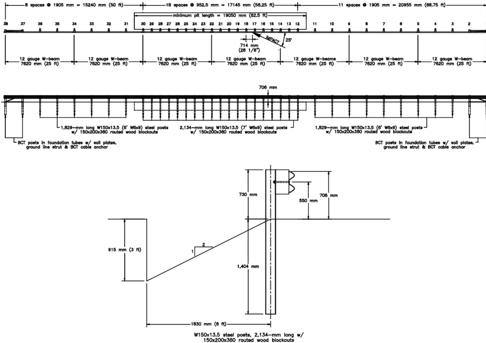
Figure 3.12 W-Beam Guardrail for Placement on a Slope (MwRSF, MOSW-1) (57).
