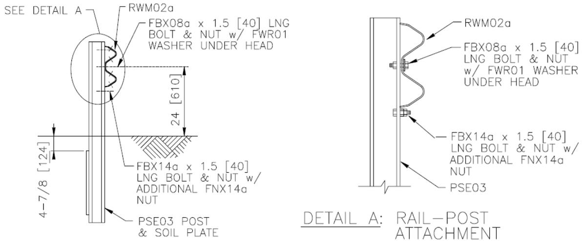
**(b) Weak Post, W-Beam Guardrail (G2) (16).**
