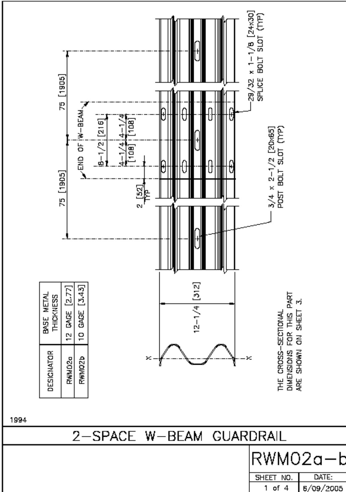
Figure A.1 AASHTO 2-space W-beam guardrail (RWM02a-b)
