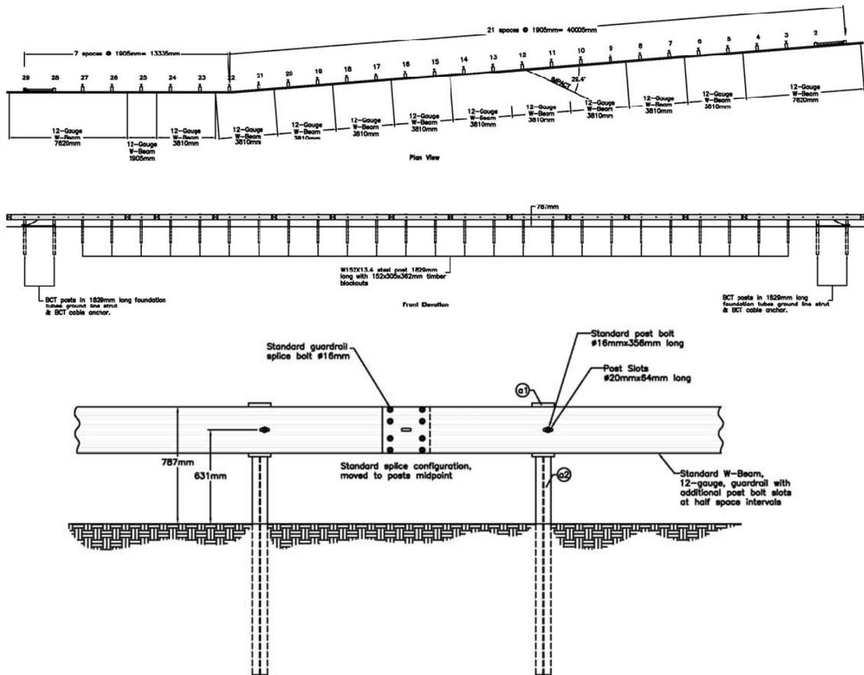
**Figure 3.14 W-beam guardrail on flare rate (MwRSF, FR-1) (63)**
