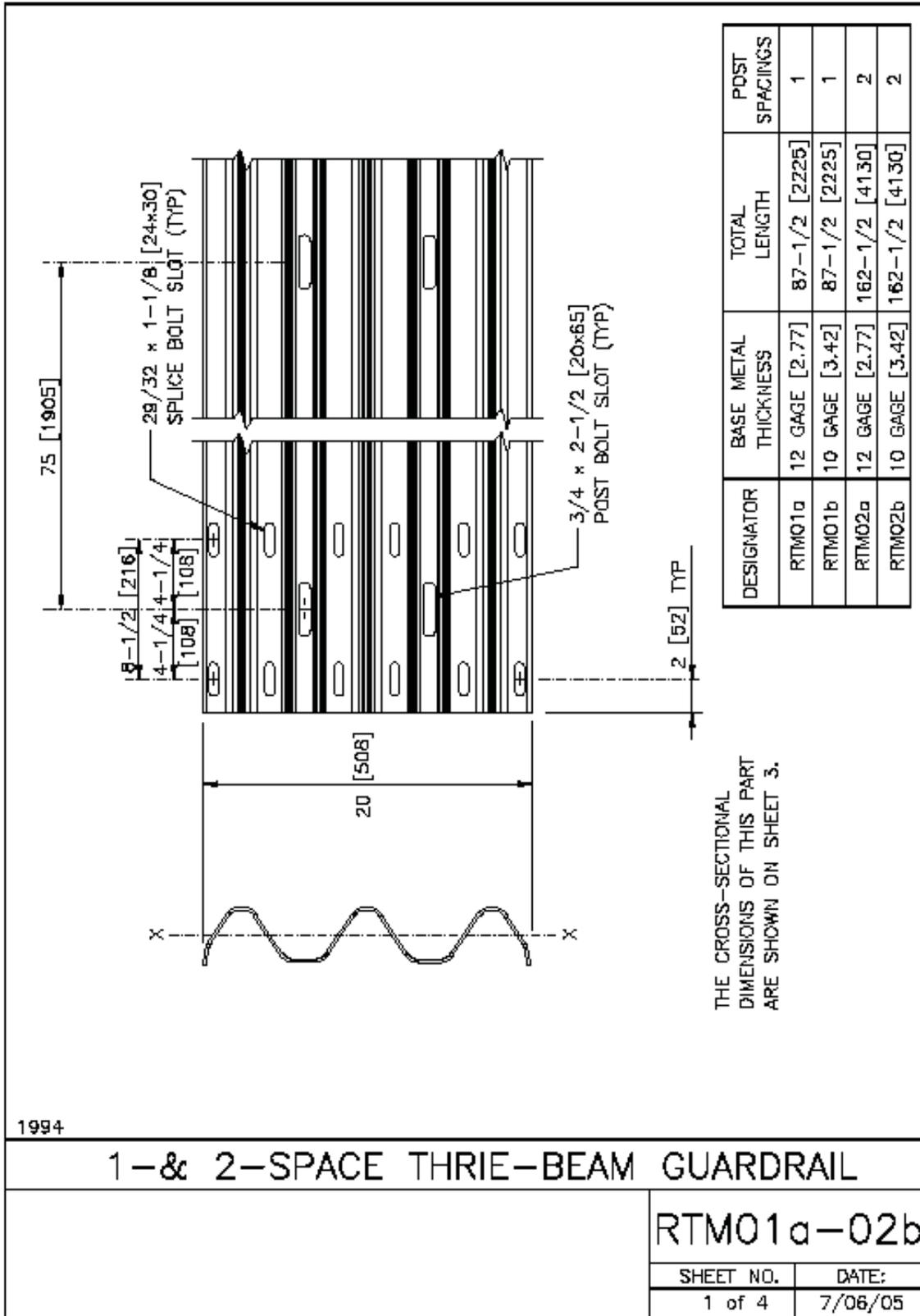
Figure A.2 AASHTO 1- & 2-space Thrie-beam guardrail (RTM01a-02b)
