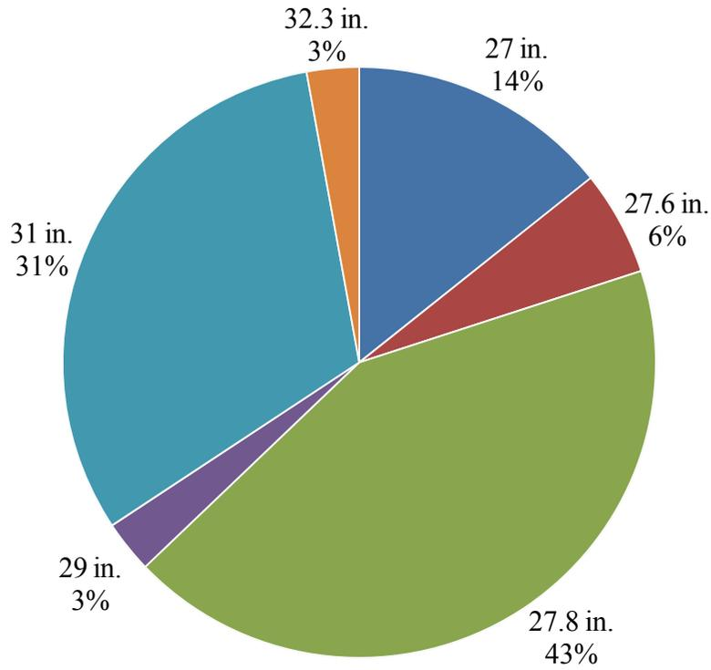
**Figure 3.3 Percentage of Rail Height for 12 gauge W-Beam Guardrail Systems.**
