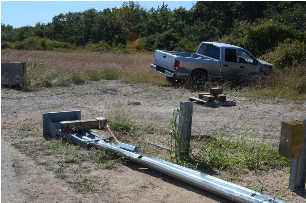
Figure 5.3. Vehicle trajectory path after test 405160-23-2.
