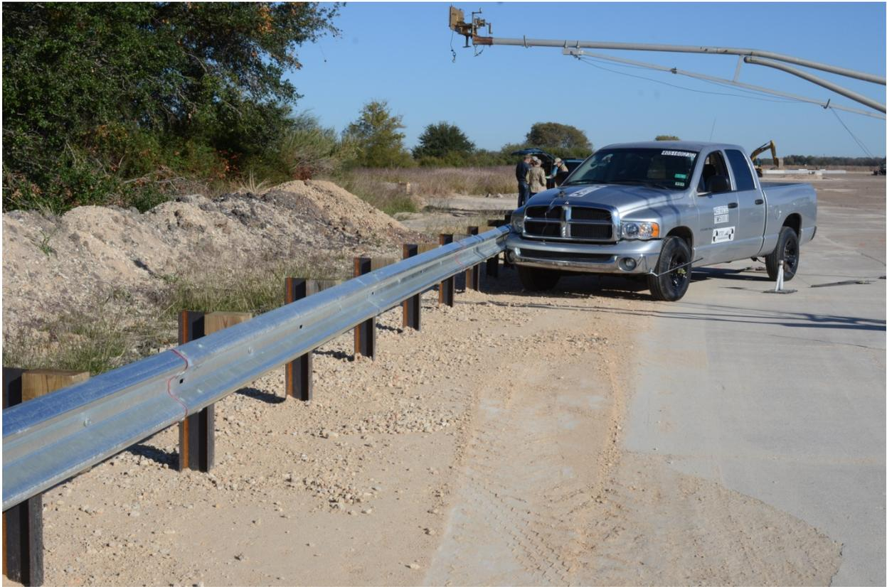
Figure 5.1. Vehicle/installation geometrics for test 405160-23-2.
