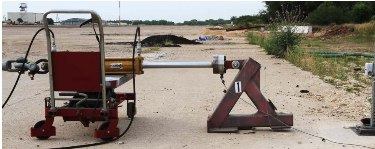
Figure 5: Test setup for quasi-static pull tests (pin installed in concrete is shown).
