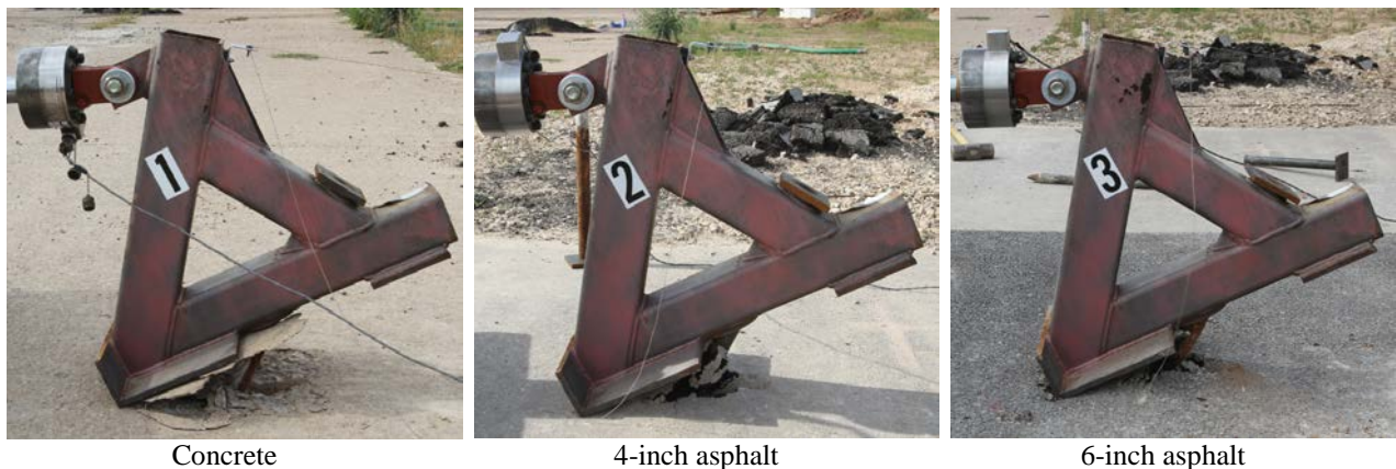
Figure 6: Concrete and asphalt damage after pull test
