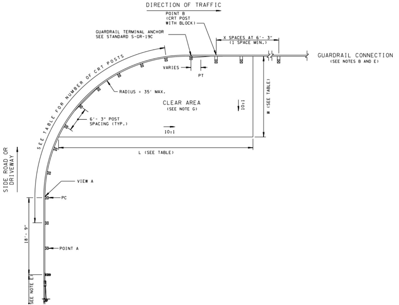
**Figure 3.5. Short Radius Guardrail (24).**
