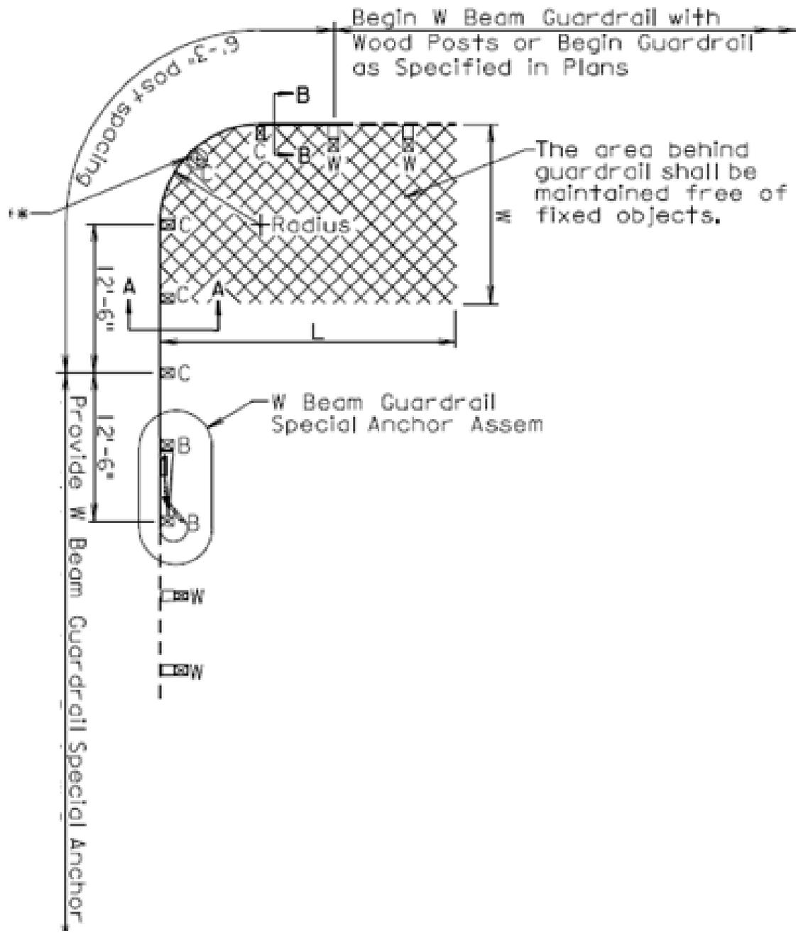
Figure 3.4. Nested Thrie Beam Transition and Short Radius Guardrail (21).
