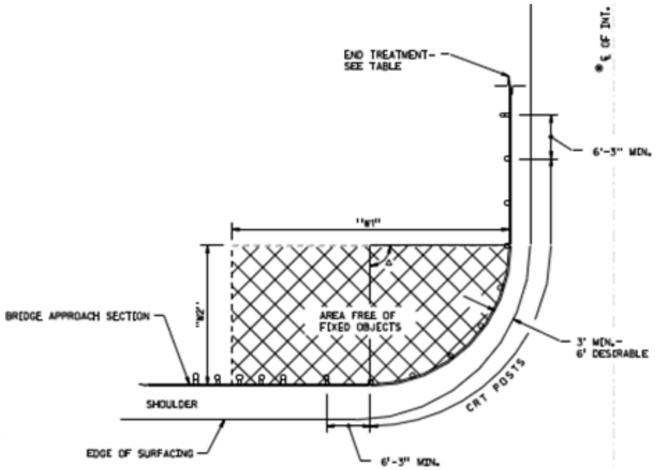
Figure 3.3. Curved Beam Guardrail (2).
