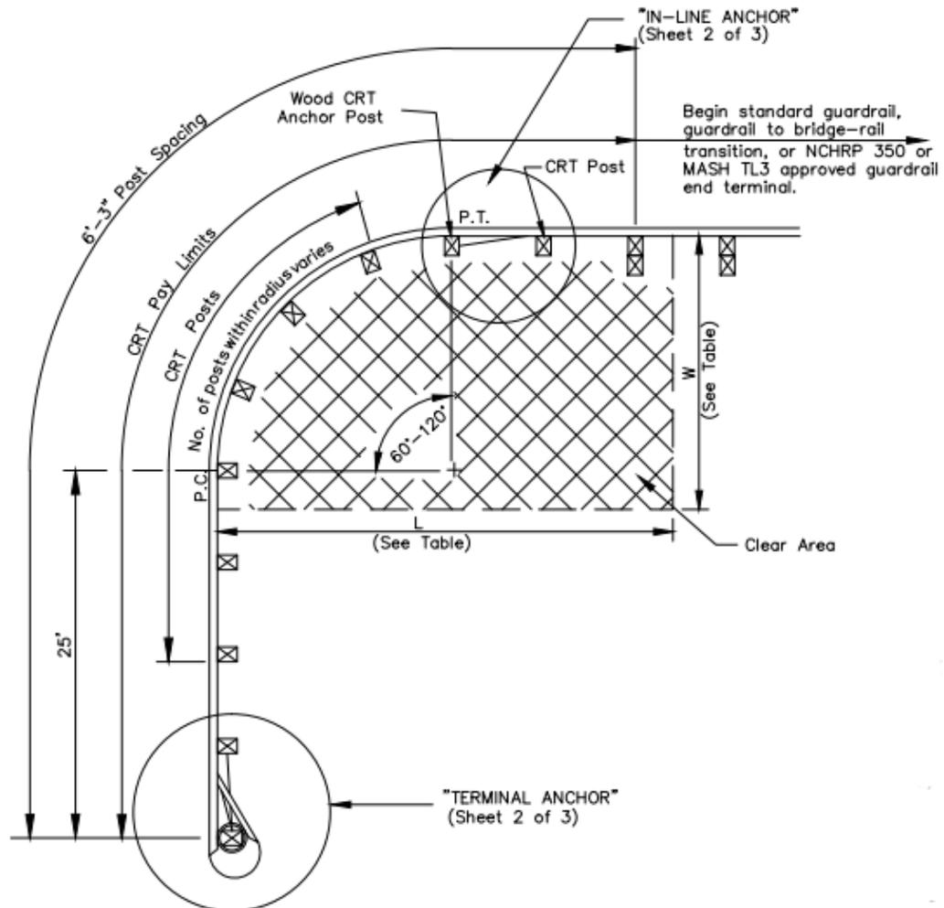
Figure 3.1. Wood Post Controlled Release Terminal (Alaska).
