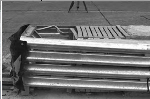
**TRACC System** – redirective, non-gating crash cushions available in a variety of lengths for a variety of highway speeds, requires low maintenance. Meets TL-2 & TL-3 test criteria.
