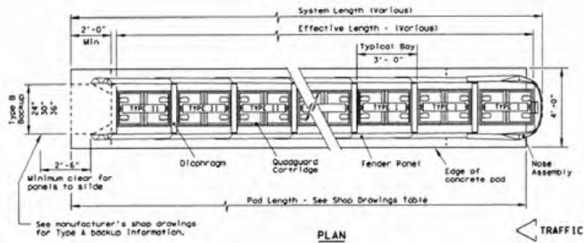
**Quadguard System** – redirective, non-gating crash cushion that consists of crushable, energy absorbing cartridges. Meets TL-3 criteria.
