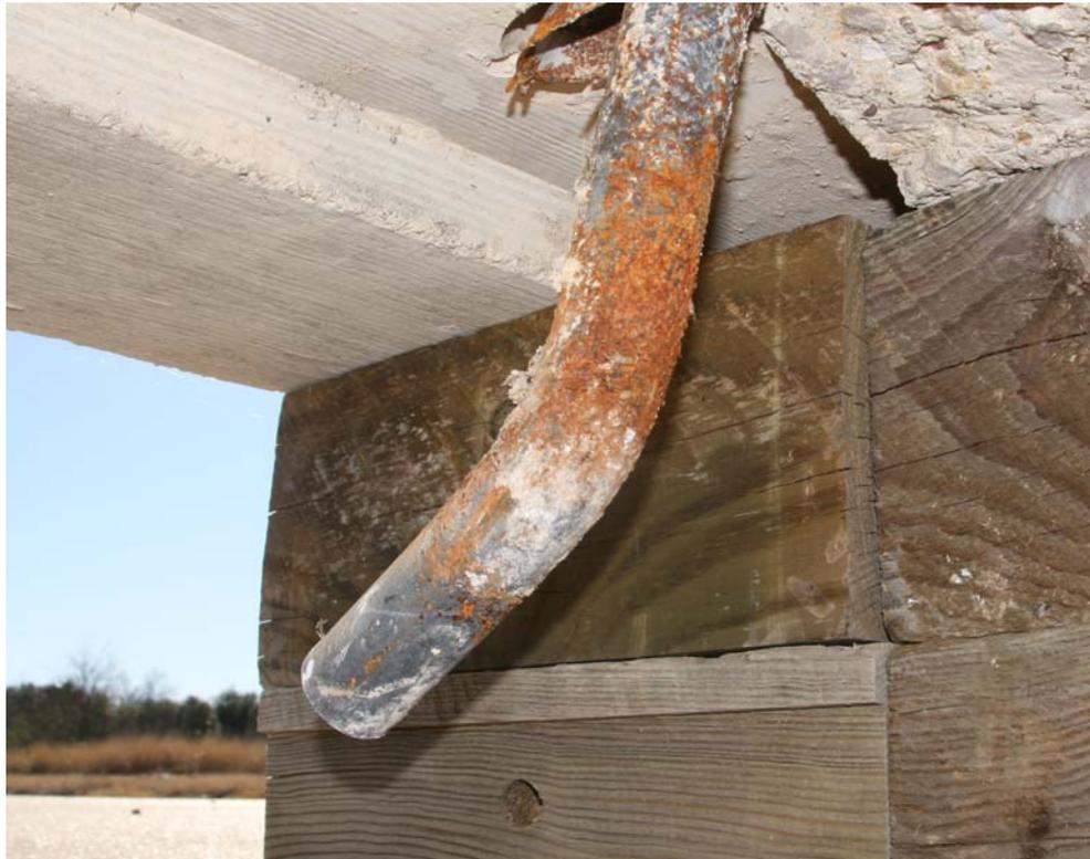
Figure 5.15. Deformed drop-pins after test 405160-3-1.
