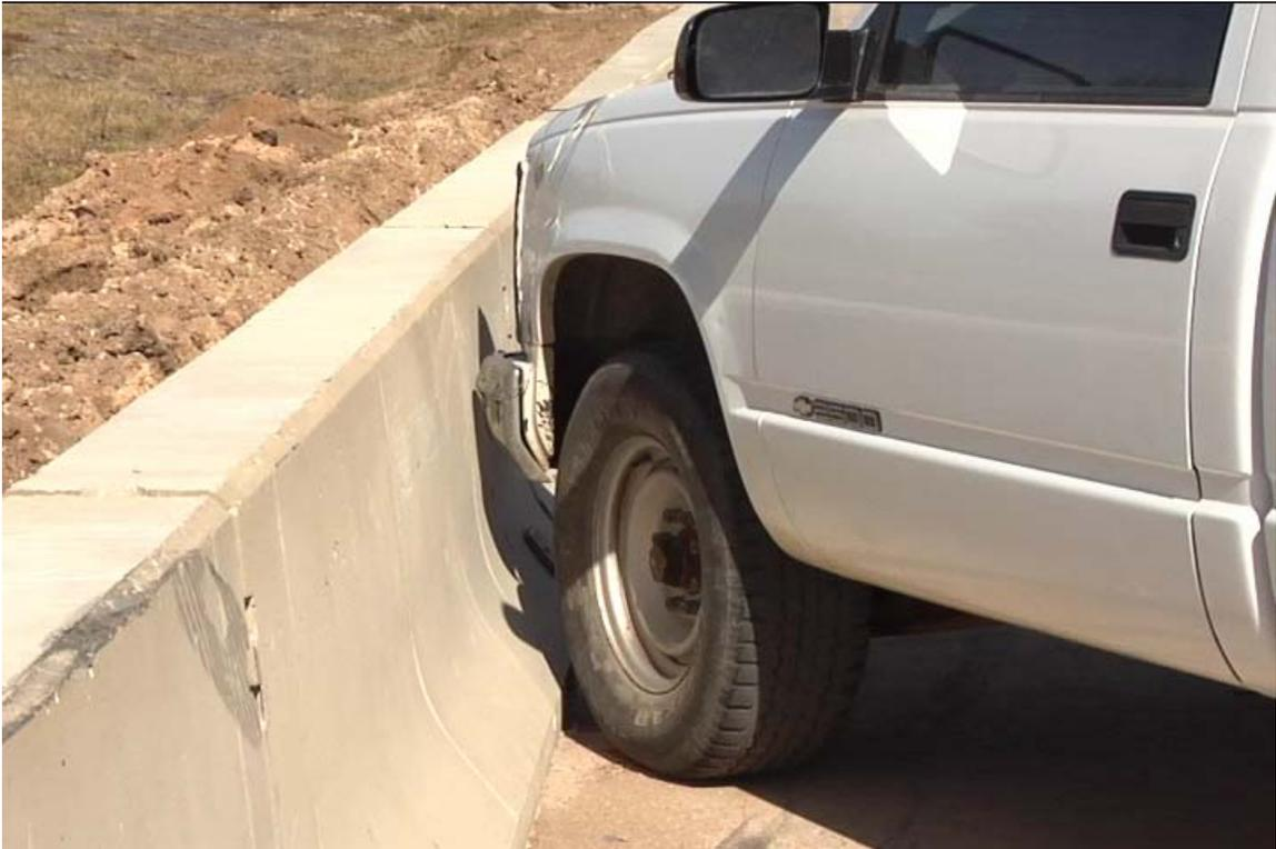
Figure 5.11. Vehicle/installation geometrics for test 405160-3-1.
