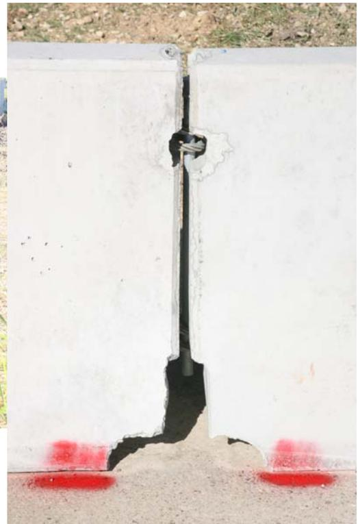
Figure 4.5. Pinned F-shape barrier prior to testing.
