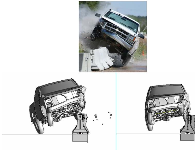
Figure 2.17. Vehicle climb comparison. Modified WSDOT simulation (left), old simulation (right), and crash test (top).
