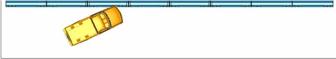
Figure 2.21. System model for the new pinned-down F-shaped barrier.
