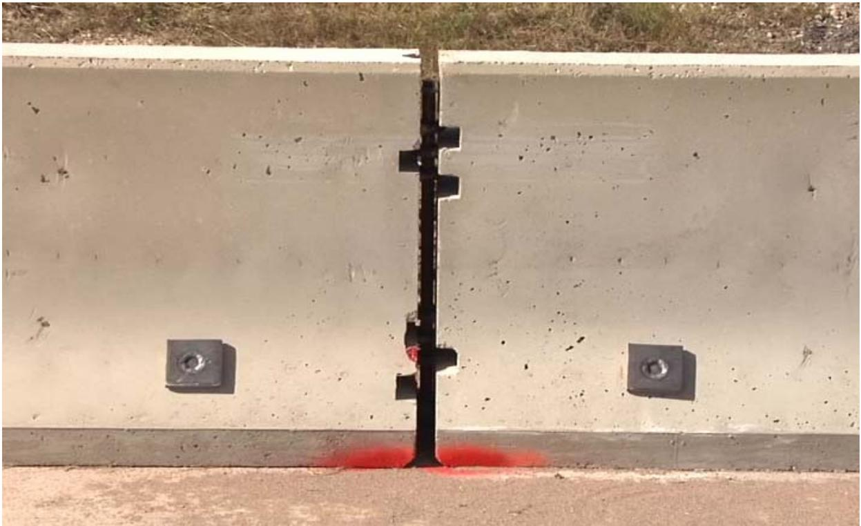
Figure 5.10. Pinned F-shape barrier prior to testing.
