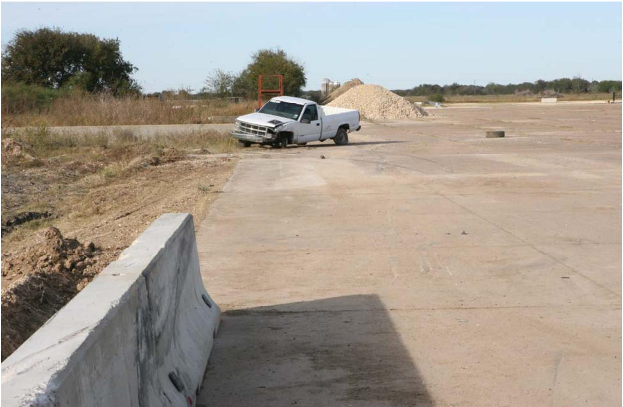
Figure 5.13. Vehicle trajectory path after test 405160-3-1.
