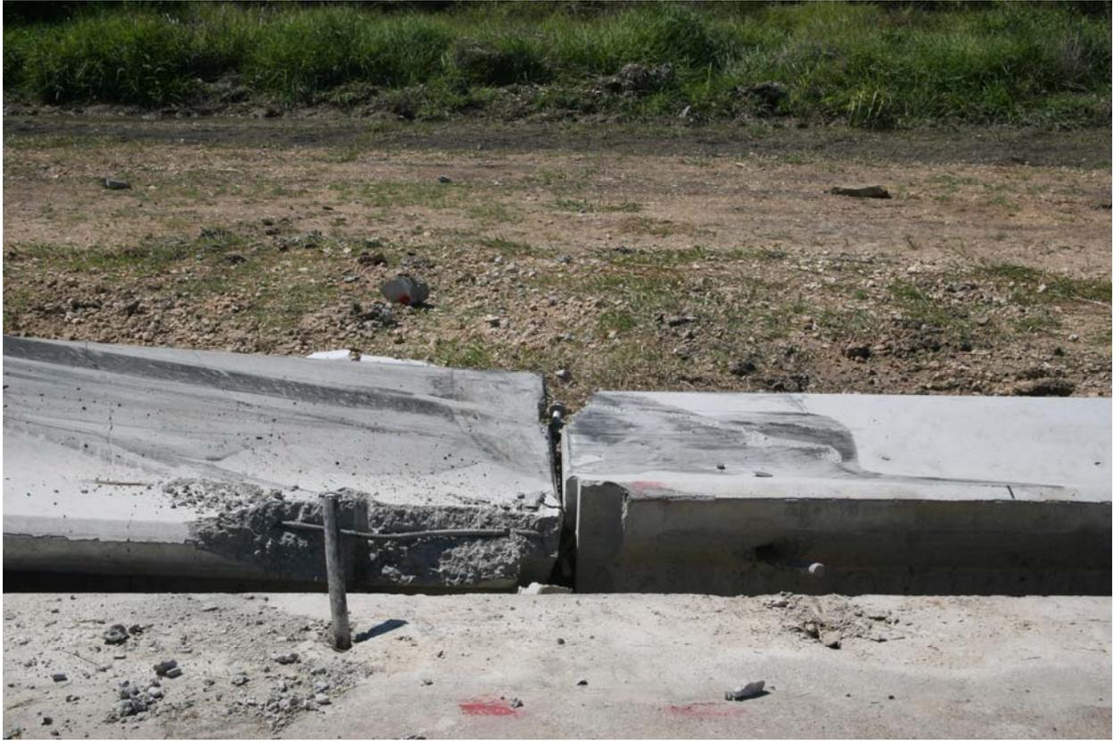
Figure 4.10. Concrete failure around the upstream drop-pin of the forth barrier segment after test 405160-3-1.
