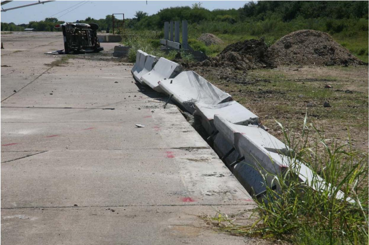
Figure 4.8. Vehicle trajectory path after test 405160-3-1.
