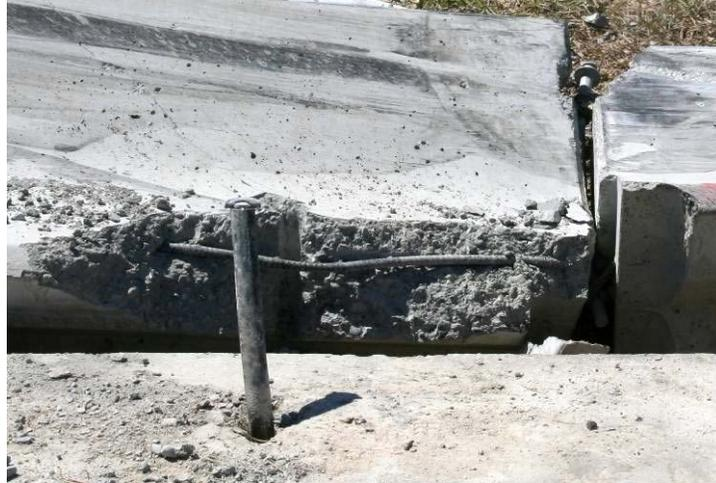
Figure 2.10. Failure of the concrete around the drop-pin at the joint of impact.
