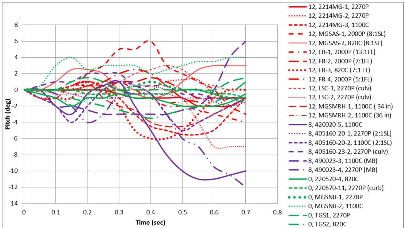
**Figure 4.20.** Recorded pitch angles from all considered tests.
