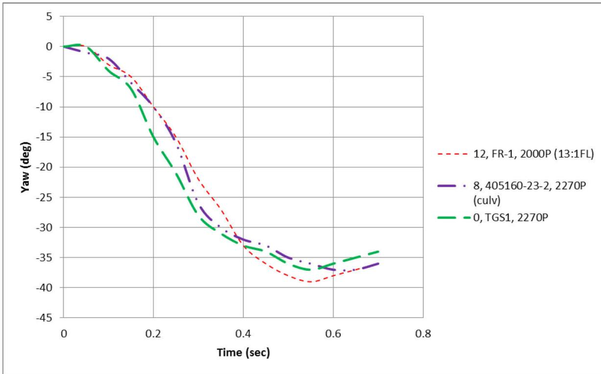
**Figure 4.2.** Yaw angular displacement comparison for selected tests with use of 12-inch, 8-inch, and no blockouts.
