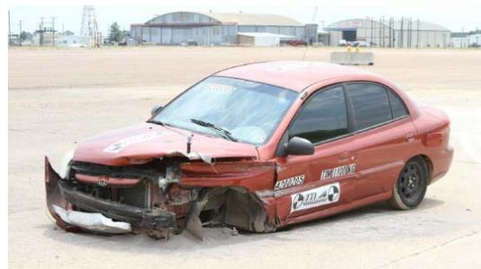
(b) Vehicle damage after test No. 420020-5
