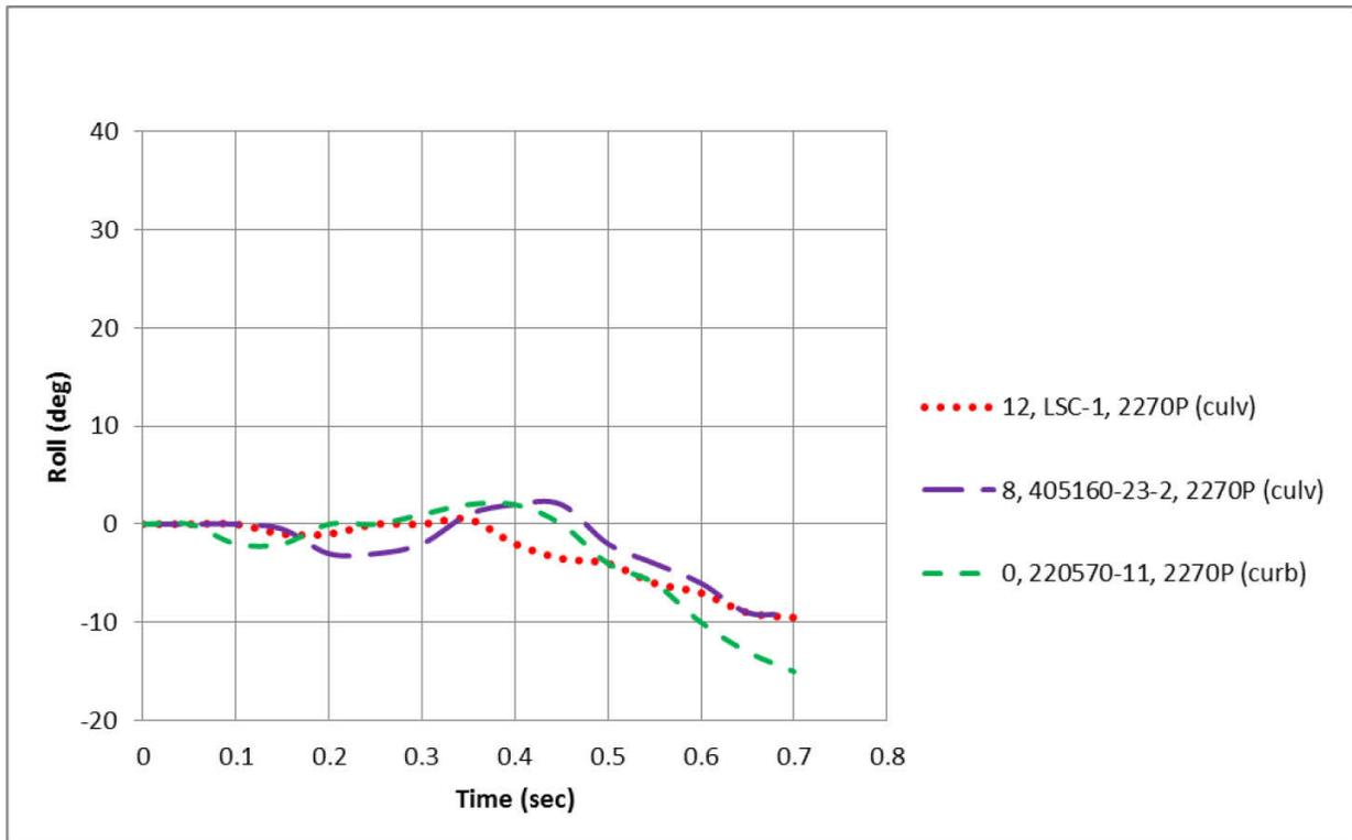
**Figure 4.12.** Roll angular displacement comparison for selected tests with use of 12-inch, 8-inch, and no blockouts.
