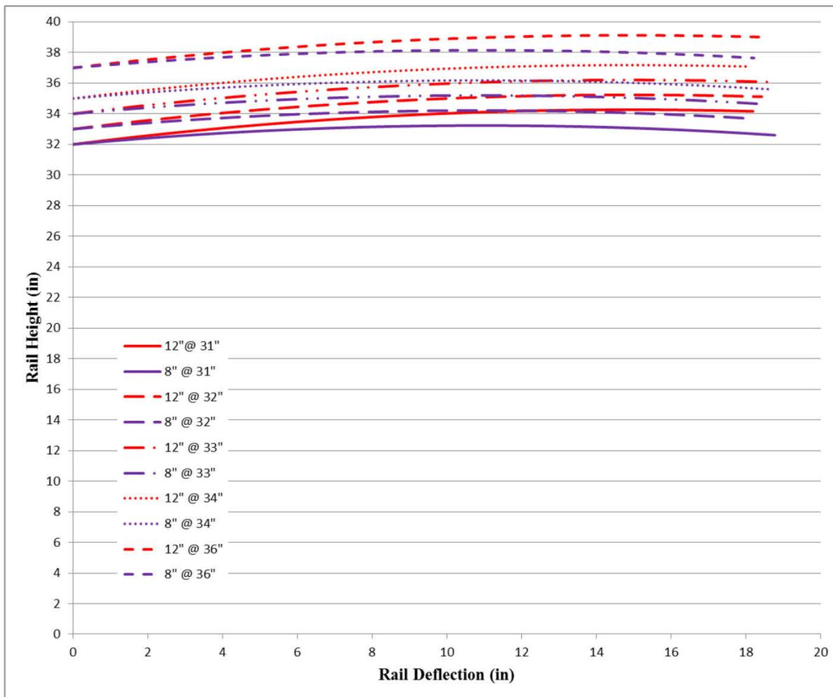
**Figure 7.1.** Analytical rail height variation with respect to horizontal rail deflection during post rotation.
