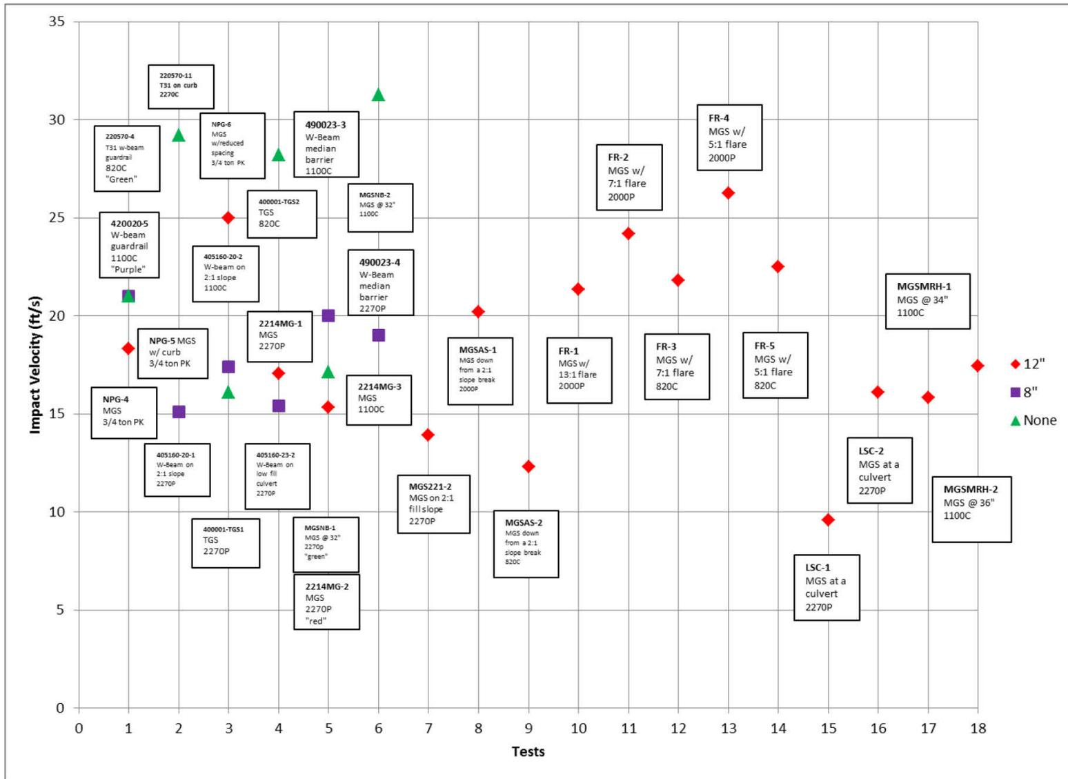
Figure 5.1. Longitudinal impact velocity with test specifications.
