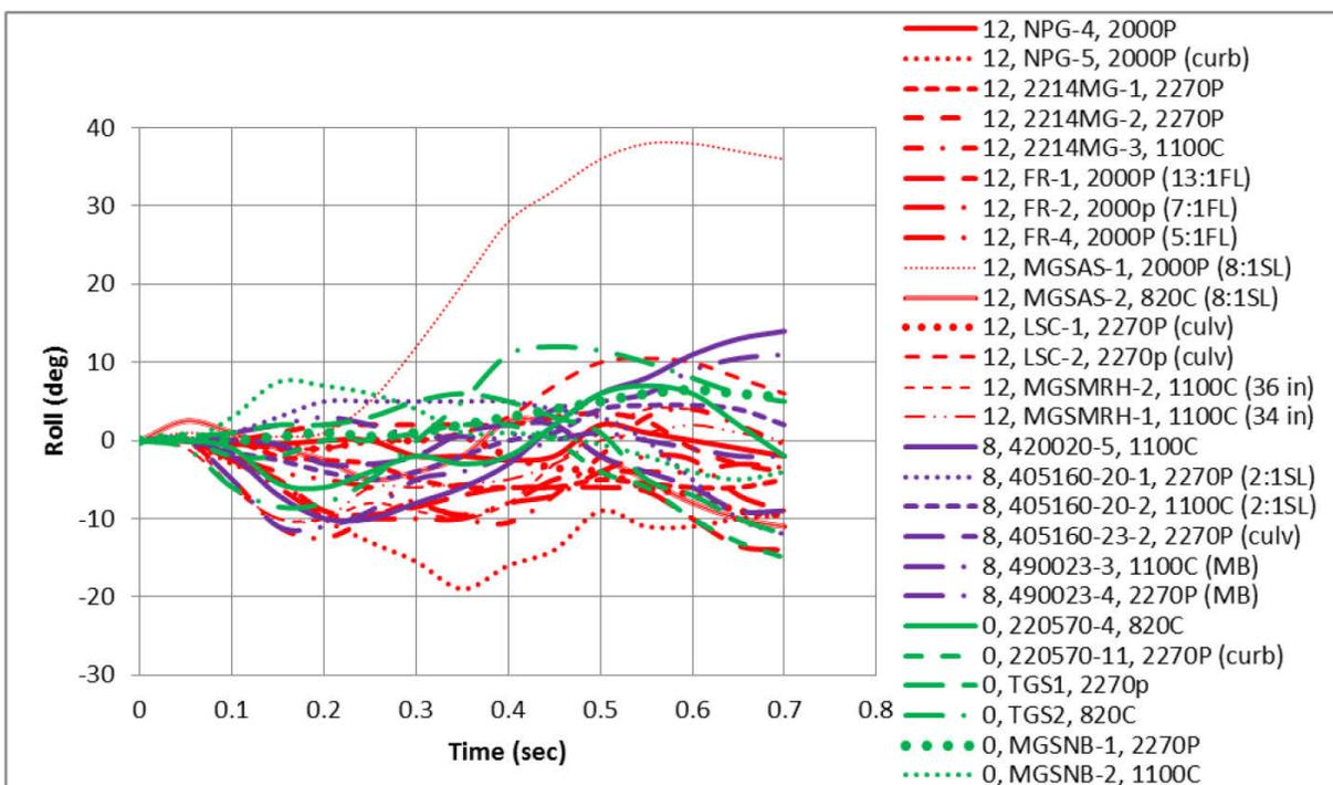
**Figure 4.11.** Recorded roll angles from all considered tests.
