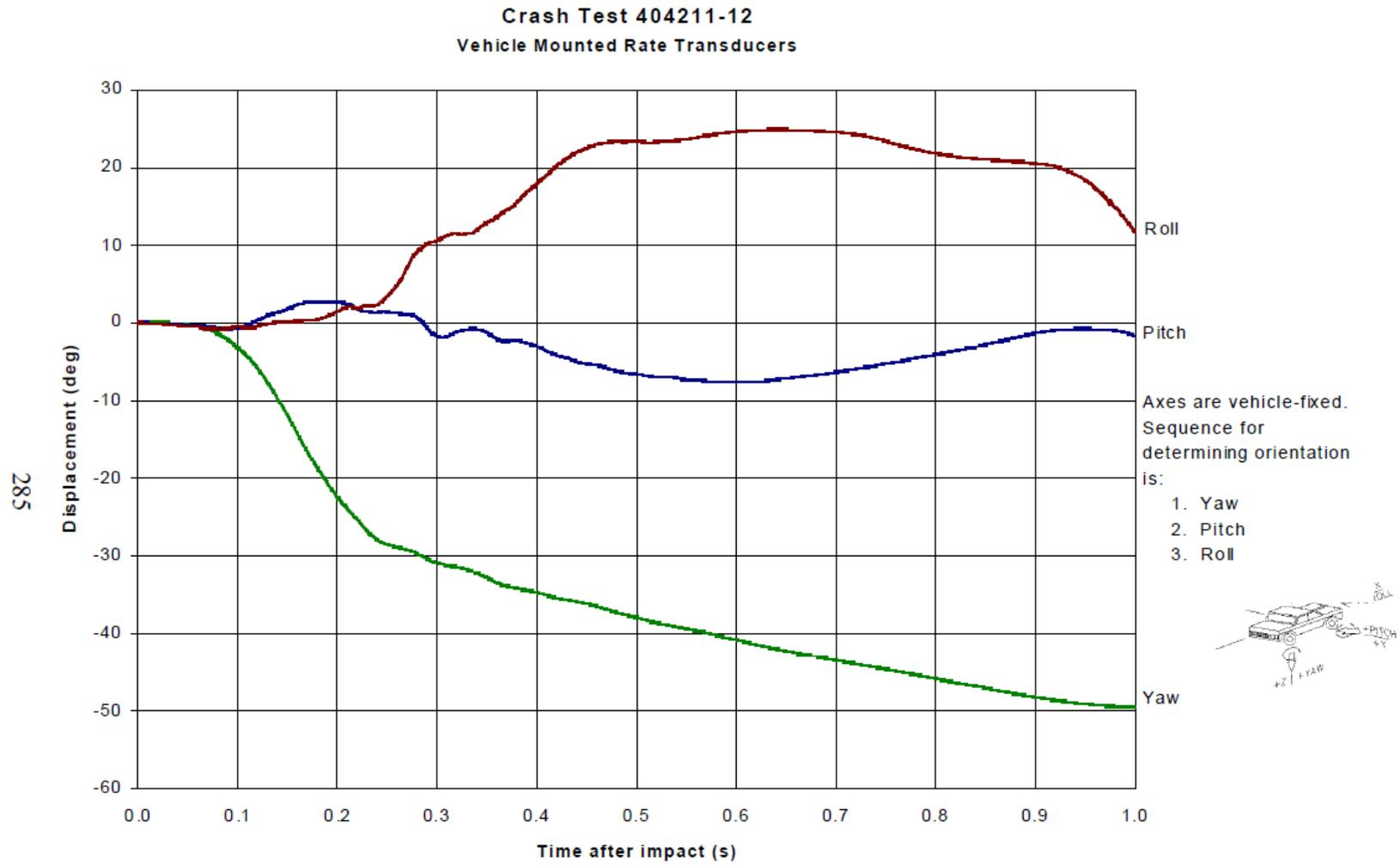
**Figure 2.6. Angular Displacements for Test 404211-12.**
