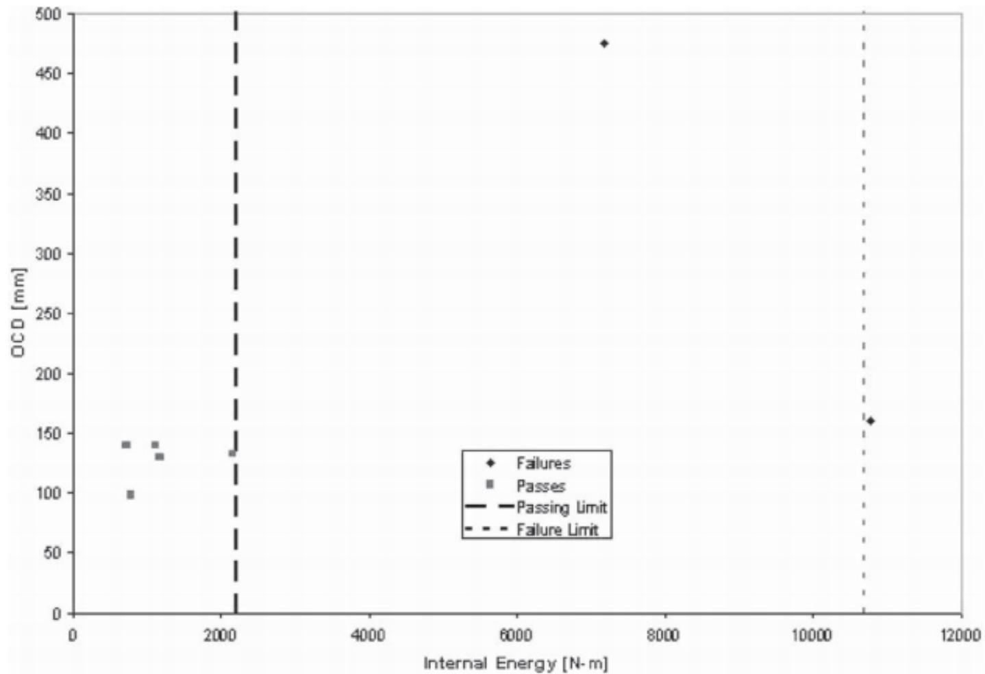
Figure 3.6. Passing and Failing Crash Tests OCD Versus Internal Energies of Floorboard (ref.).
