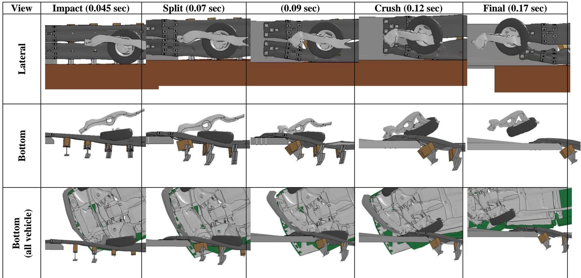
Figure 3.9. Vehicle Snagging Behavior Against Parapet from FE Simulation of 31-in High Stacked W-Beam Transition (without Bolts).
