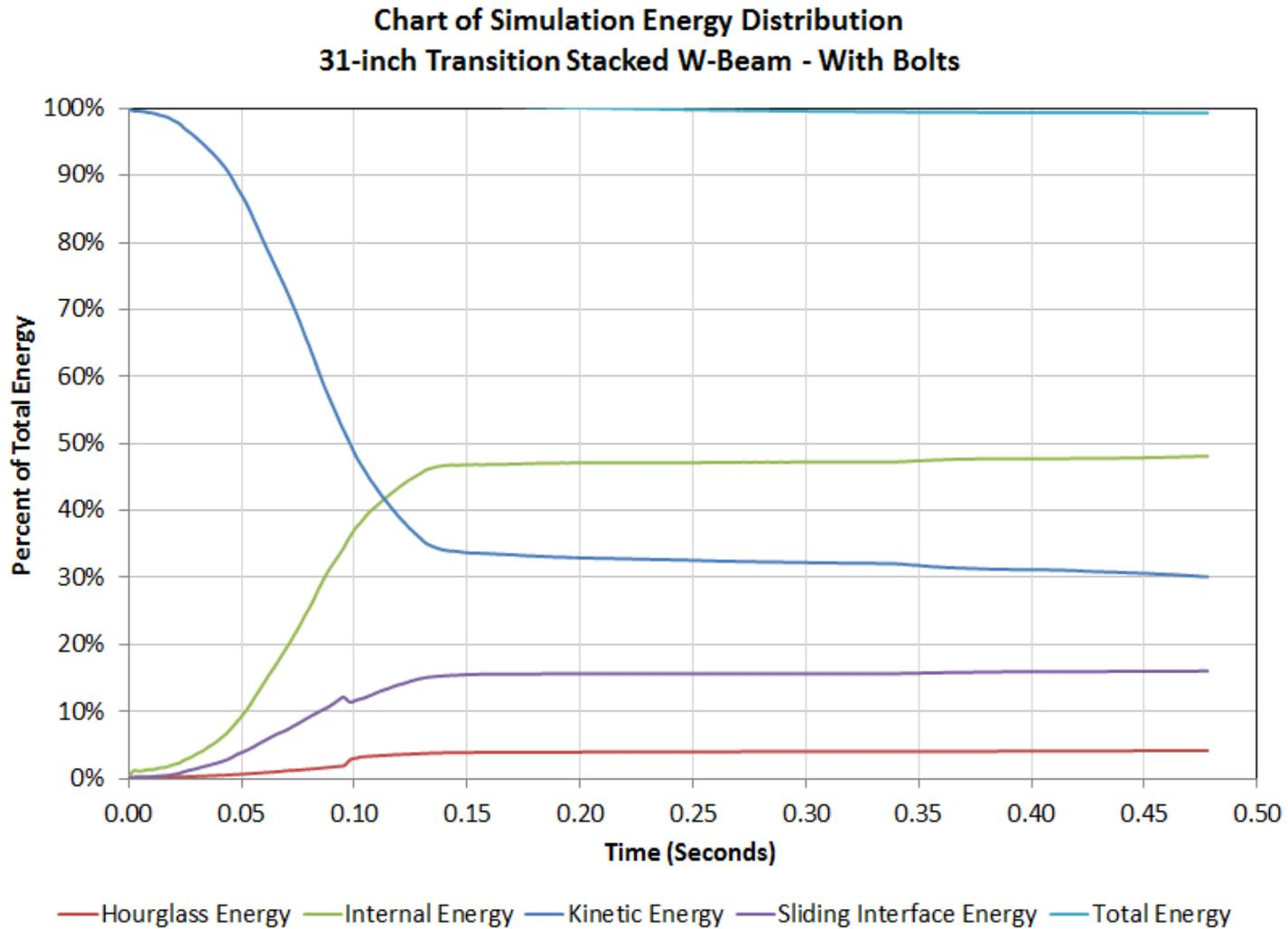
**Figure 3.12. Energy Distribution Time History (31-in Height Stacked W-Beam Transition with Bolts).**
