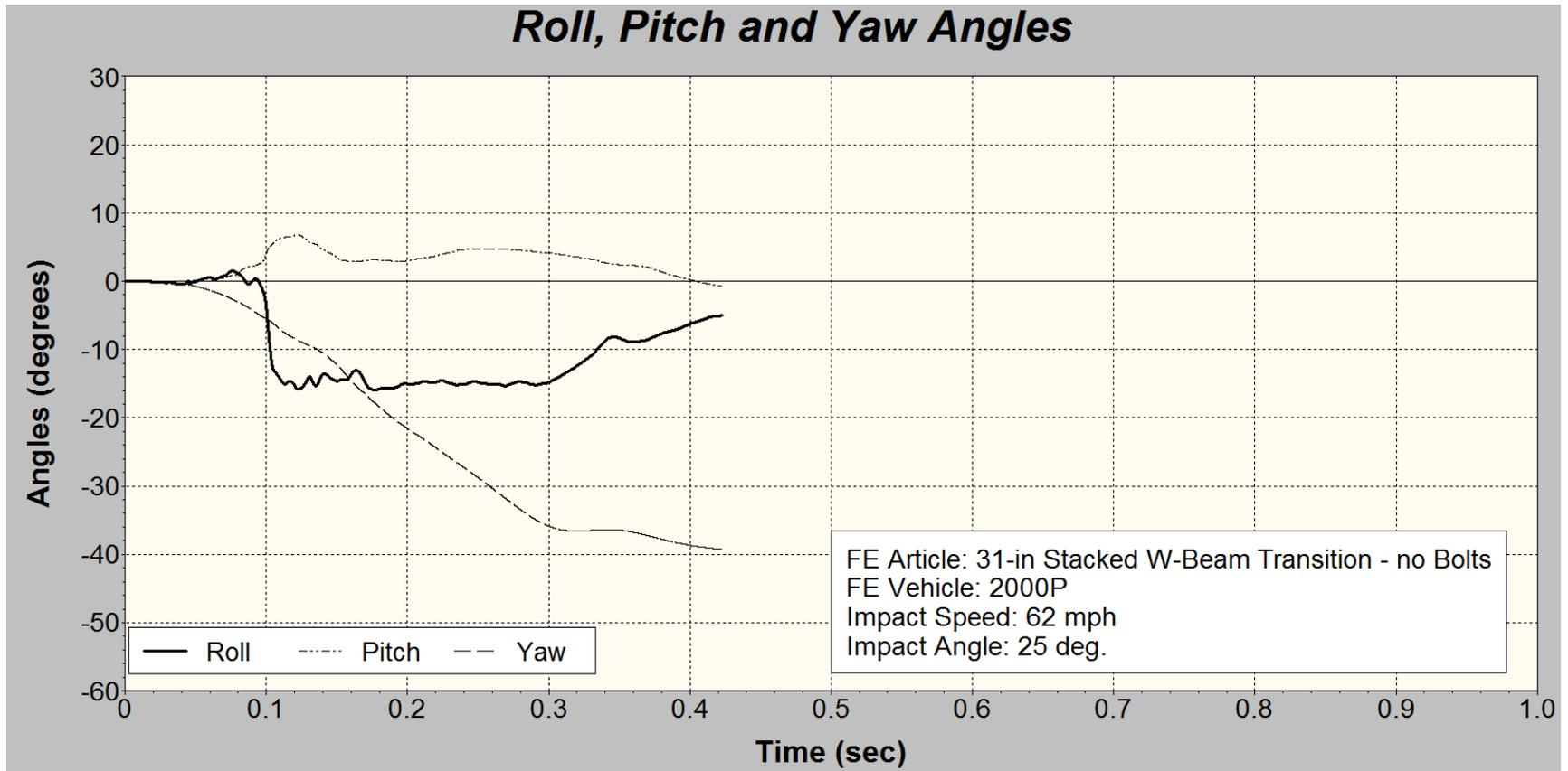
**Figure 3.5. Angular Displacements for FE Simulation Validation of the 31-in High Stacked W-Beam Transition, no Bolts.**
