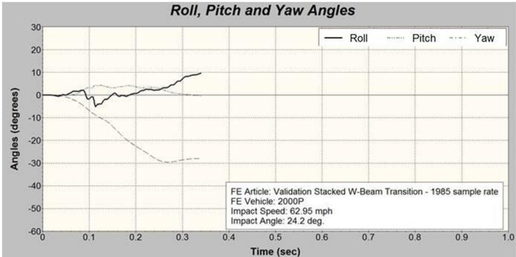
**Figure 2.7. Angular Displacements for FE Simulation Validation of the 27-in High Stacked W-Beam Transition.**
