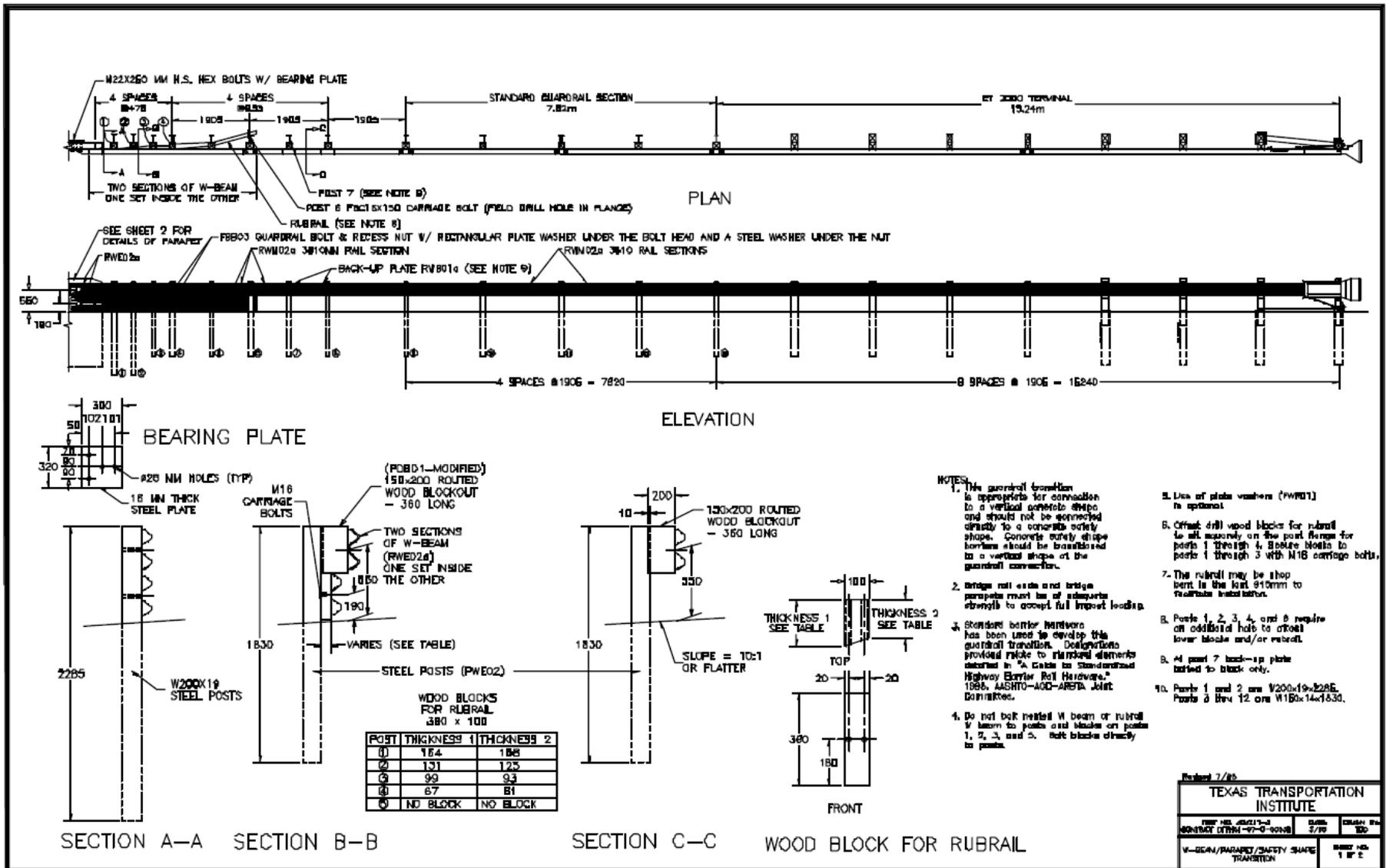
Figure 2.1. Details of the Vertical Wall Transition Installation for Test 404211-12.
