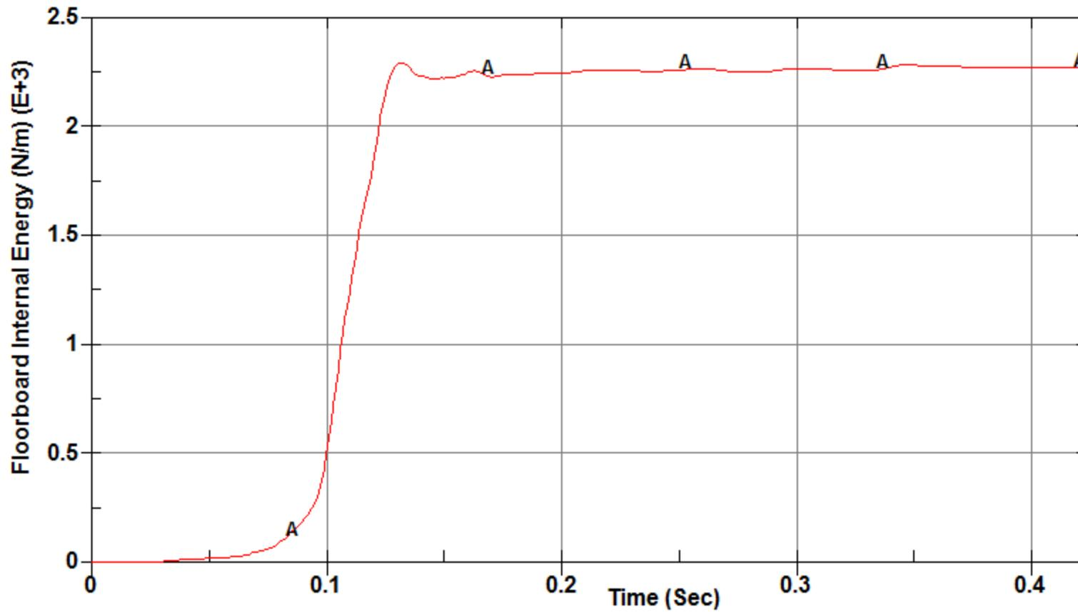
Figure 3.7. Floorboard Internal Energy for NCHRP 350 Test 3-21 with 31-in Stacked W-Beam Transition (without Bolts).
