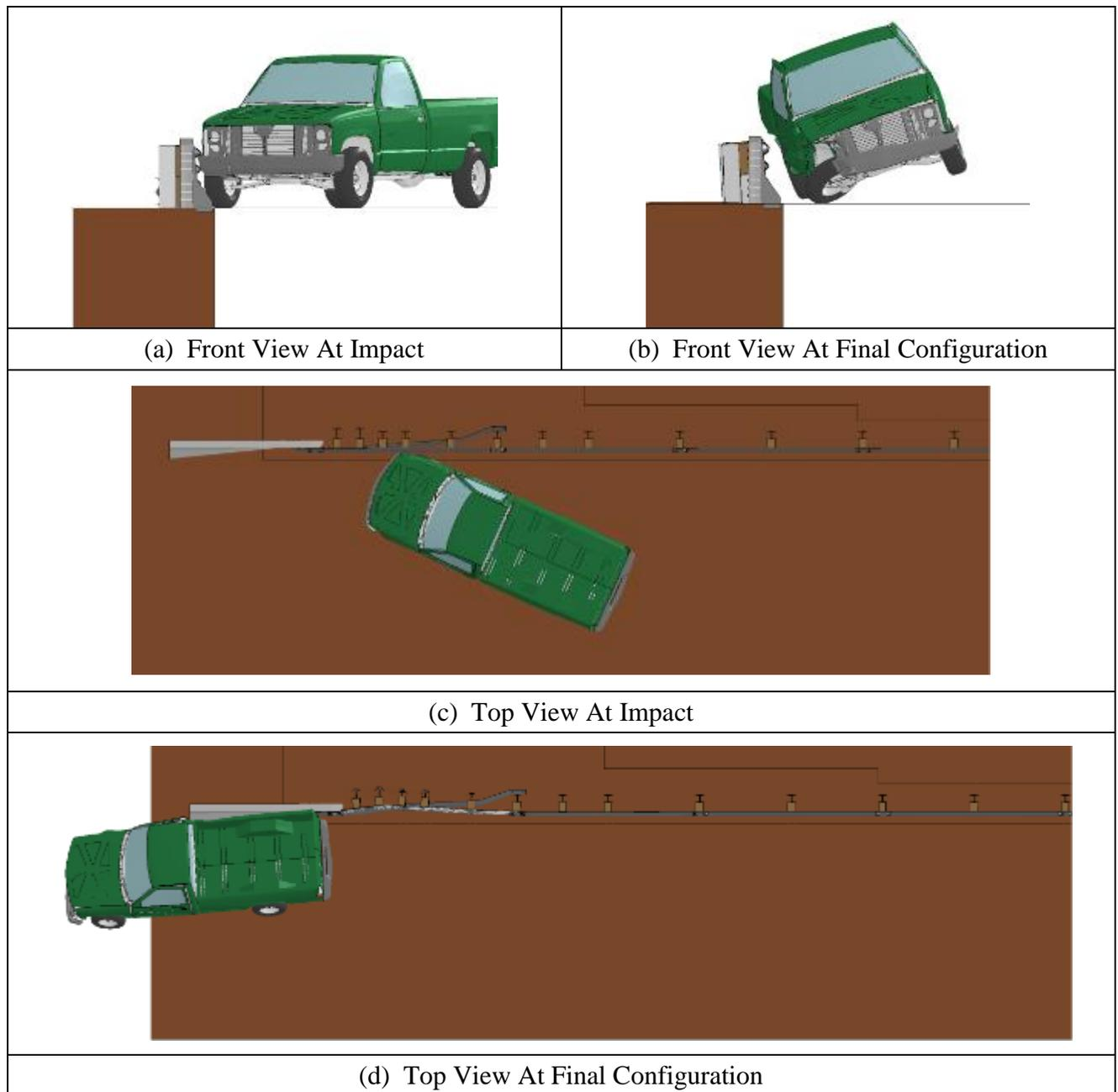
**Figure 2.3. Initial and Deflected Shape of Barrier (27-in Height Stacked W-Beam Transition).**
