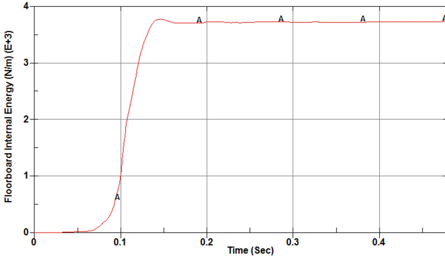
Figure 3.15. Floorboard Internal Energy for NCHRP 350 Test 3-21 with 31-in Stacked W-Beam Transition (with Bolts).
