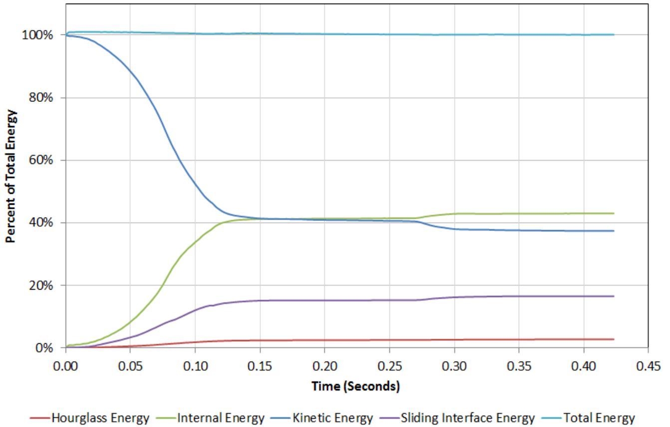
**Figure 3.3. Energy Distribution Time History (31-in Height Stacked W-Beam Transition without Bolts).**
