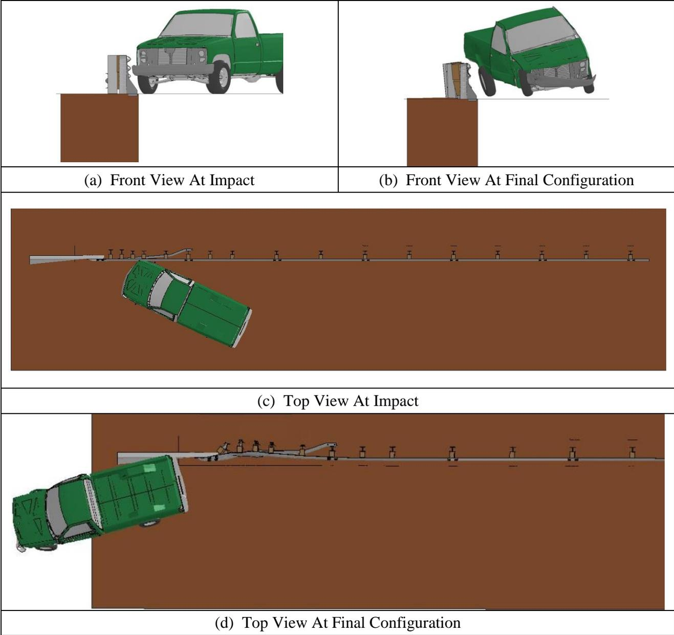
**Figure 3.2. Initial and Deflected Shape of Barrier (31” Height Stacked W-Beam Transition, without Bolts).**
