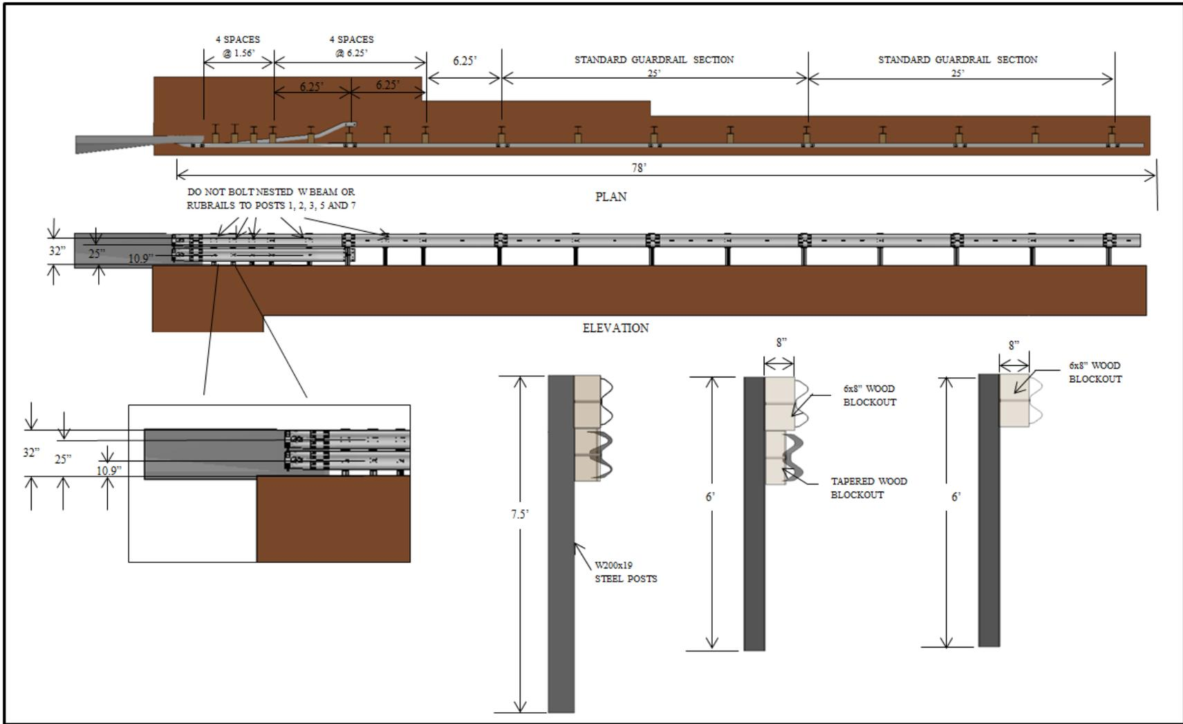
**Figure 3.1. Details of the Vertical Wall Transition Installation for Finite Element Computer Model Simulations (31-in, no bolts).**
