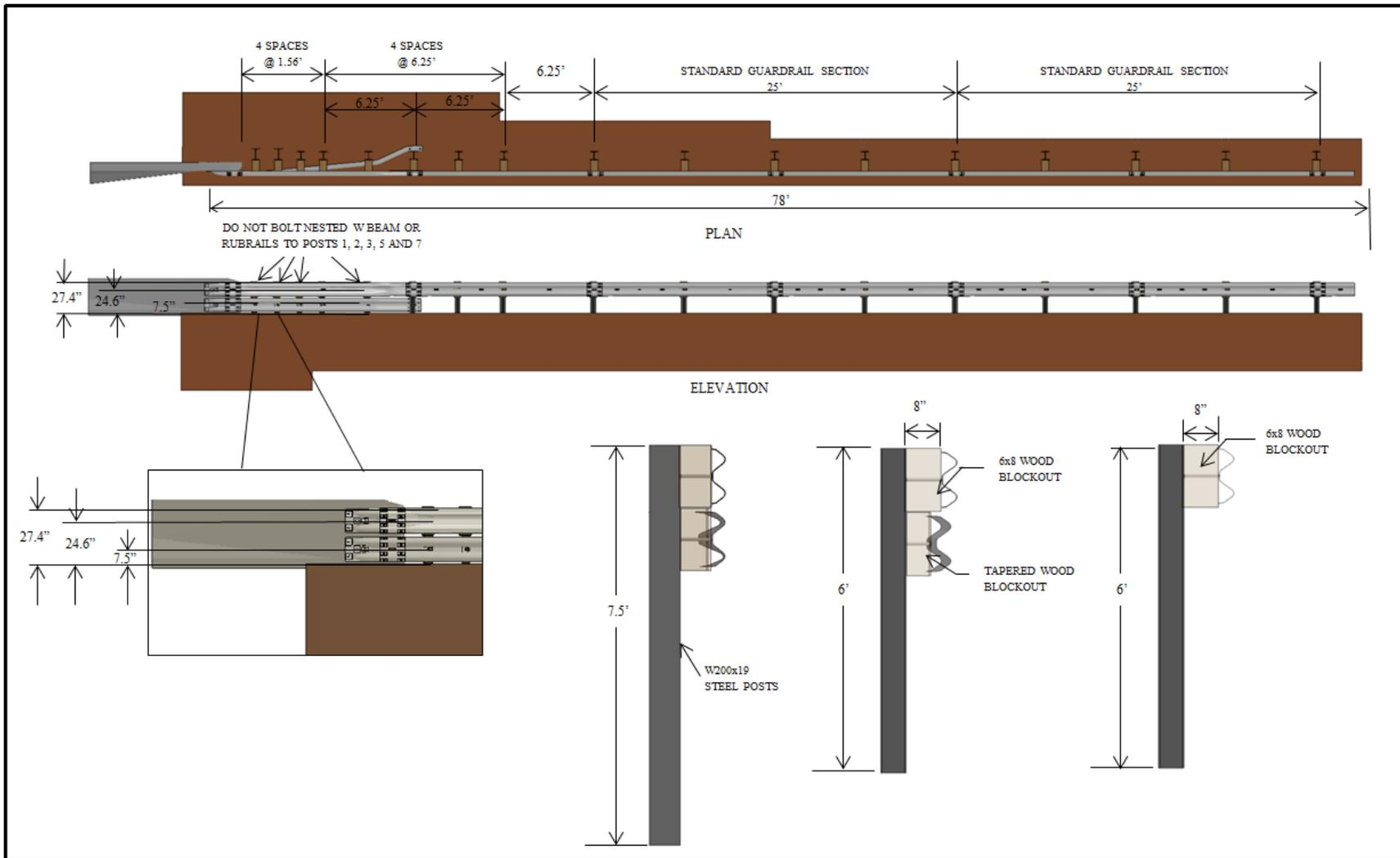
**Figure 2.2. Details of the Vertical Wall Transition Installation for Finite Element Computer Model Simulations.**
