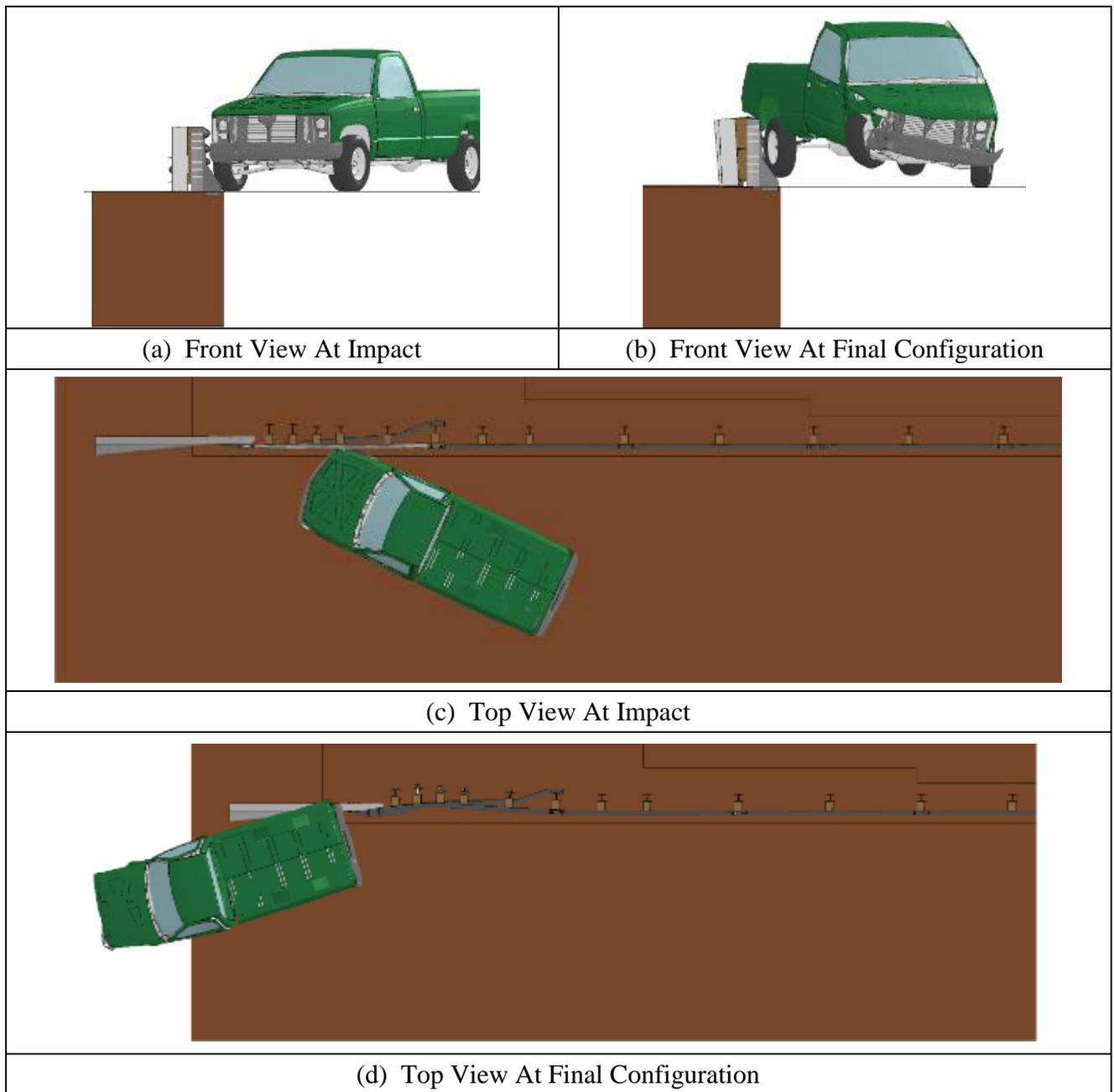
**Figure 3.11. Initial and Deflected Shape of Barrier (31-in Height Stacked W-Beam Transition with Bolts).**
