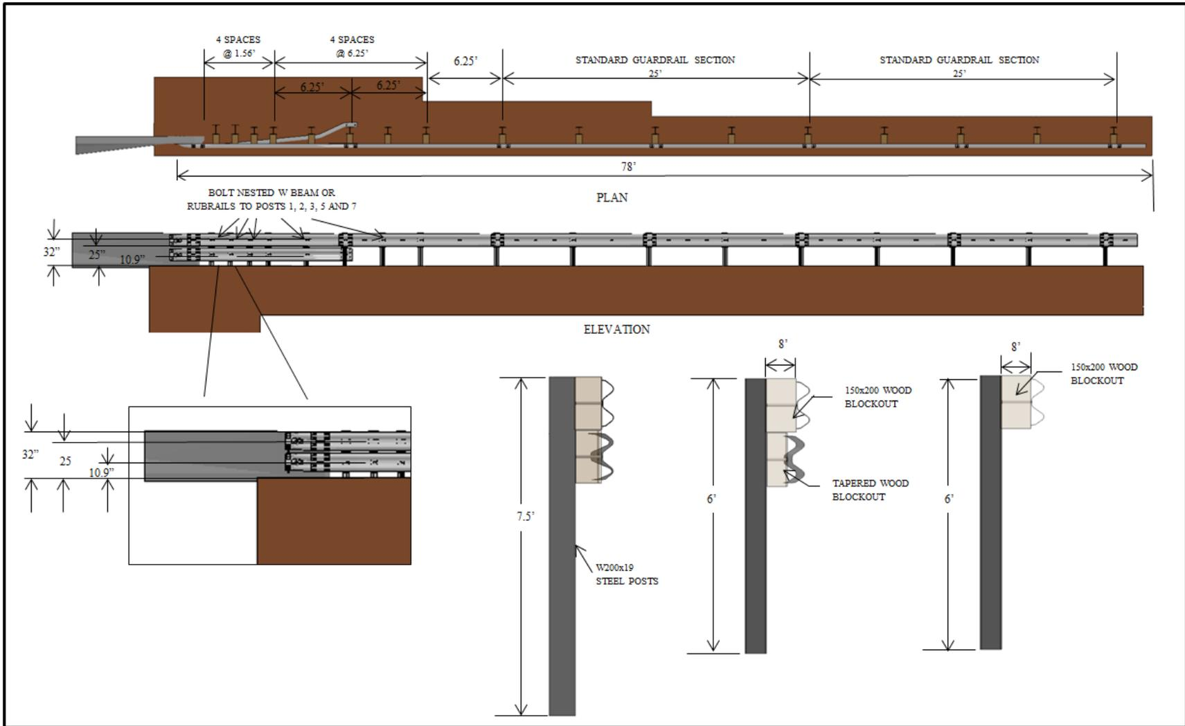
**Figure 3.10. Details of the Vertical Wall Transition Installation for Finite Element Computer Model Simulations (31-in, with Bolts).**
