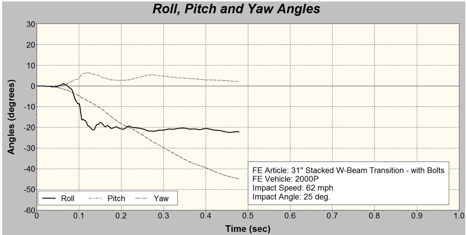
**Figure 3.14. Angular Displacements for FE Simulation of the 31-in High Stacked W-Beam Transition (with Bolts).**
