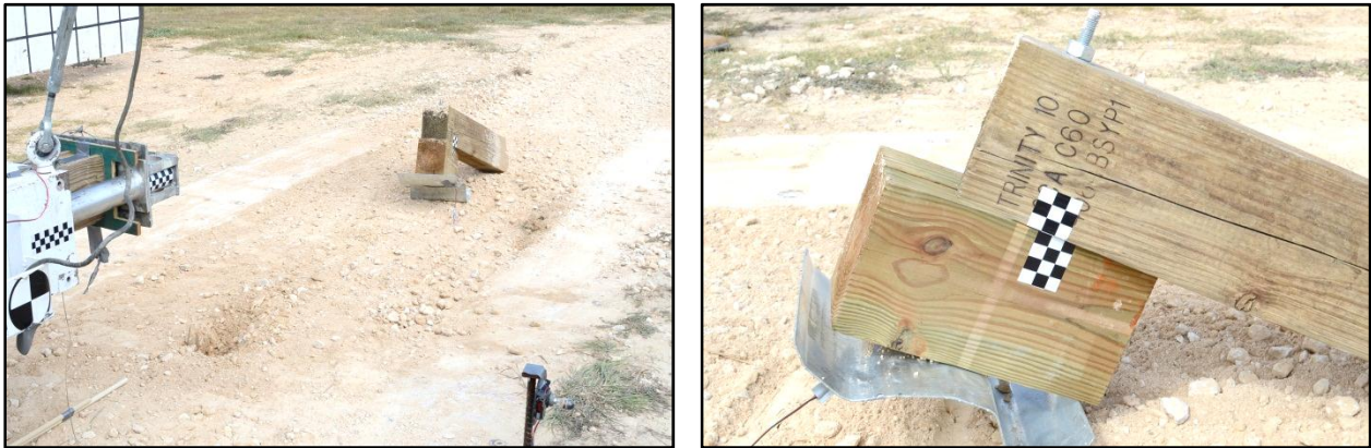
Figure 5. Post and Blockout after Test P2.
