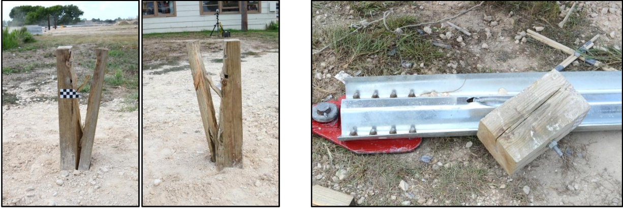
Figure 6. Post and Blockout after Test P3.
