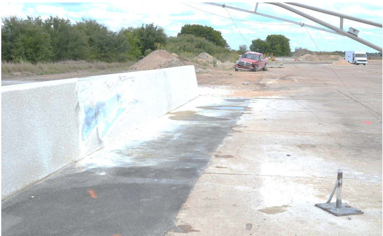
Figure 5.3. Vehicle/Washington Concrete Traffic Barrier with Acoustic Coating Positions after Test No. 602191-1.
