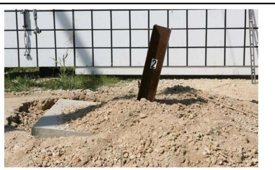
Test P2: Steel posts over underground structure with 48" concrete. AFTER test
