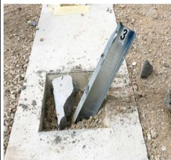
Post in unreinforced concrete wedge after test
