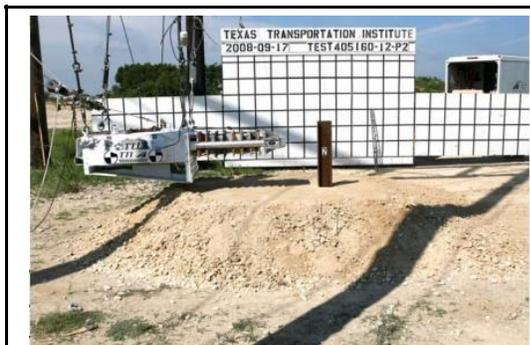
Test P2: Steel posts over underground structure with 48" concrete. BEFORE test
