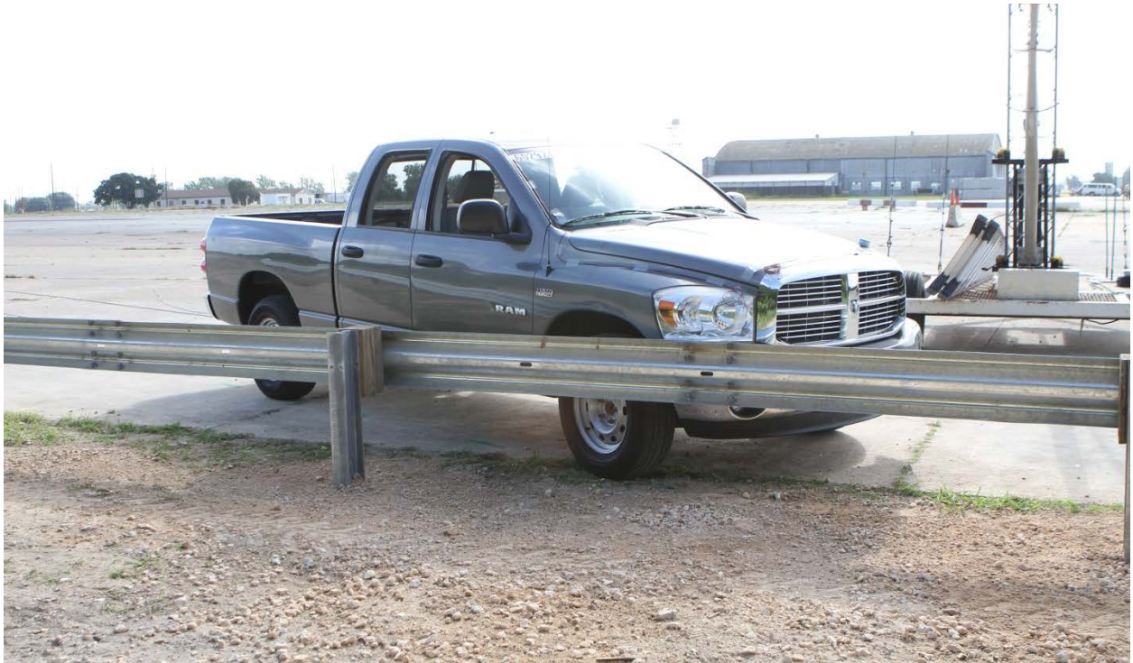
Figure 5.1. Vehicle and Installation Geometrics for Test No. 602921-1.
