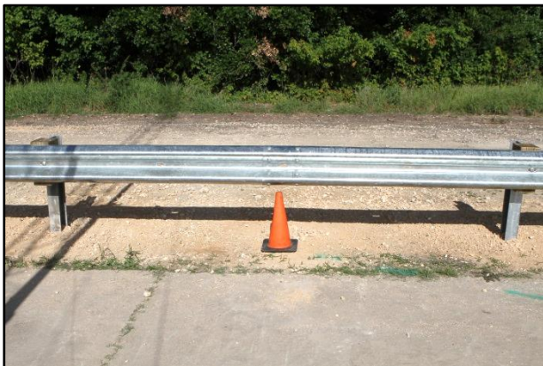
Figure 2.2. 31-inch Guardrail with 12 ft 6 inch Post Spacing Prior to Testing.
