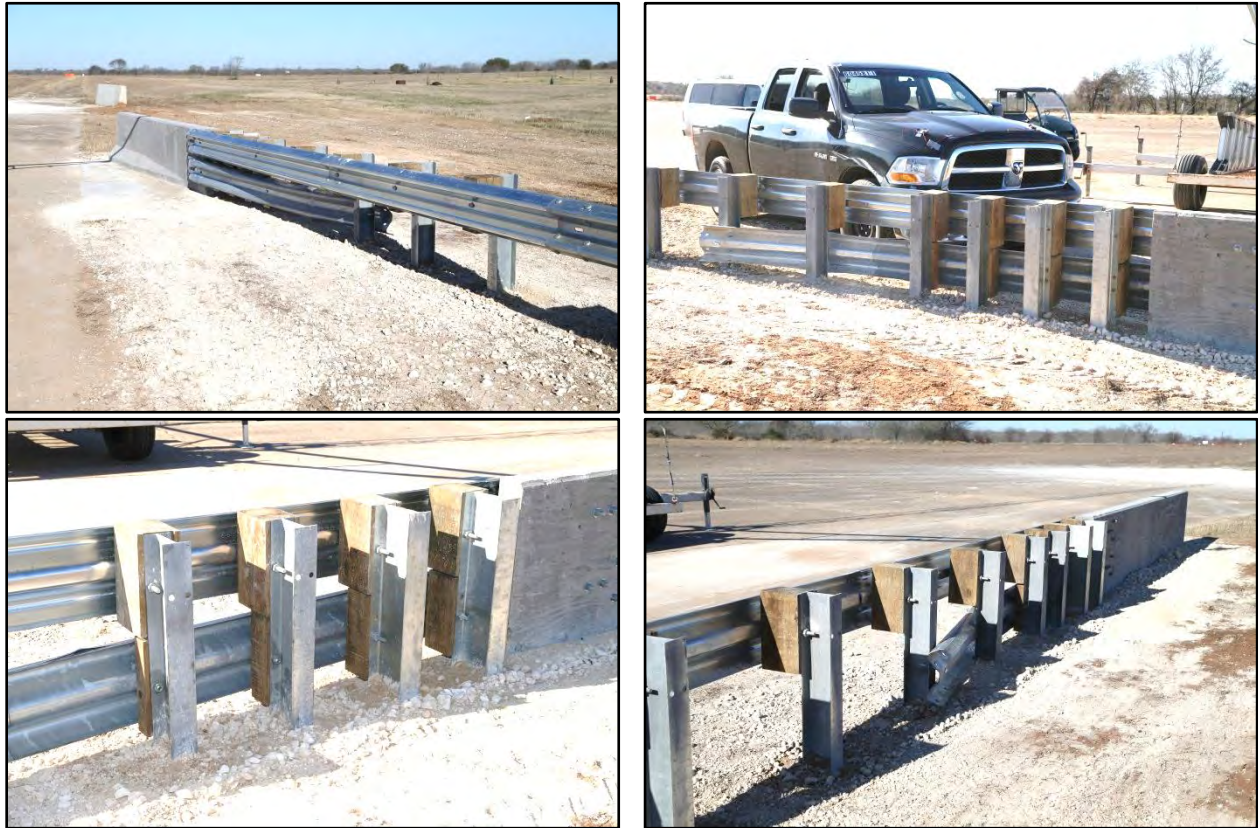
Figure 1. Stacked W-Beam Transition before Test No. 604581-1.
