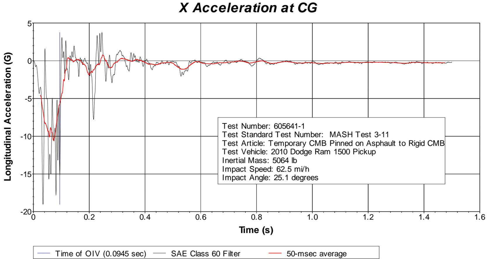
**Figure C.4. Vehicle Longitudinal Accelerometer Trace for Test No. 605641-1
