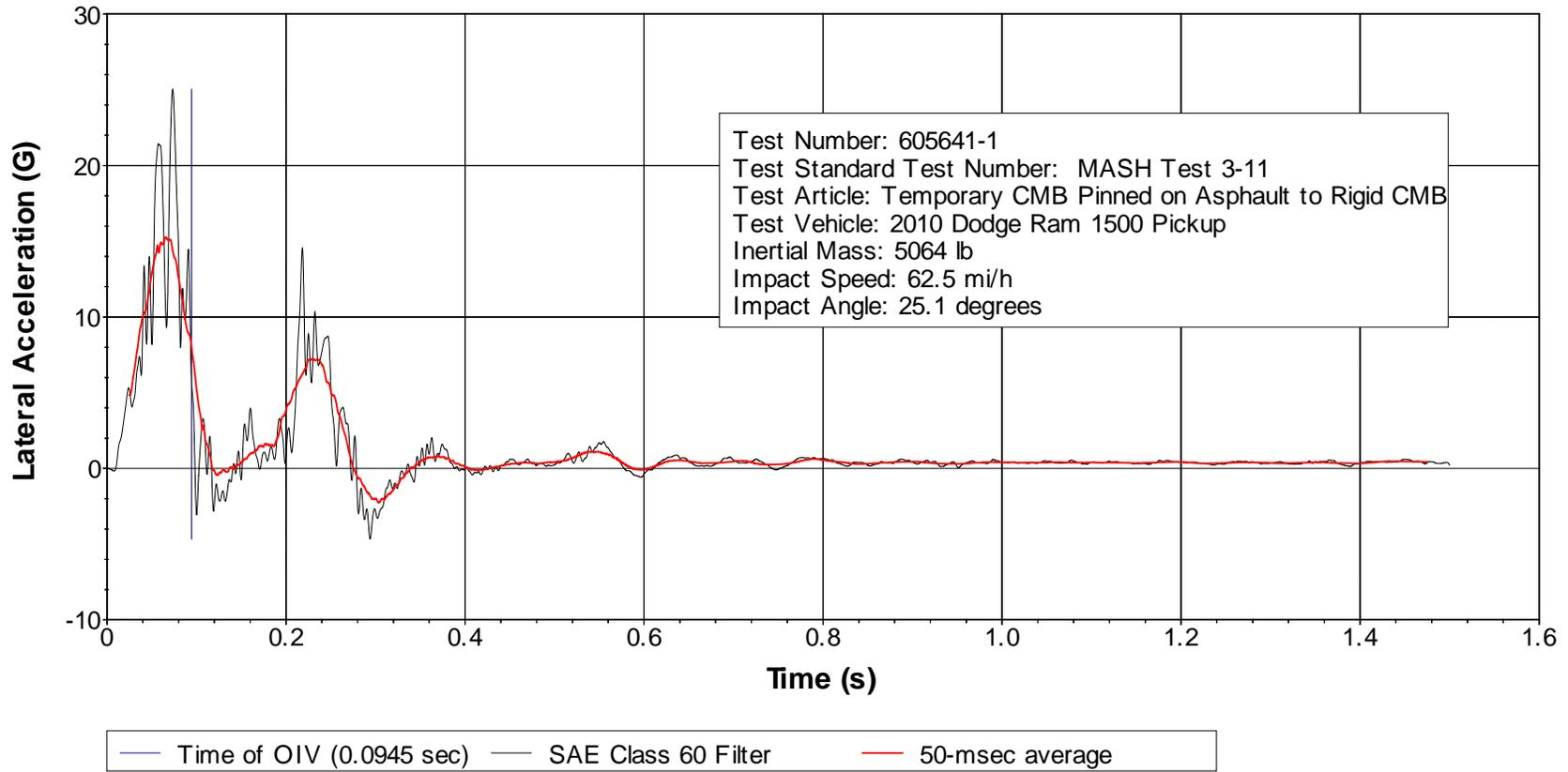
**Figure C.5. Vehicle Lateral Accelerometer Trace for Test No. 605641-1 (Accelerometer Located at Center of Gravity).**
