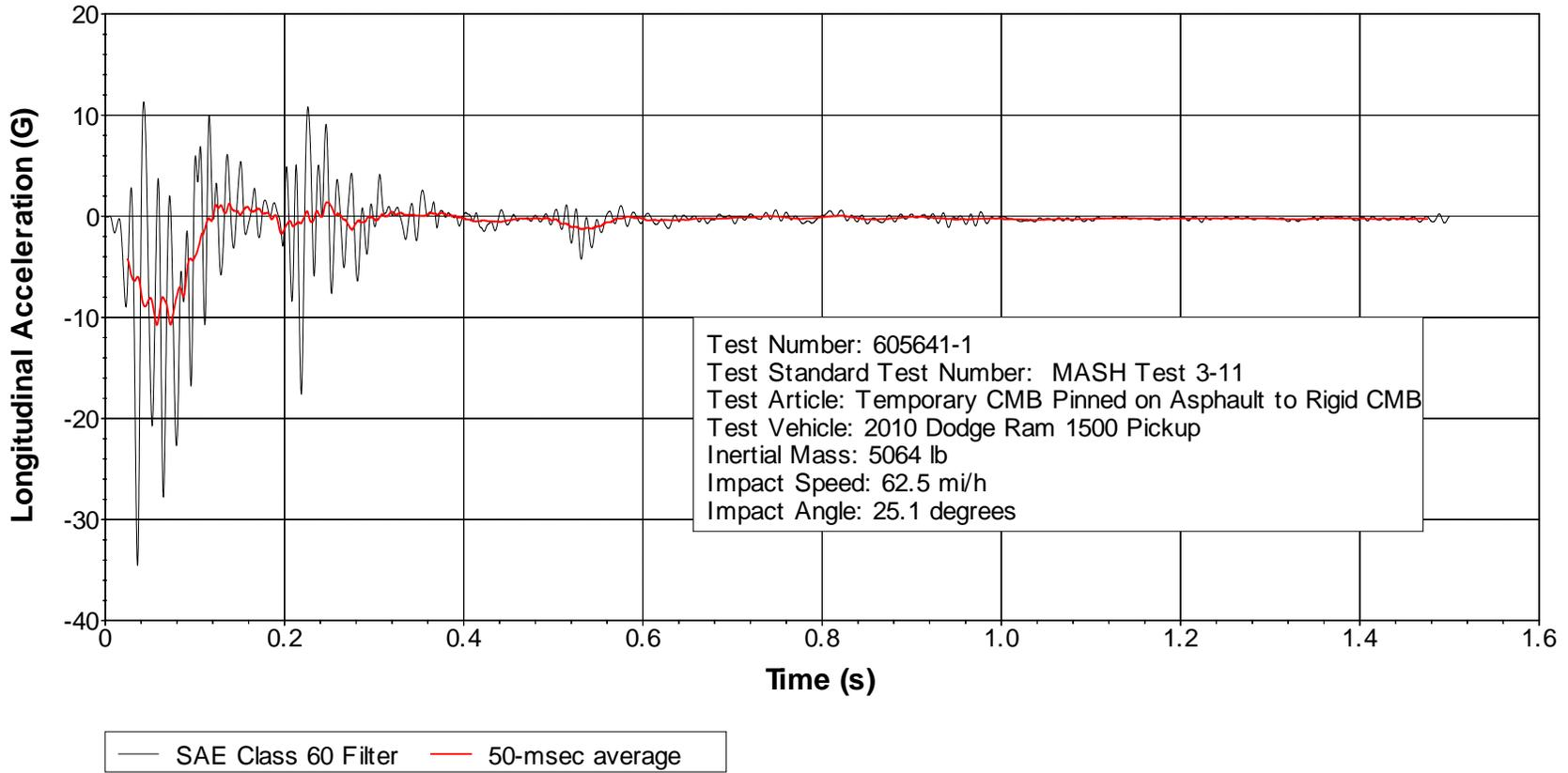
**Figure C.7. Vehicle Longitudinal Accelerometer Trace for Test No. 605641-1 (Accelerometer Located Rear of Center of Gravity).**
