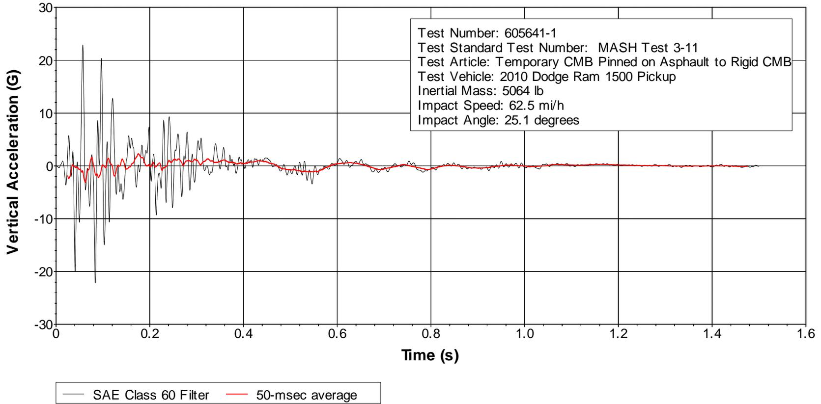
**Figure C.9. Vehicle Vertical Accelerometer Trace for Test No. 605641-1
