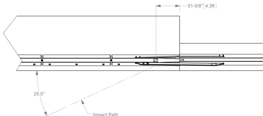
**Figure 3.1. CIP for Transition from Temporary Concrete Barrier Pinned on Asphalt to Rigid Concrete Barrier.**
