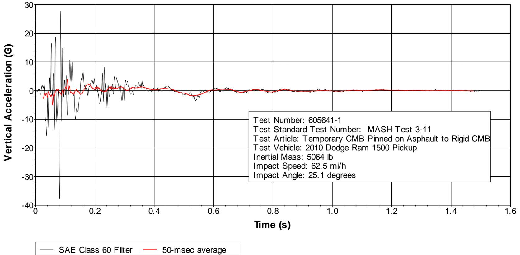
**Figure C.6. Vehicle Vertical Accelerometer Trace for Test No. 605641-1 (Accelerometer Located at Center of Gravity).**
