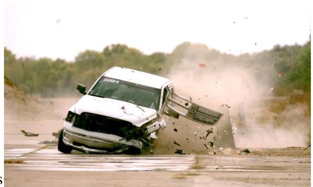
**Figure C.1. Sequential Photographs for Test No. 605641-1 (Overhead and Frontal Views) (Continued).**
