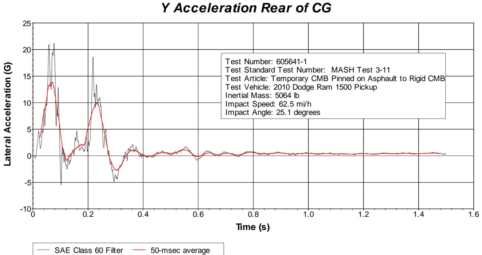
**Figure C.8. Vehicle Lateral Accelerometer Trace for Test No. 605641-1
