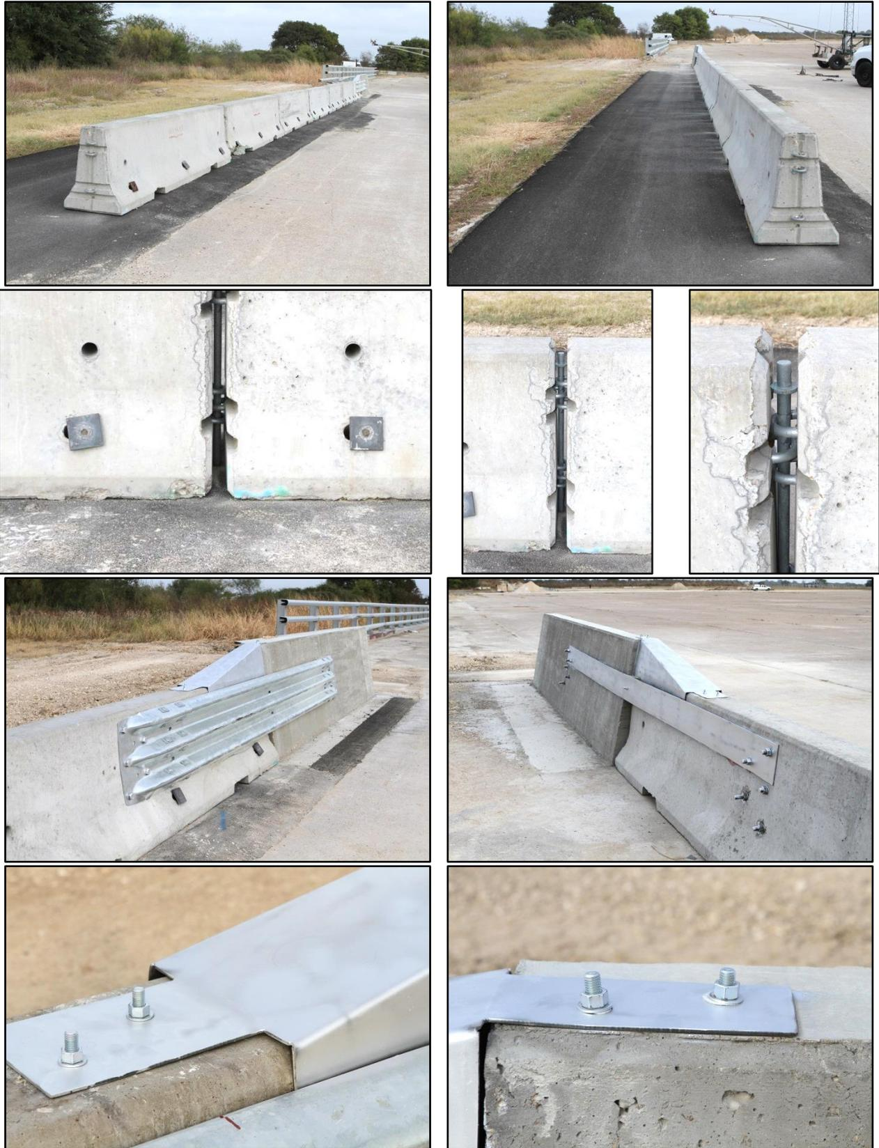
**Figure 2.2. Transition Installation prior to Testing.**
