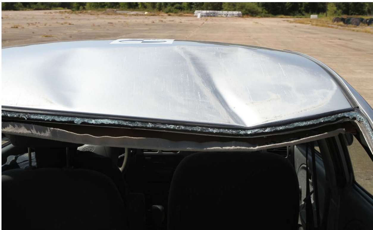
Figure 9.58. Vehicle Roof Deformation after Test No. 463631-3.
