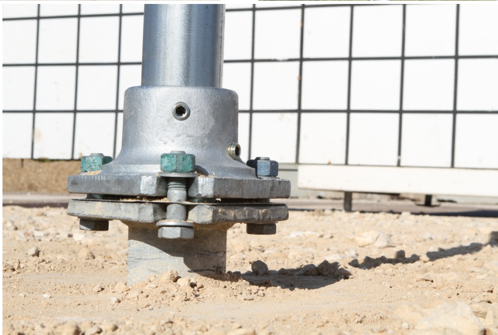
Figure 9.52. Sign Support System prior to Test No. 463631-3.
