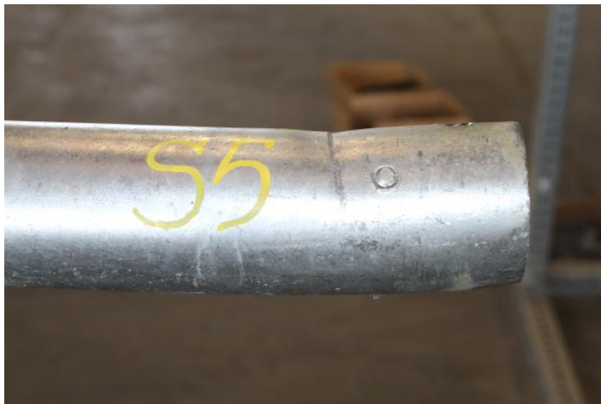
Figure 11.16. Deformation to Schedule 80 Pipe Support.
