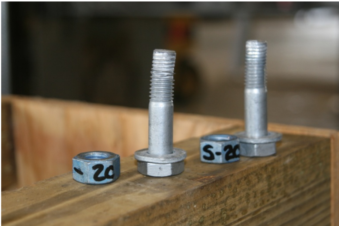
Figure C8. Slip Bolts after Test S20.
