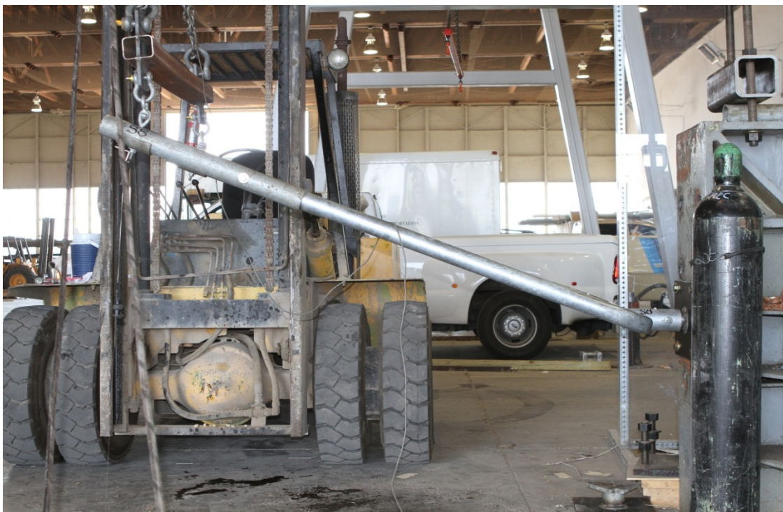
Figure 11.20. U-Bracket Static Test Setup at Maximum Load.
