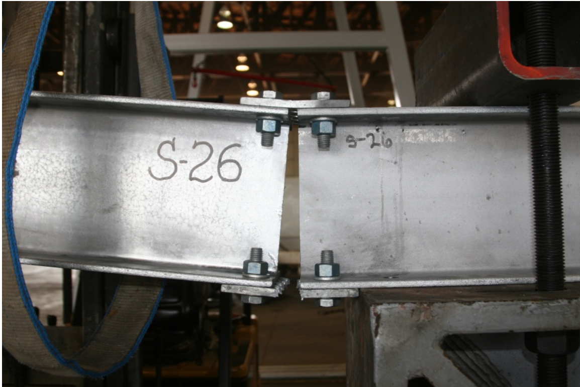
Figure C9. Test Sample S26 after Fuse Plate Rupture.
