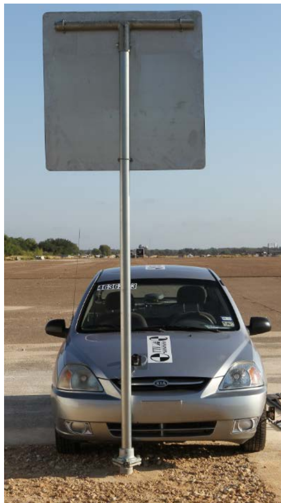
Figure 9.53. Vehicle/Installation Geometrics for Test No. 463631-3.
