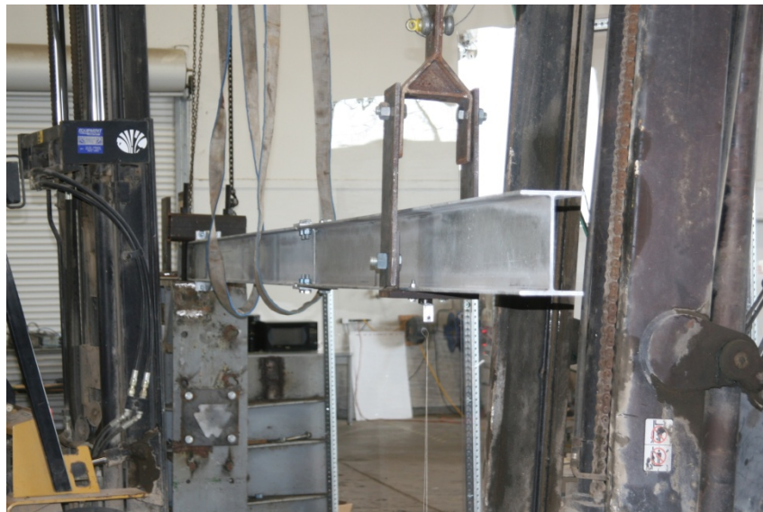
Figure 5.12. W8×18 Support Ready for Load Application (S3).
