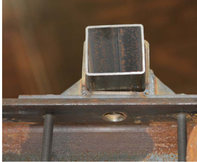
Figure 7.9. Static Test of HSS3×3×1/8 with Bracket Connection.
