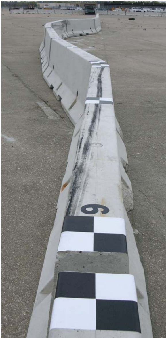
Figure 22. Temporary Barrier Damage, Test 2214TB-2
