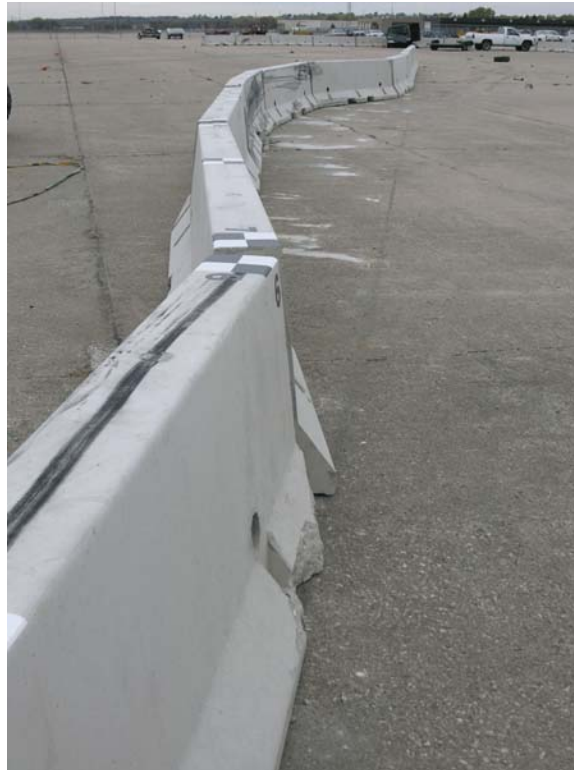
Figure 21. Vehicle Final Position and Trajectory Marks, Test 2214TB-2
