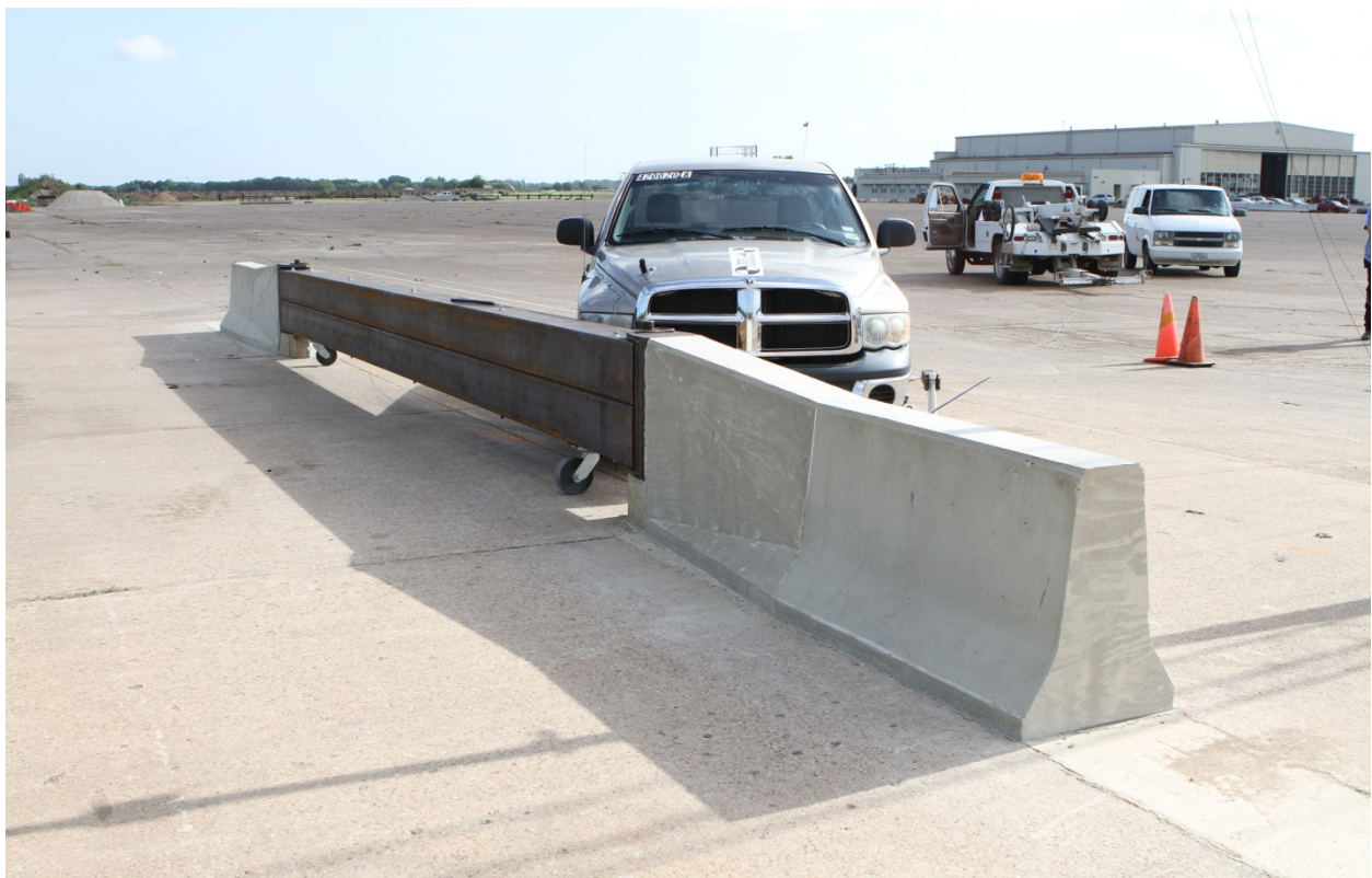
Figure 8.1. Vehicle/Gate Geometrics for Test No. 420020-8.
