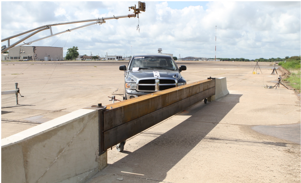
Figure 7.1. Vehicle/Gate Geometrics for Test No. 420020-7.
