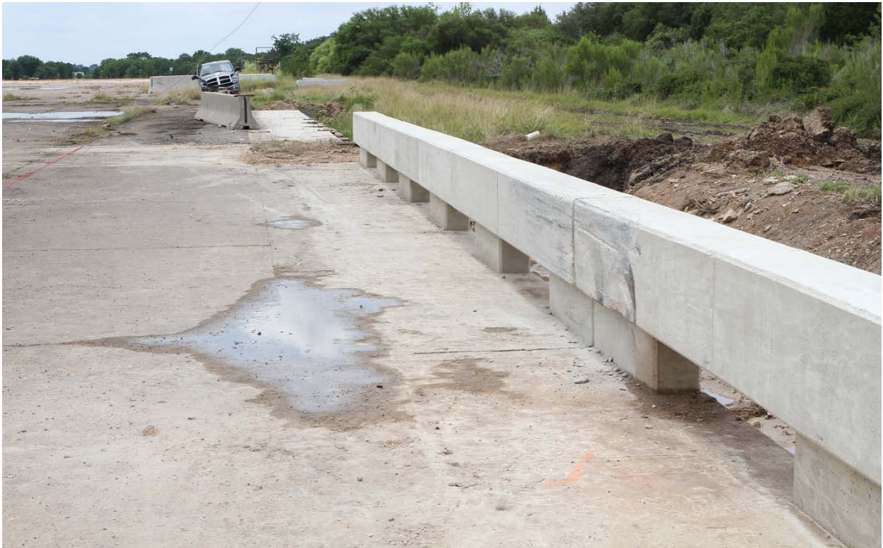
Figure 7.3. After Impact Vehicle/Barrier Positions for Test No. 420021-5.
