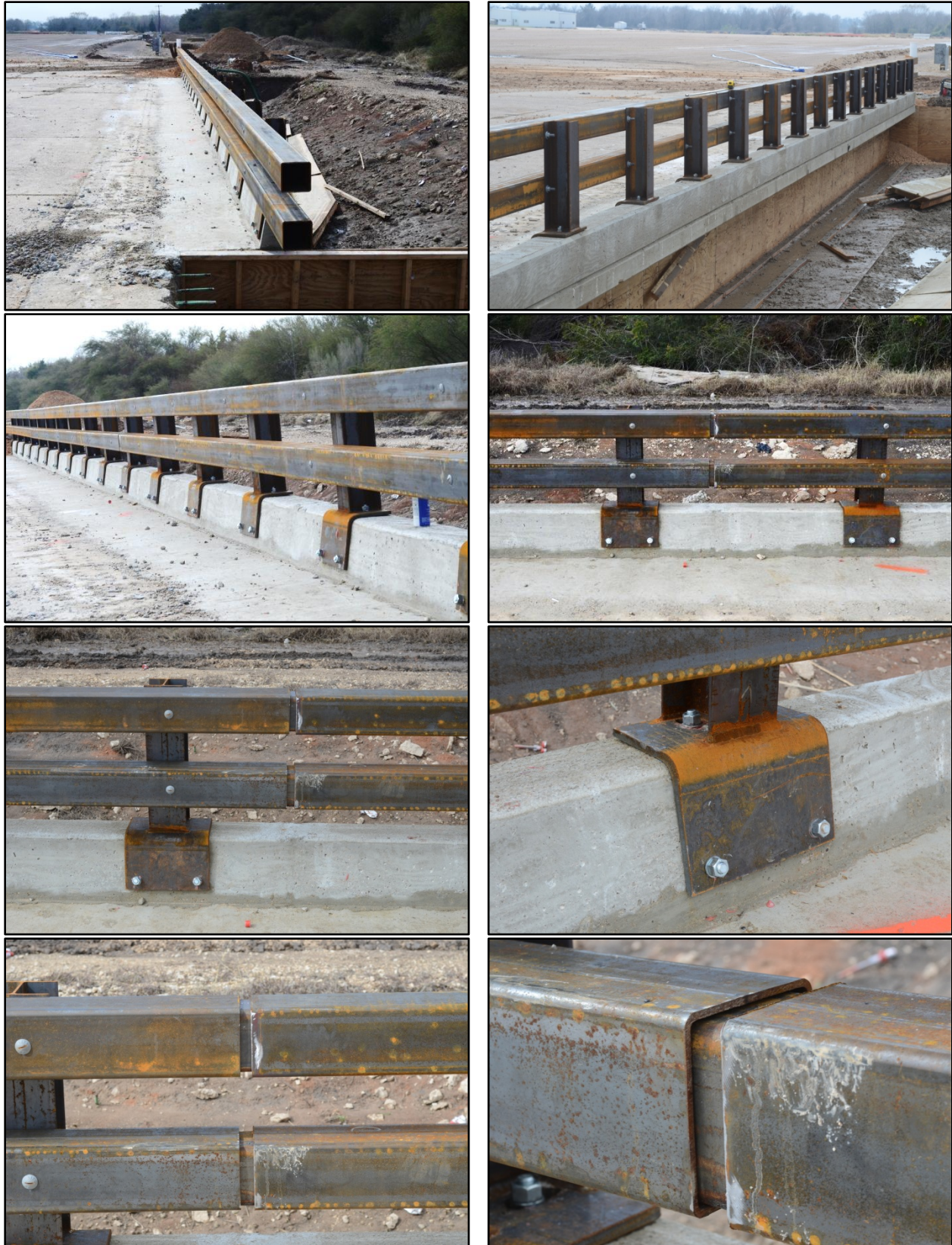
Figure 2.3. T131RC Bridge Rail Installation before Test No. 490022-1.
