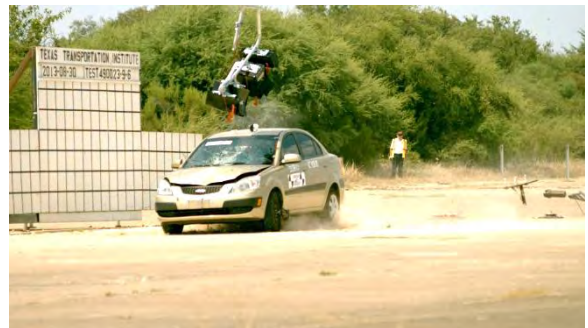
Figure F1. Sequential Photographs for Test No. 490023-9-6 (Perpendicular and Oblique Views) (Continued).
