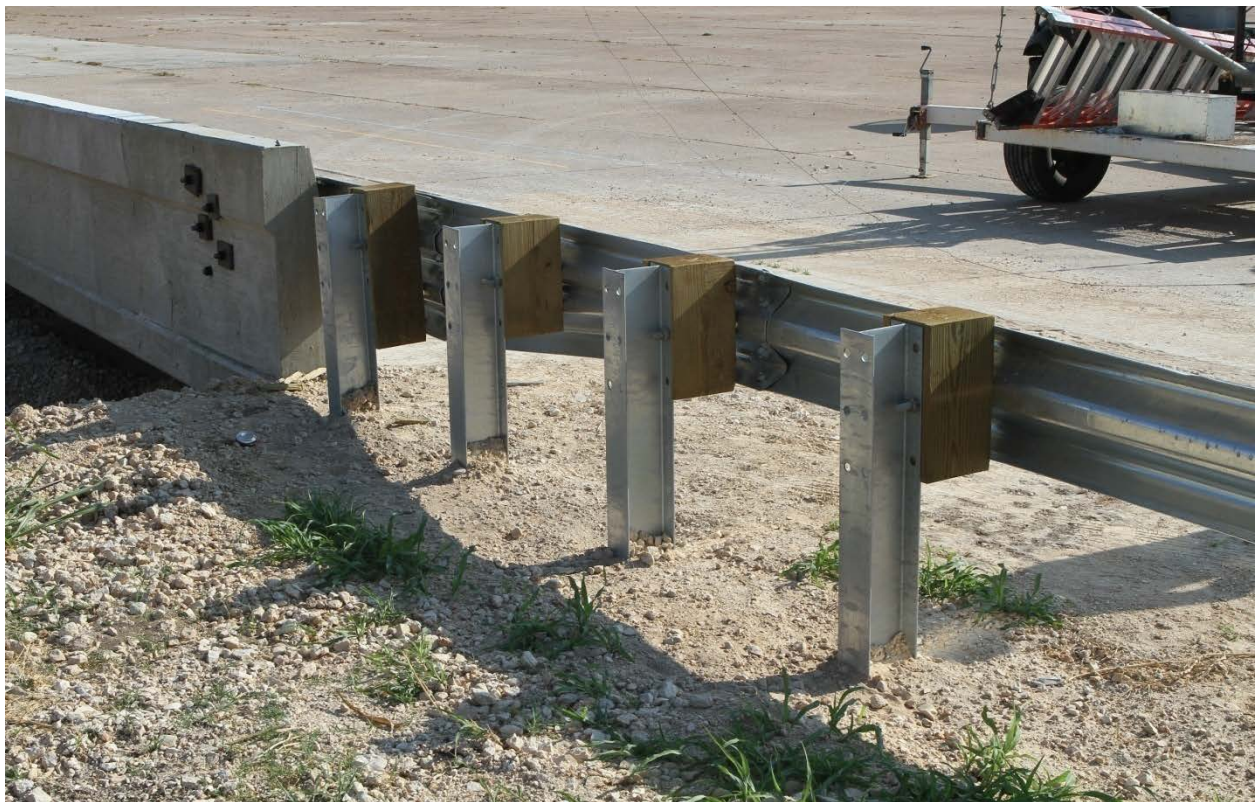
Figure 3.2. MASH TL-2 Transition before Test No. 420021-4.
