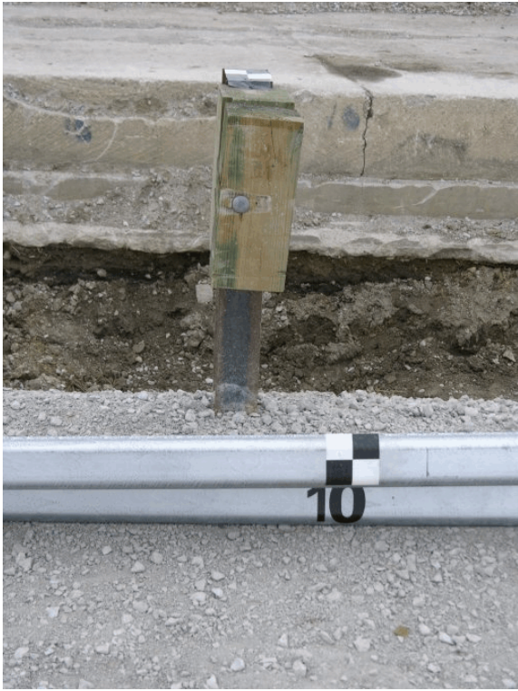
Figure 60. Post Nos. 9 through 12 Damage, Test No. MGS221-2
