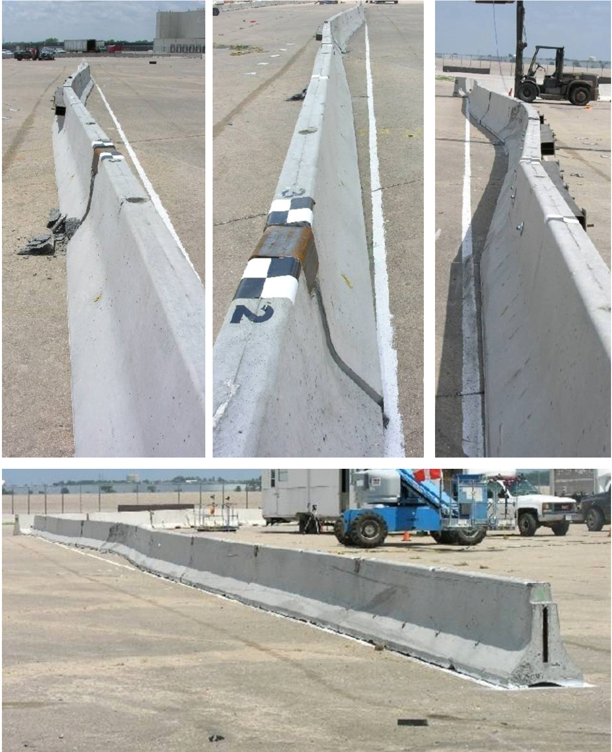
Figure 37. Temporary Barrier Damage, Test NYTCB-1
