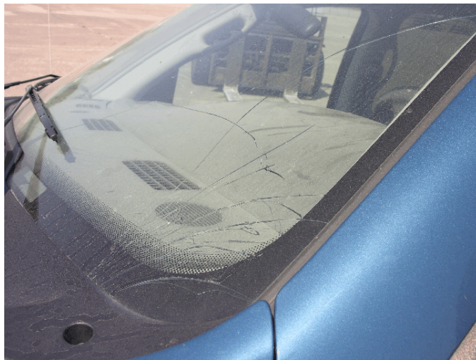
Figure 86. Additional Vehicle Damage, Test NYTCB-3
