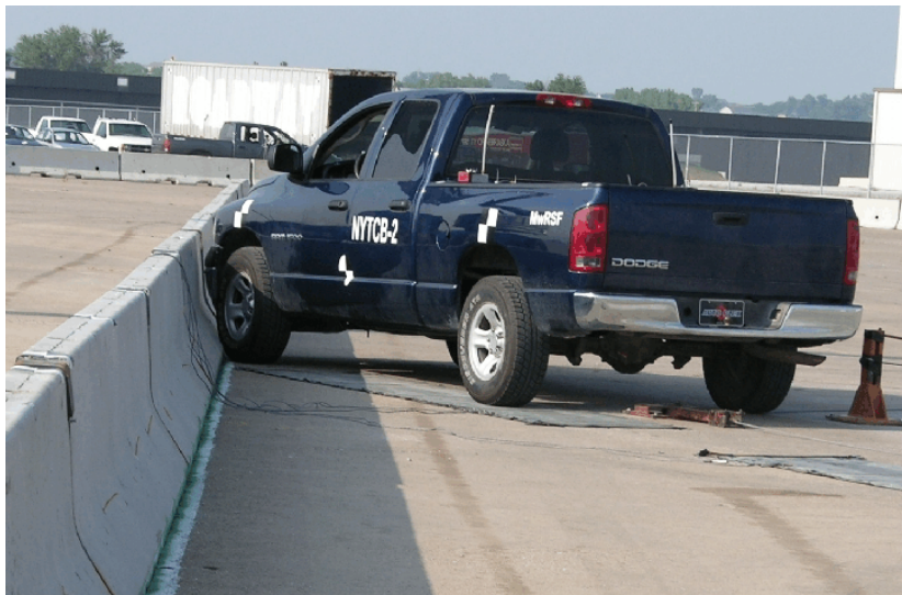
Figure 56. Impact Location, Test NYTCB-2
