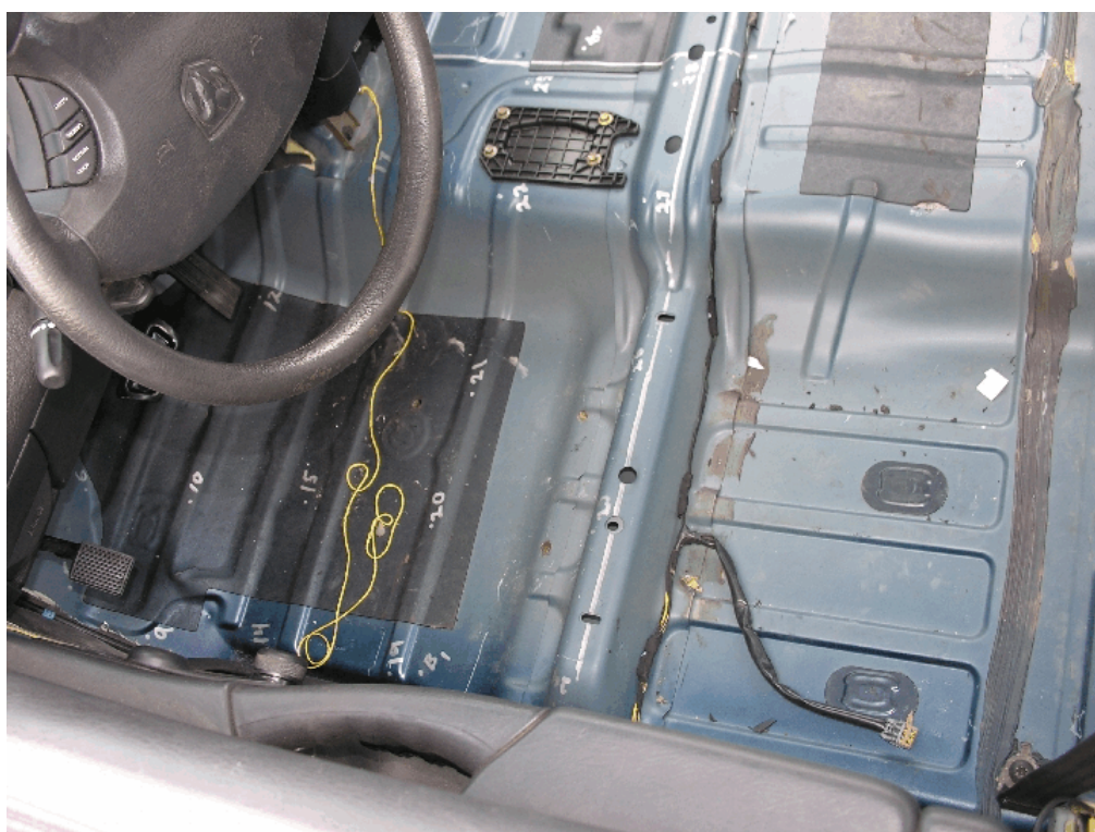
Figure 64. Occupant Compartment Deformation, Test NYTCB-2
