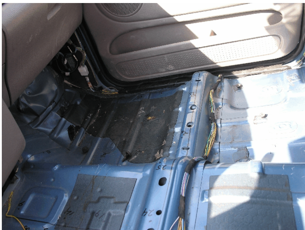
Figure 87. Occupant Compartment Deformation, Test NYTCB-3
