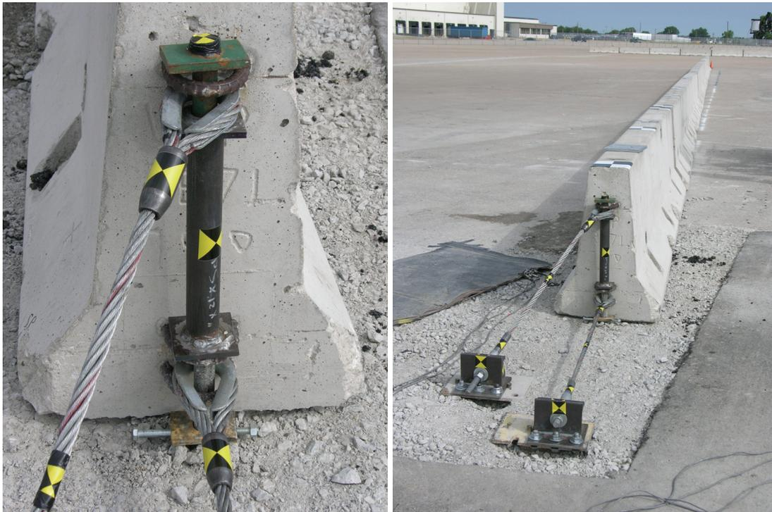
**Figure 2. Termination of TCB, Test No. TTCB-1**
