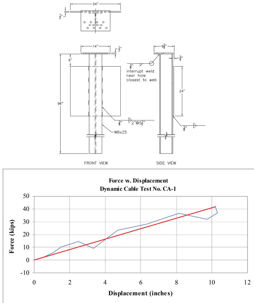
Figure 1. Single Driven Steel Pile Anchorage
