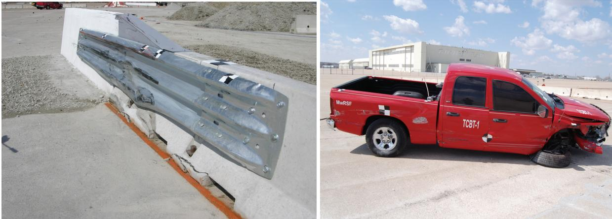
**Figure 8. Post Test Damage, Test No. TCBT-1**
