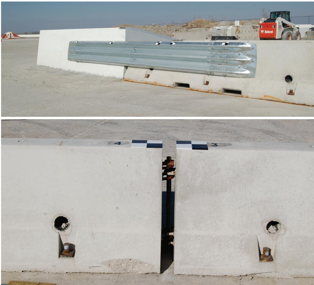
**Figure 6. TCB Approach Transition to 42-in. High Single-Slope Barrier**
