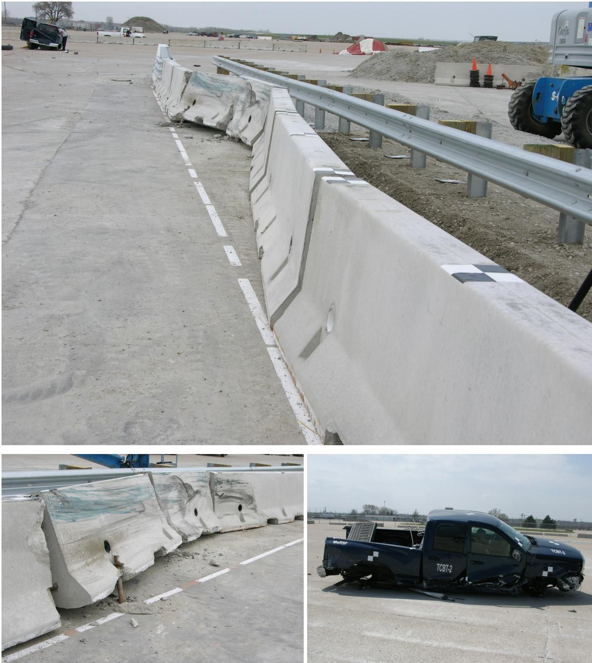
**Figure 10. Post Test Damage, Test No. TCBT-2**
