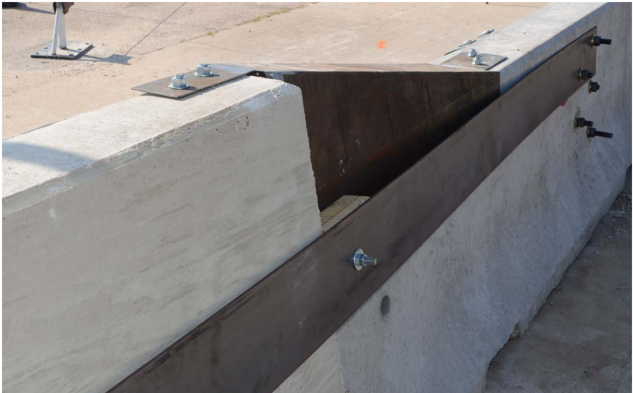
Figure 3.2. Transition design for anchored temporary barrier to rigid concrete barrier prior to testing.
