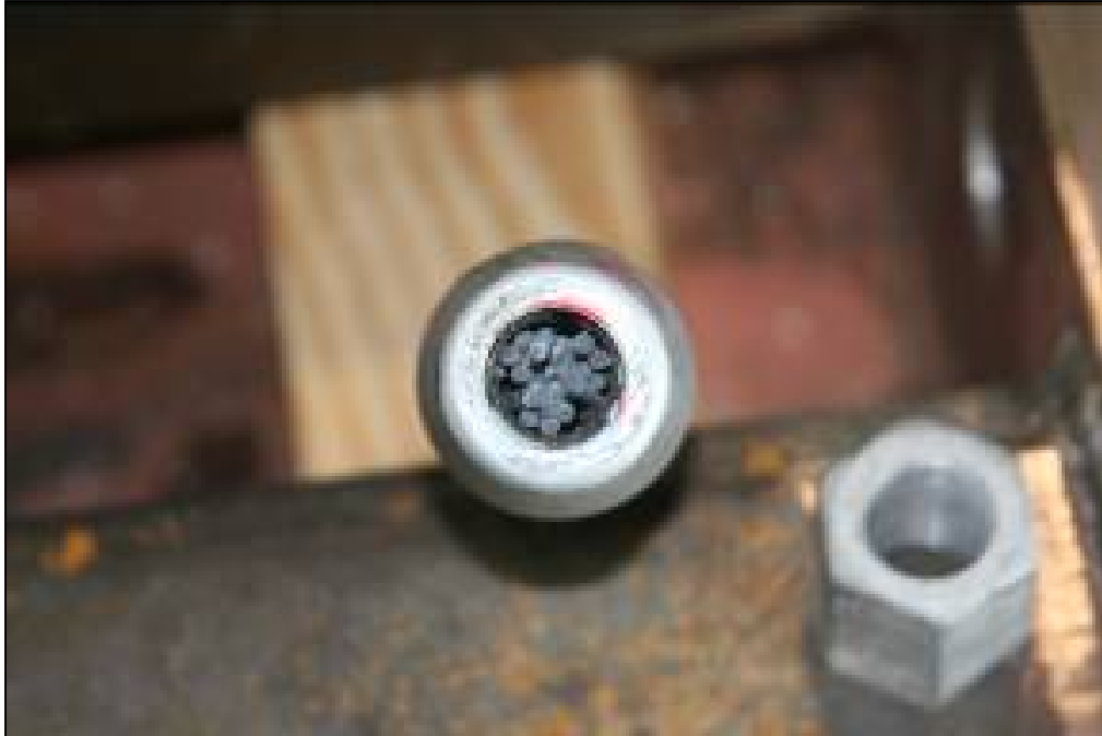
Figure 3.18. Nucor Steel Marion wire rope termination B (end view) after test NSM-S31.
