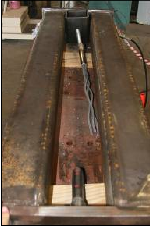
Figure 3.8. Field Swage wire rope terminations after test S7.
