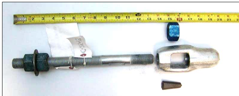
Figure 2.2. Exploded view of assembly (Assembly Specialty Products, Inc.).
