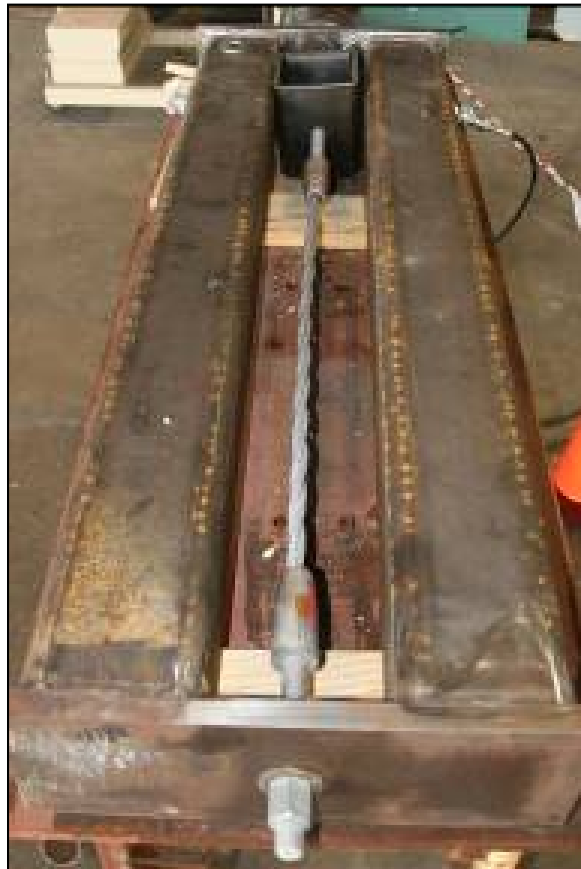
Figure 3.1. Static load frame with test sample installed and ready for testing.
