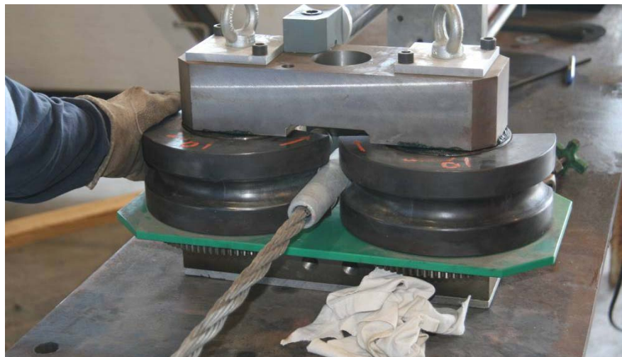
Figure 9. Image of a Proper Hand Placement during Wire Rope Swaging Process.
