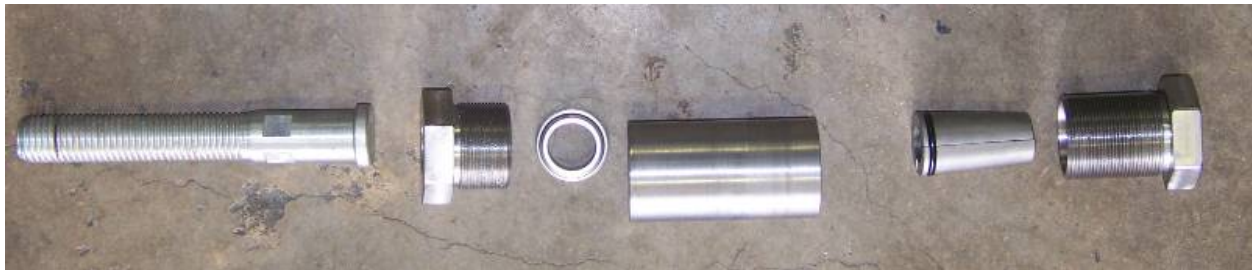
Figure 2.10. Exploded view of the components of Precision Sure-Lock Prototype 2.
