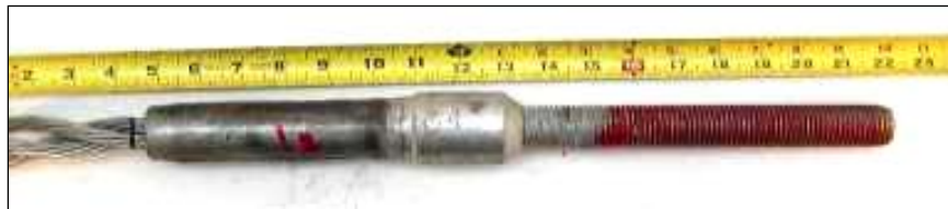
Figure 2.4. Field swaged termination that has been previously tested.
