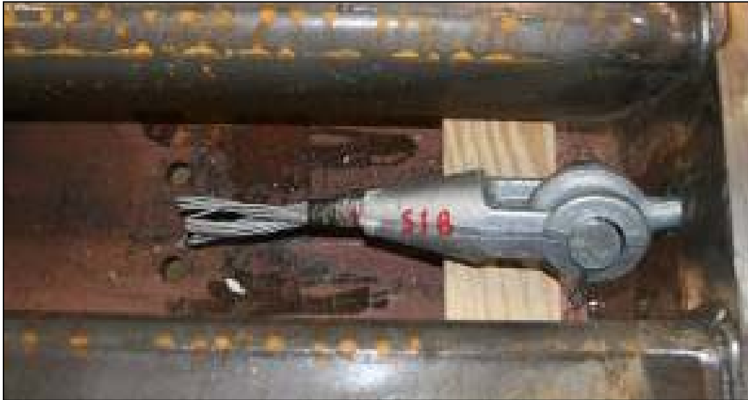
Figure 3.3. Epoxy Socket wire rope termination B after test S1.
