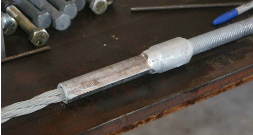
Figure 9. Image of a Properly Swaged Termination.
