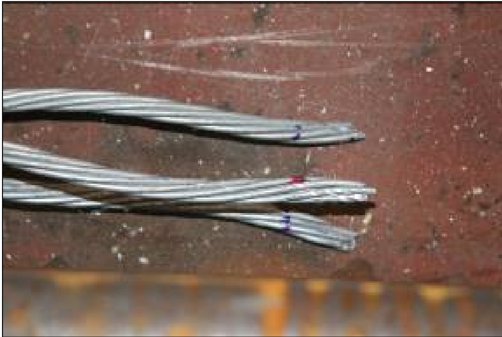
Figure 3.6. Field Swage wire rope termination A after test S3.
