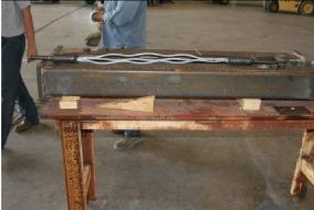
Figure 3.15. Precision Sure-Lock Prototype 2 wire rope terminations after test S6.
