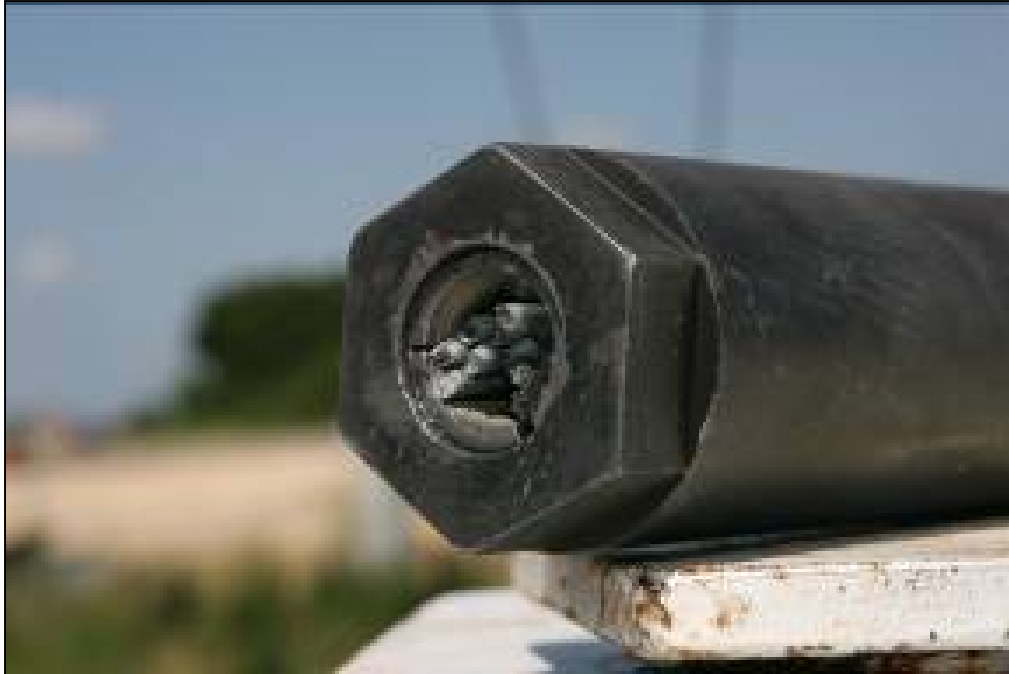
Figure 3.28. Precision Sure-Lock Prototype 2 wire rope termination A after test P6.
