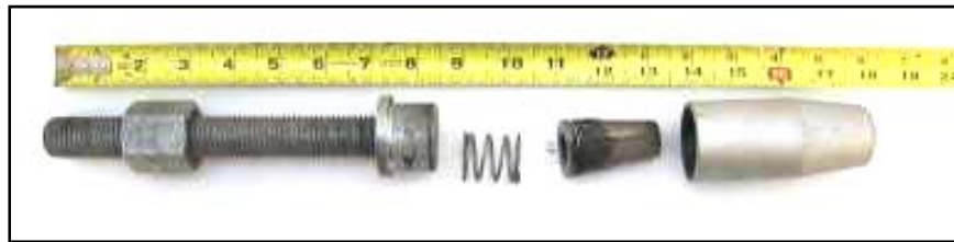
Figure 2.8. Exploded view of Nucor Steel Marion assembly.
