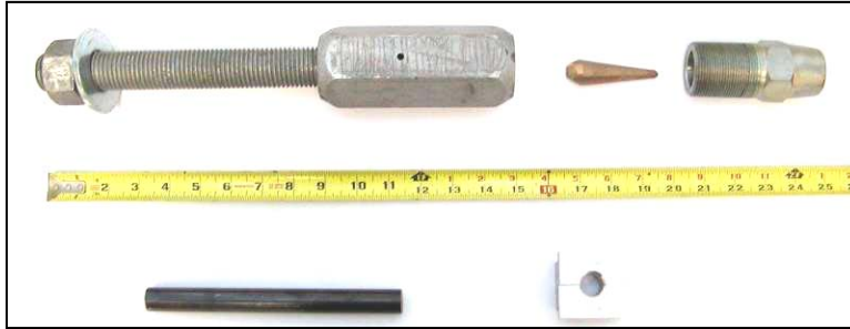
Figure 2.7. Exploded view of Electroline (by ESMET, Inc.) assembly.
