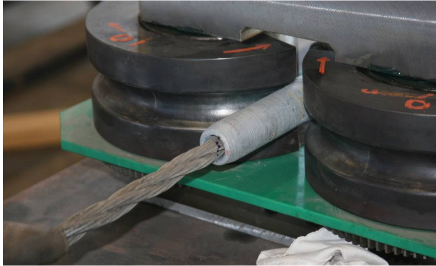
Figure 8. Image of a Properly Embedded Wire Rope Ready for Swaging.
