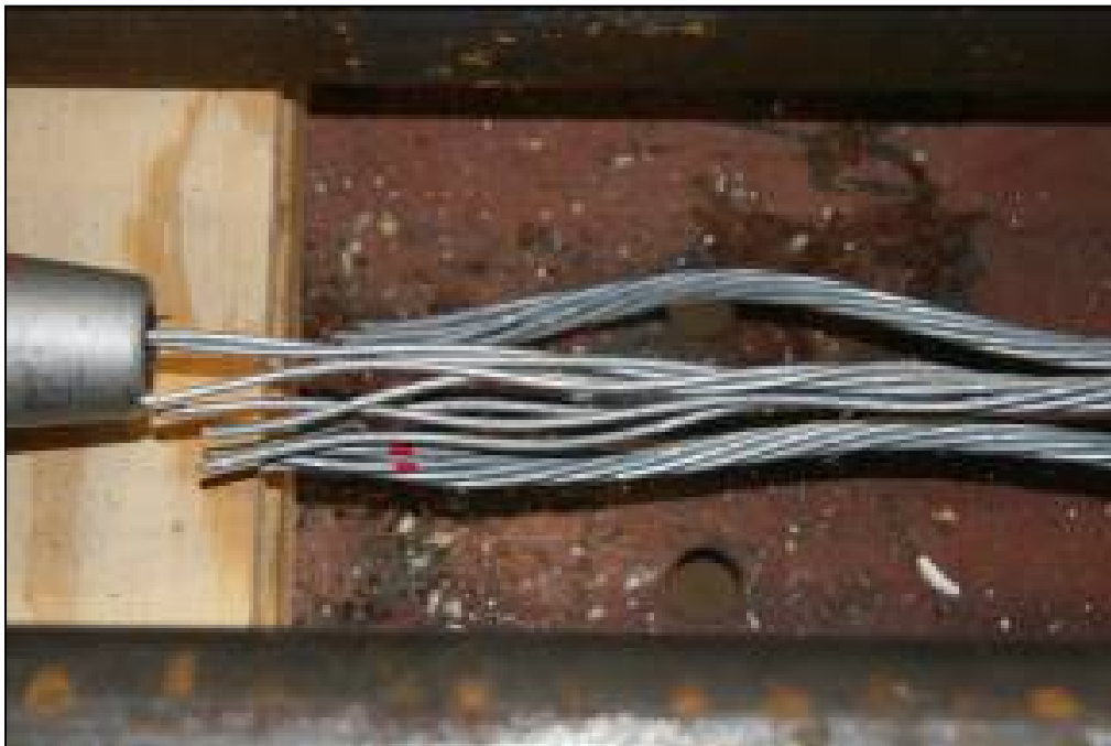
Figure 3.17. Nucor Steel Marion wire rope termination A after test NSM-S30.
