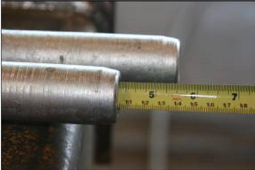
Figure 3.10. Example of an incorrect embedment depth of a Field Swage termination due to zinc plug in termination.
