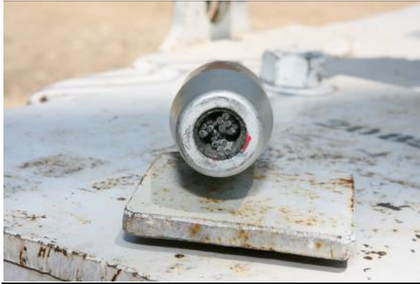
Figure 3.32. Nucor Steel Marion wire rope termination A after test NSM-P16.
