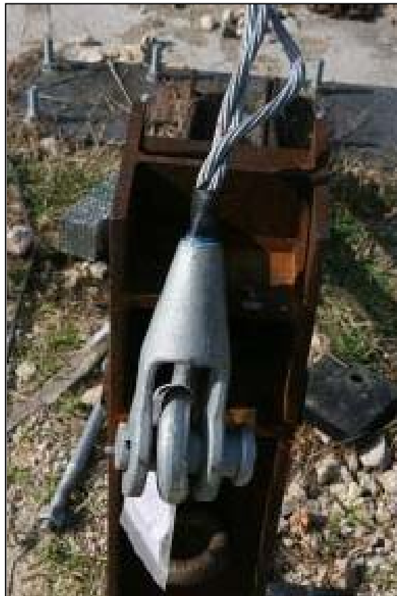
Figure 3.22. Epoxy Socket wire rope termination B after test P1.
