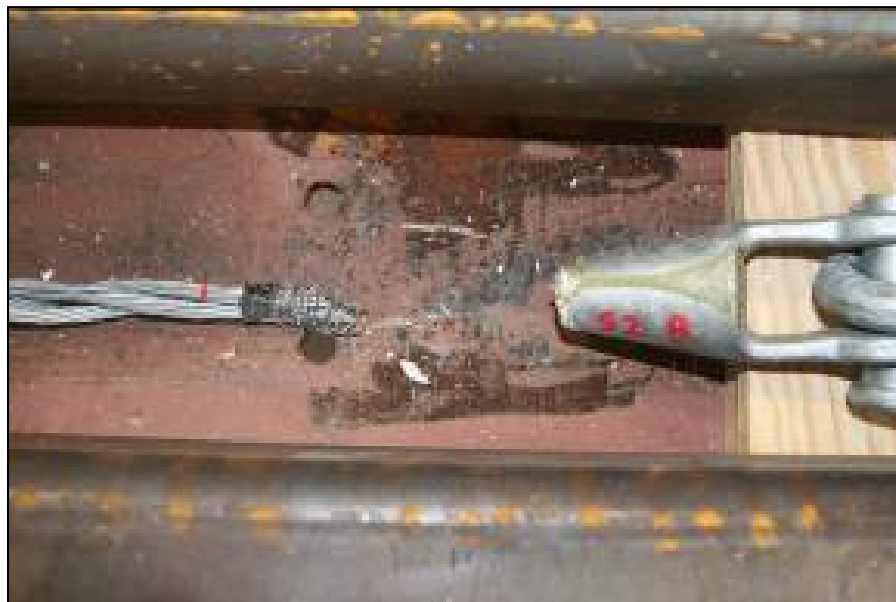
Figure 3.4. Epoxy Socket wire rope termination B after test S2.
