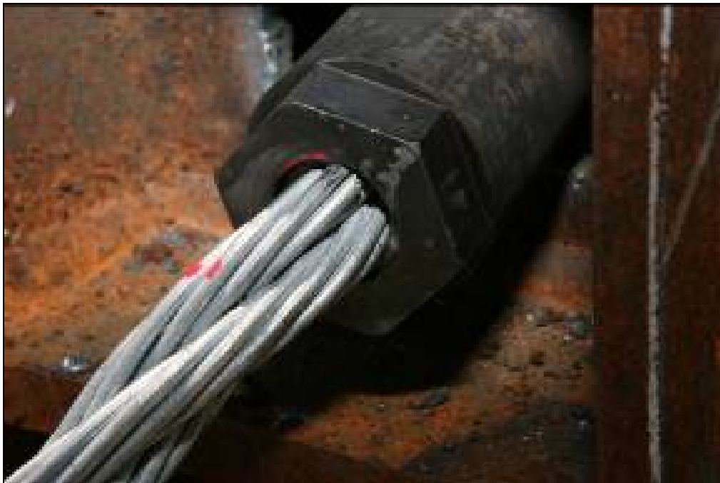
Figure 3.29. Precision Sure-Lock Prototype 2 wire rope termination B after test P6.
