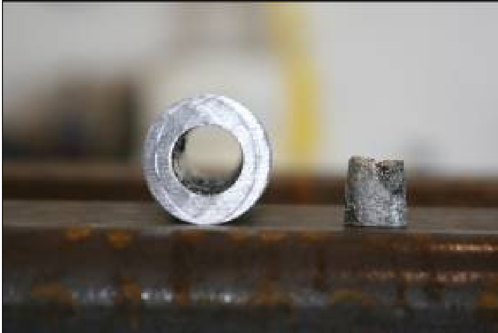
Figure 3.12. Field Swage termination cross-section with galvanization plug.
