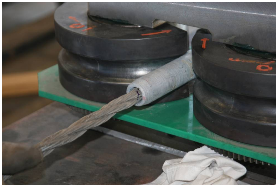
Figure 6. Image of a Properly Embedded Wire Rope Ready for Swaging.
