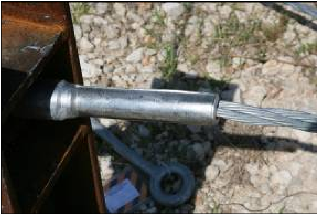
Figure 3.26. Field Swage wire rope termination B after test P4.
