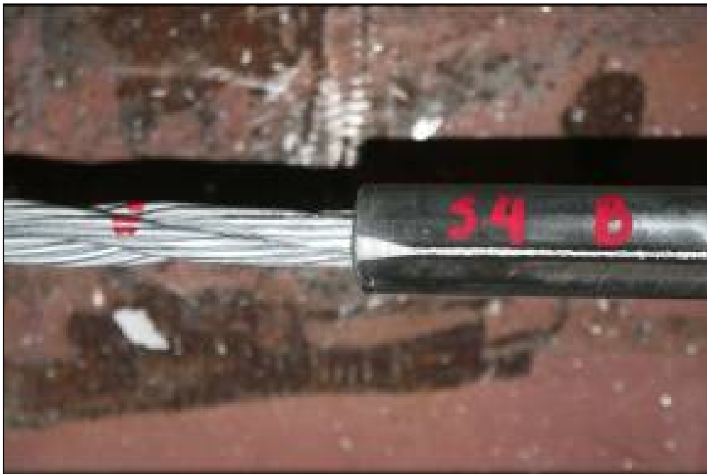
Figure 3.7. Field Swage wire rope termination B after test S4.
