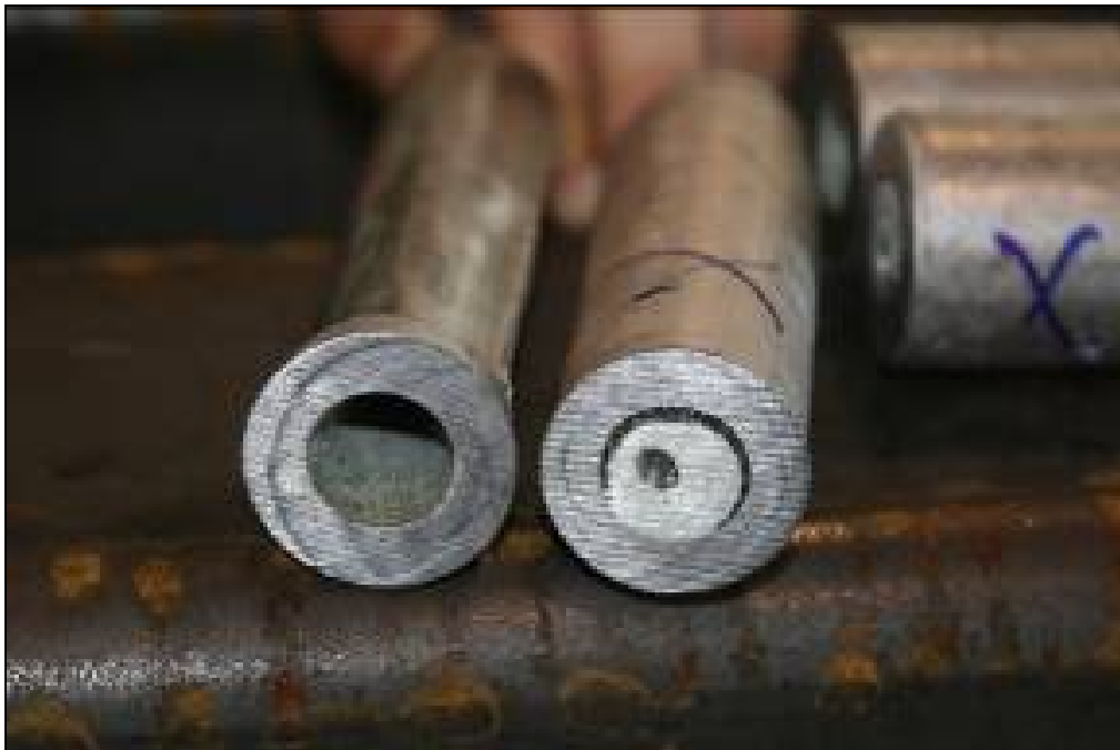
Figure 3.11. Field Swage termination cross-section with and without galvanization plug.
