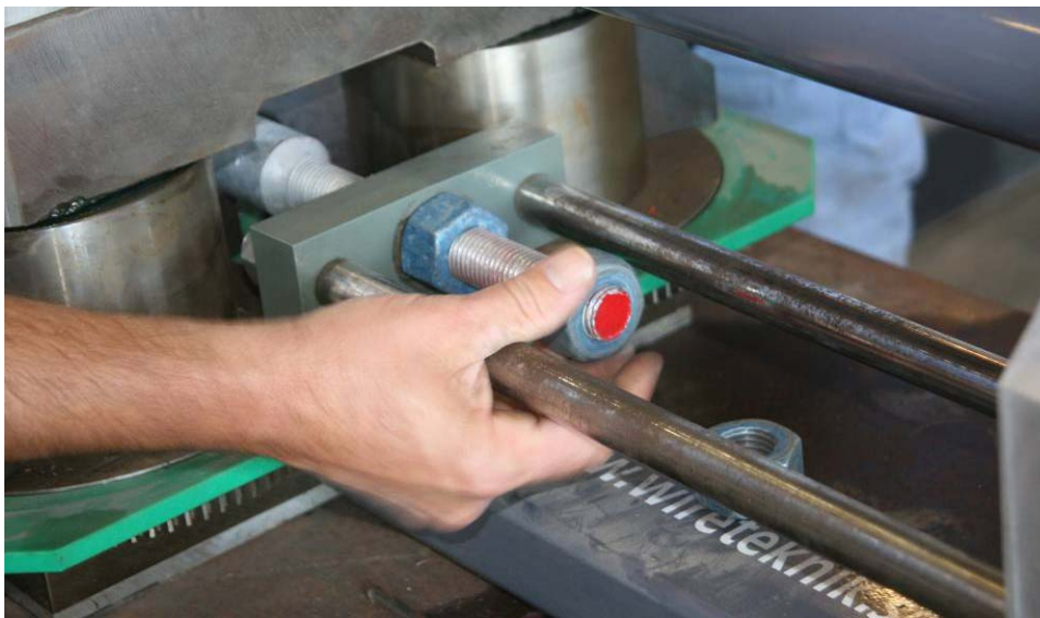
Figure 7. Image of Installation of Field Swage Termination in Swaging Machine.
