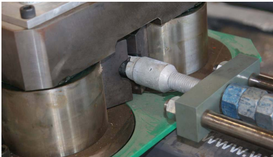
Figure 8. Image Showing Initial Engagement of Compression Dies.
