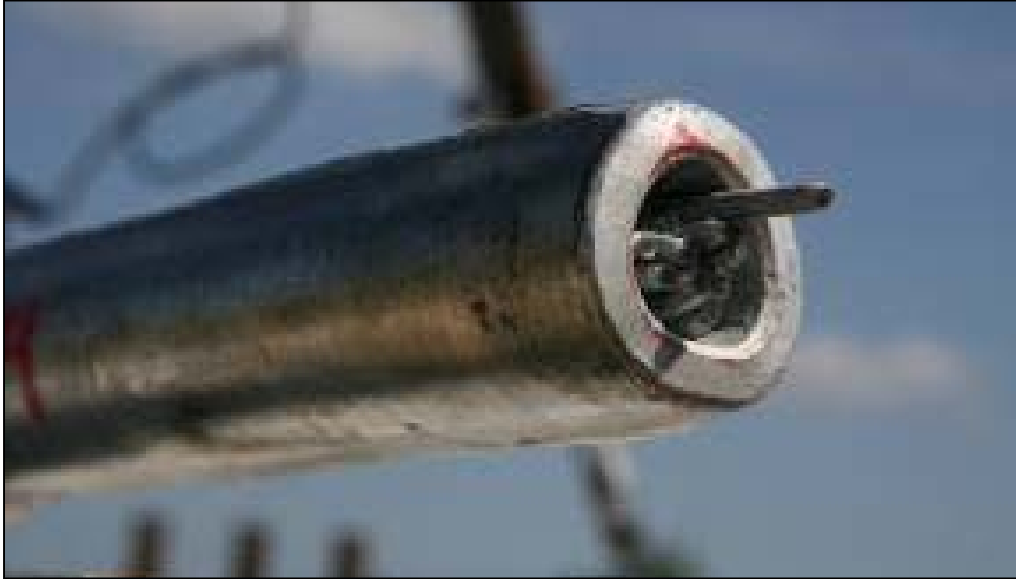
Figure 3.25. Field Swage wire rope termination A after test P4.
