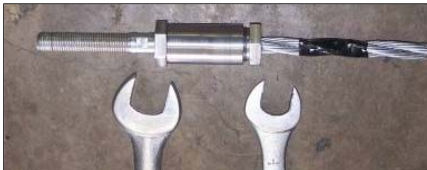
Figure 2.6. Assembled view of the Precision Sure-Lock Prototype 2 termination with required wrenches.
