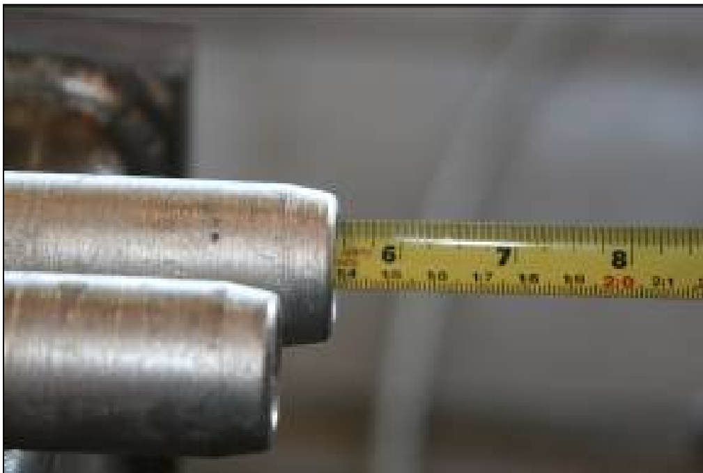
Figure 3.9. Correct embedment depth of a Field Swage termination.
