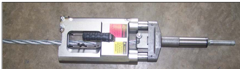
Figure 2.5. Precision Sure-Lock Prototype 1 with tensioning linear jack.
