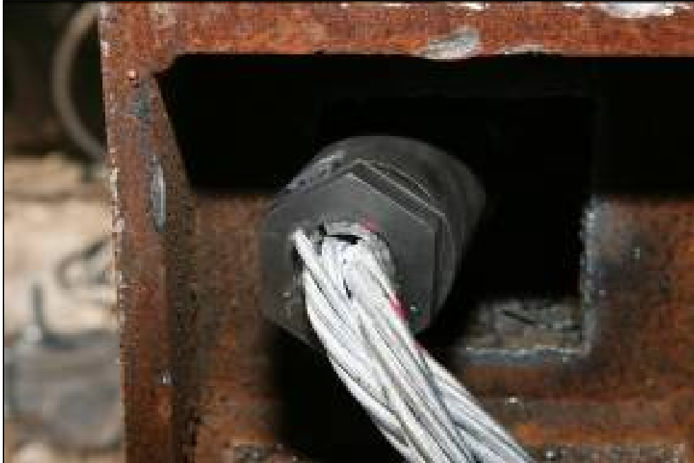
Figure 3.30. Precision Sure-Lock Prototype 2 wire rope termination B after test P7.
