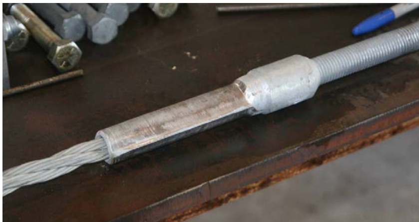
Figure 11. Image of a Properly Swaged Termination
