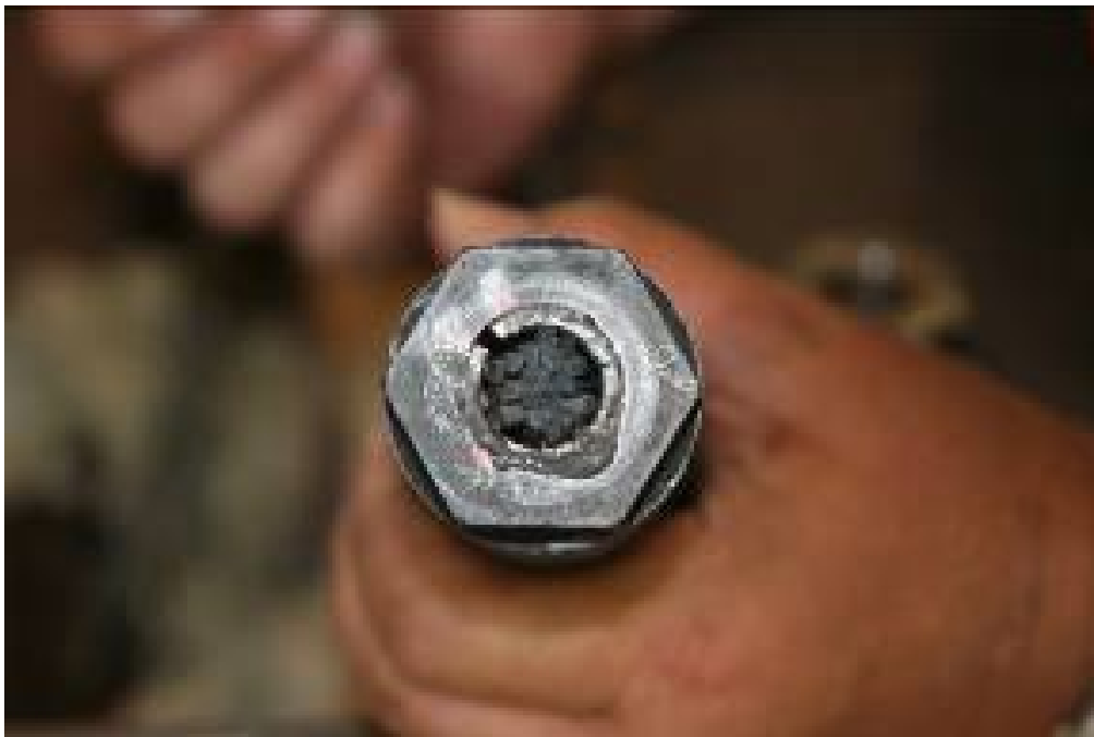
Figure 3.14. Precision Sure-Lock Prototype 2 wire rope termination B (end view) after test S5.
