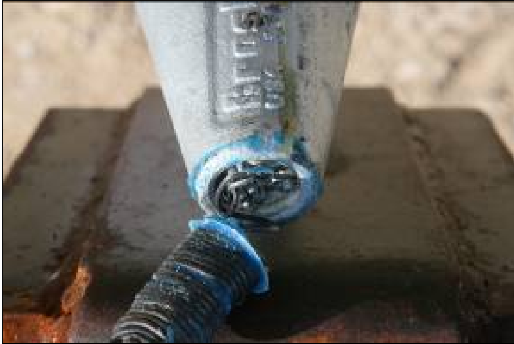
Figure 3.21. Epoxy Socket wire rope termination A after test P1.
