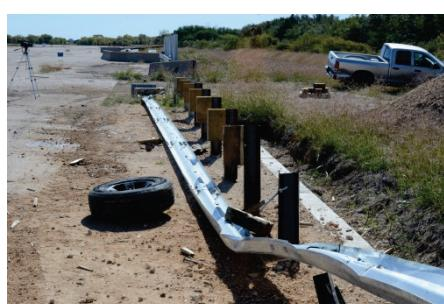
W-Beam Guardrail on Low-Fill Box Culvert after Test
