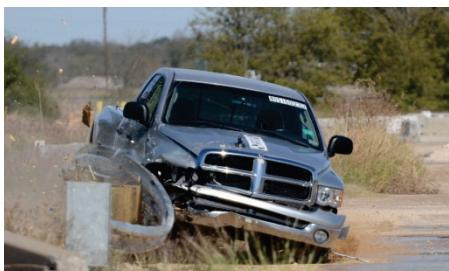
2270P Vehicle Redirecting during Test with W-Beam Guardrail over Low-Fill Box Culvert
