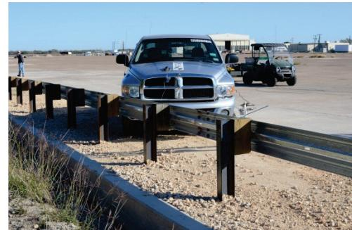
**31-inch W-Beam Guardrail on Low-Fill Box Culvert**
