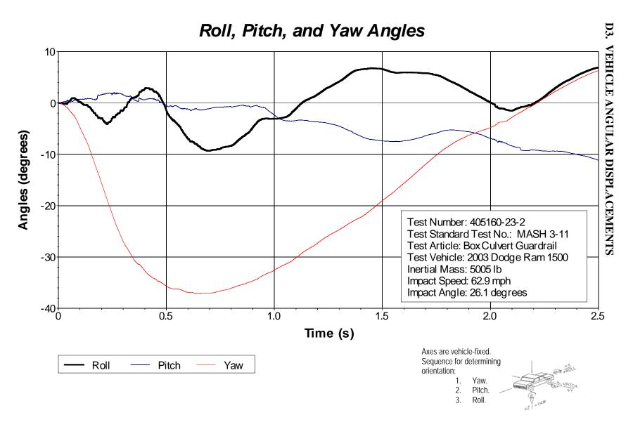
Figure D2. Vehicle angular displacements for test 405160-23-2.
