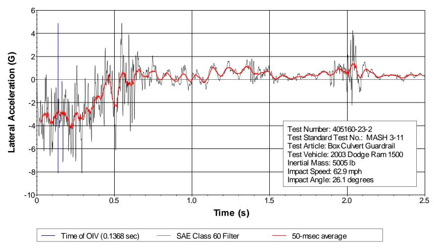
Figure D4. Vehicle lateral accelerometer trace for test 405160-23-2 (accelerometer located at center of gravity).
