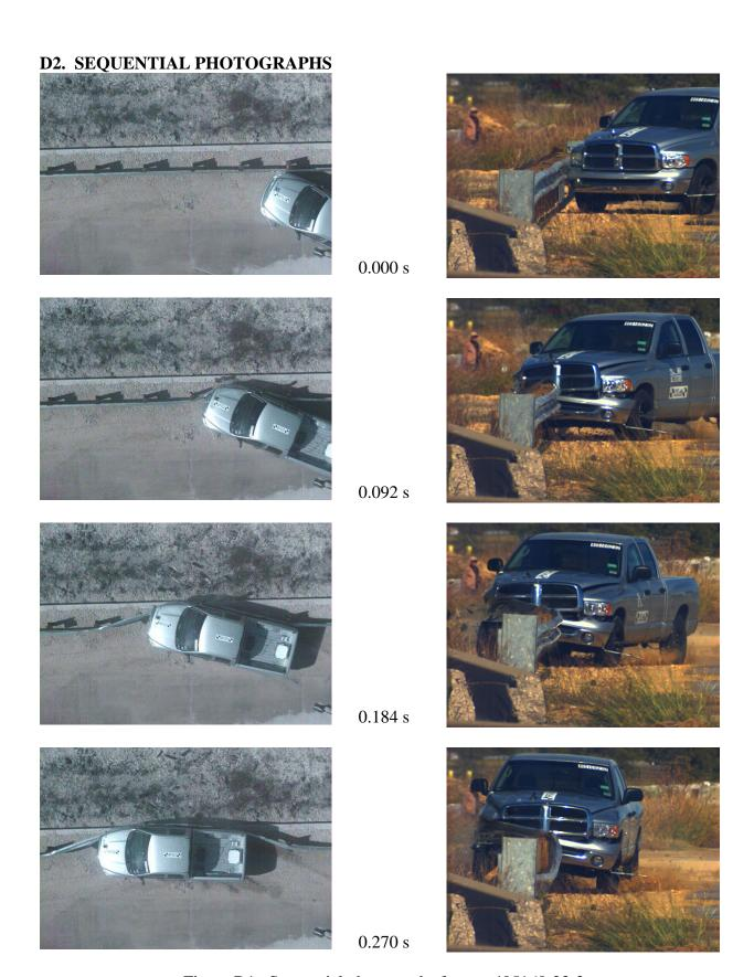
Figure D1. Sequential photographs for test 405160-23-2 (overhead and frontal views).
