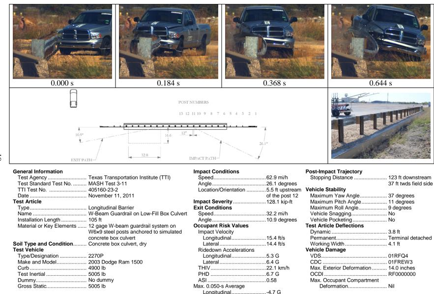
Figure 5.7. Summary of results for MASH test 3-11 on the W-Beam Guardrail on Low-Fill Box Culvert.
