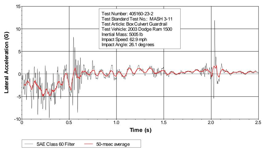
Figure D7. Vehicle lateral accelerometer trace for test 405160-23-2 (accelerometer located over rear axle).
