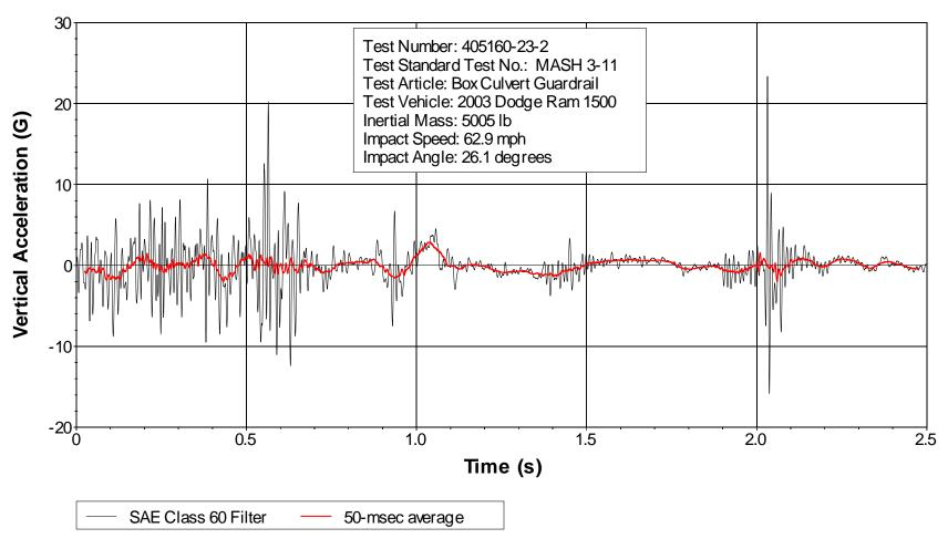
Figure D8. Vehicle vertical accelerometer trace for test 405160-23-2 (accelerometer located over rear axle).
