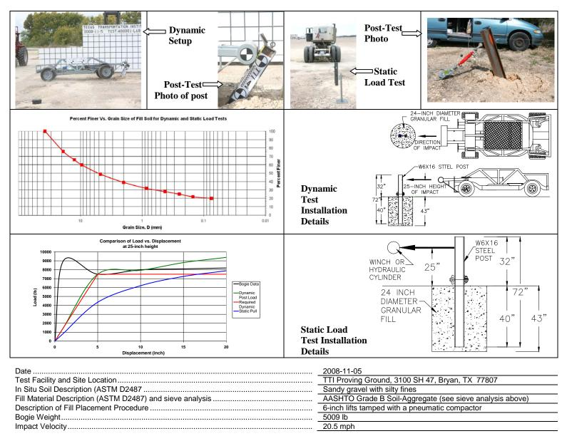
Figure C2. Summary of strong soil test results for establishing installation procedure.
