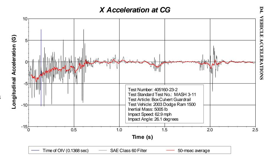
Figure D3. Vehicle longitudinal accelerometer trace for test 405160-23-2 (accelerometer located at center of gravity).
