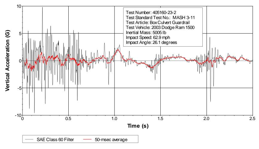
Figure D5. Vehicle vertical accelerometer trace for test 405160-23-2 (accelerometer located at center of gravity).
