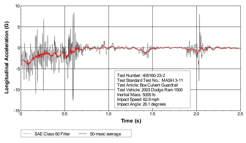
Figure D6. Vehicle longitudinal accelerometer trace for test 405160-23-2 (accelerometer located over rear axle).
