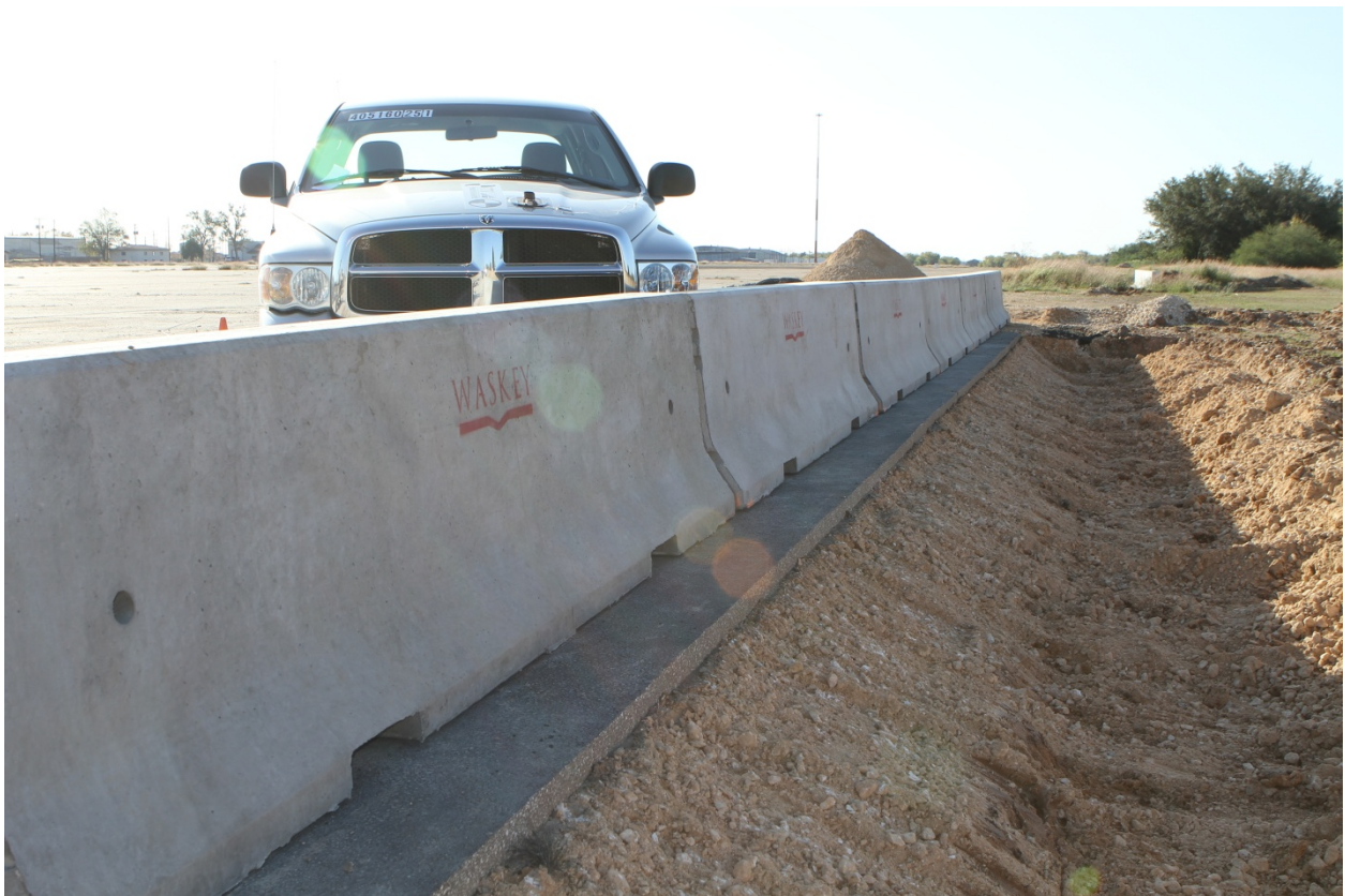
Figure 6.1. Vehicle/installation geometrics for test 405160-25-1.
