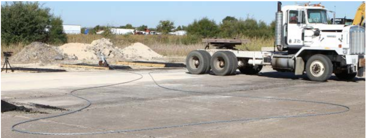
Figure 2.3. Test set up for dynamic pull testing of pins installed in asphalt.
