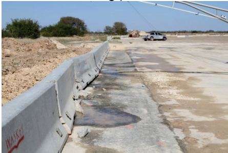
Pinned barrier and vehicle after test
