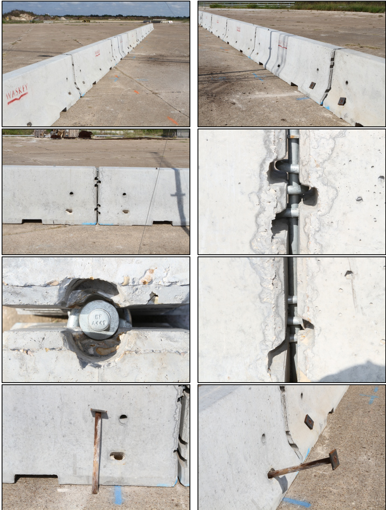
Figure 5.2. Transition from free-standing F-shape barrier to pinned F shape barrier prior to test 405160-26-2.
