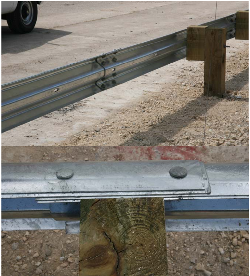
Figure 6. Long-Span Guardrail prior to testing.
