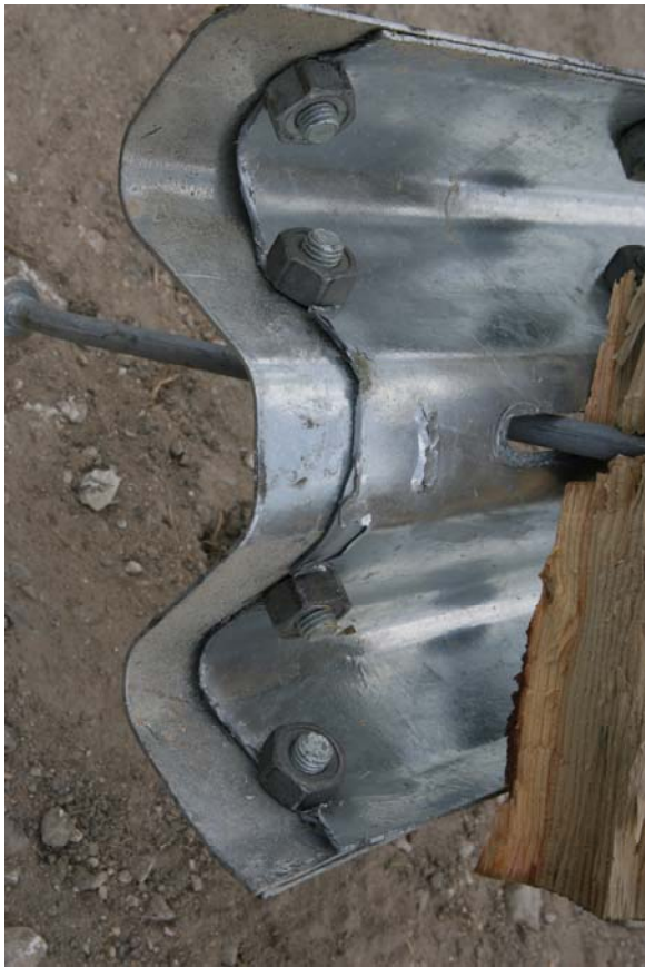
Figure 10. Installation after test 405160-1-1.
