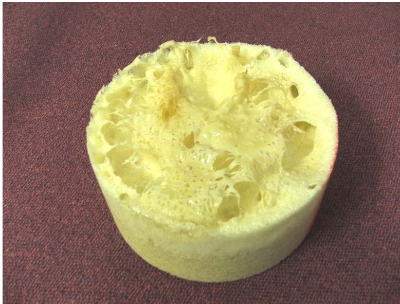
Figure 5: Foam sample – noticeable large voids found at bottom of cylindrical samples.
