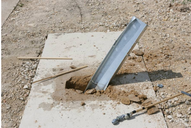
Figure 19: Post in standard two-sack grout after test B1.
