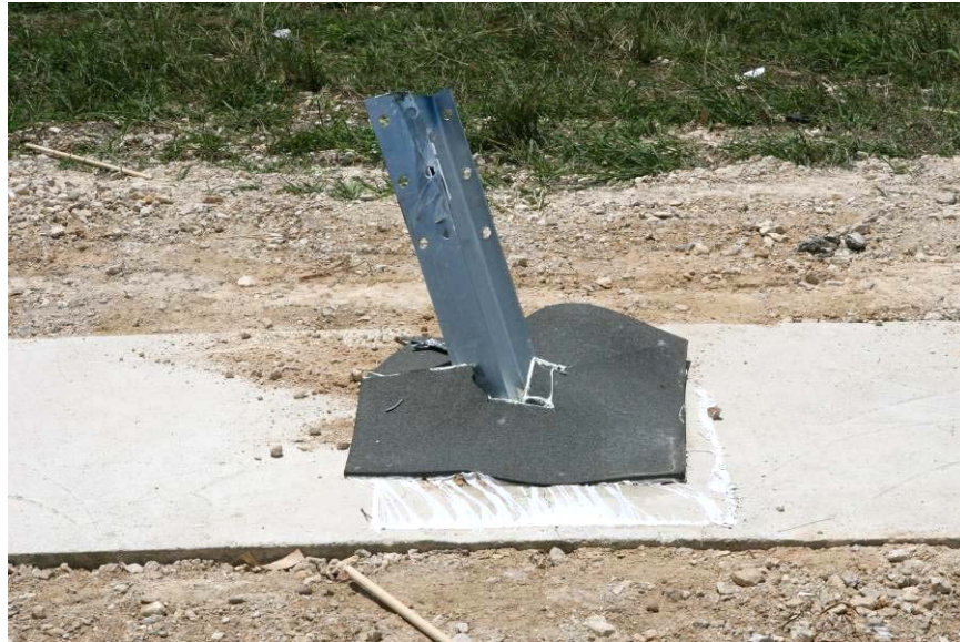
Figure 27: Post with flat mat after test B5.
