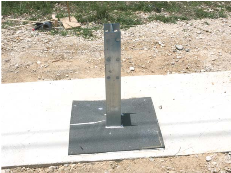
Figure 26: Post with flat mat prior to test B5.
