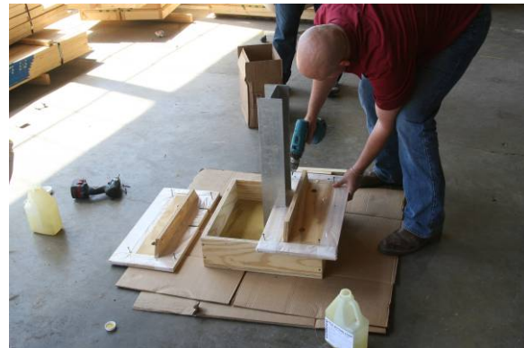
Figure 14: Installing top plates on mold after placement of foam mixture.
