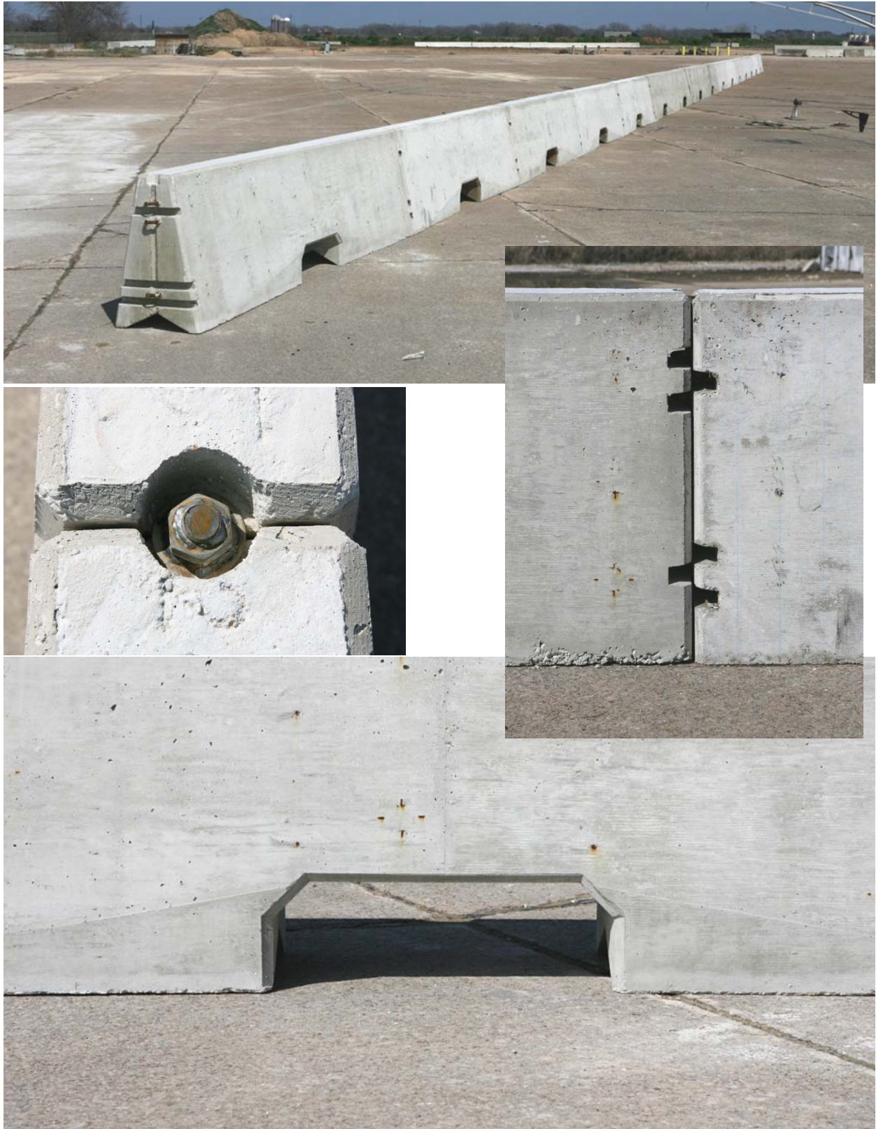
Figure 4.3. Washington DOT pin and loop concrete barrier with drainage slots prior to testing.
