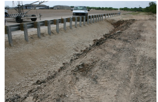
Modified G4(1S) W-Beam Guardrail on 2H:1V Slope
