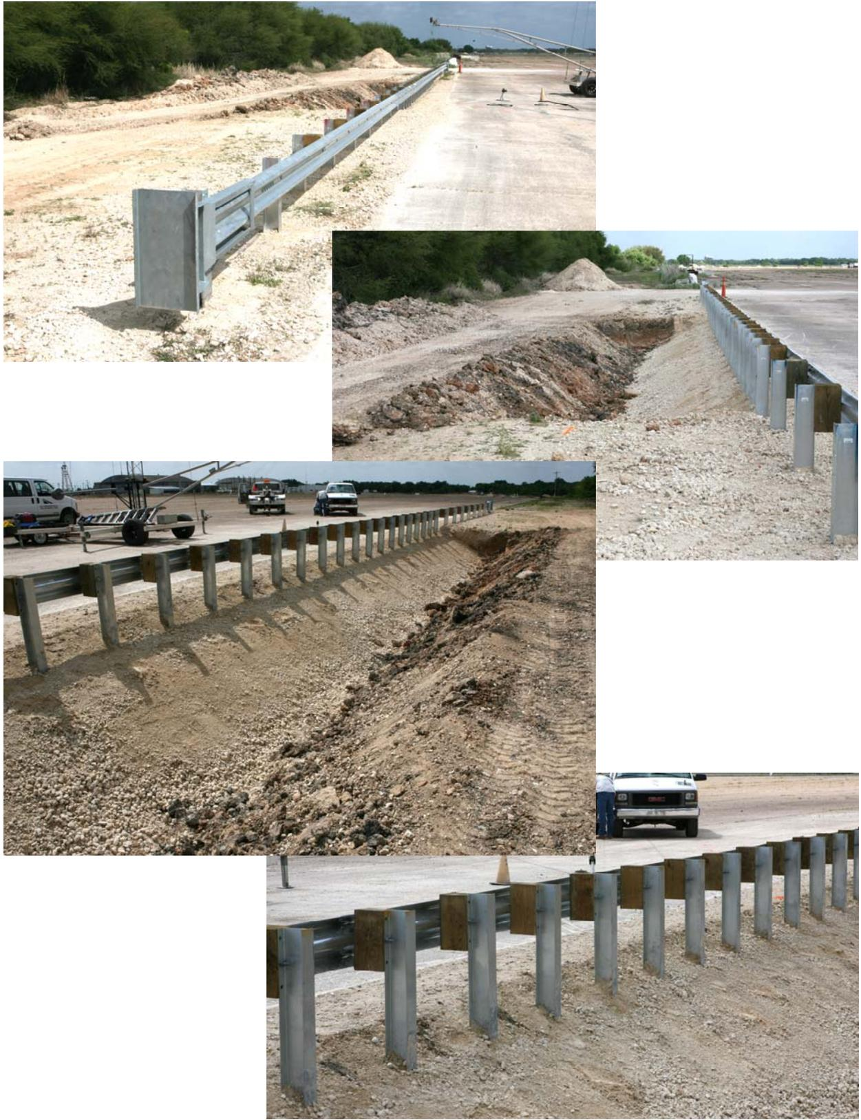
Figure 3.12. Guardrail on 2H:1V slope prior to testing.
