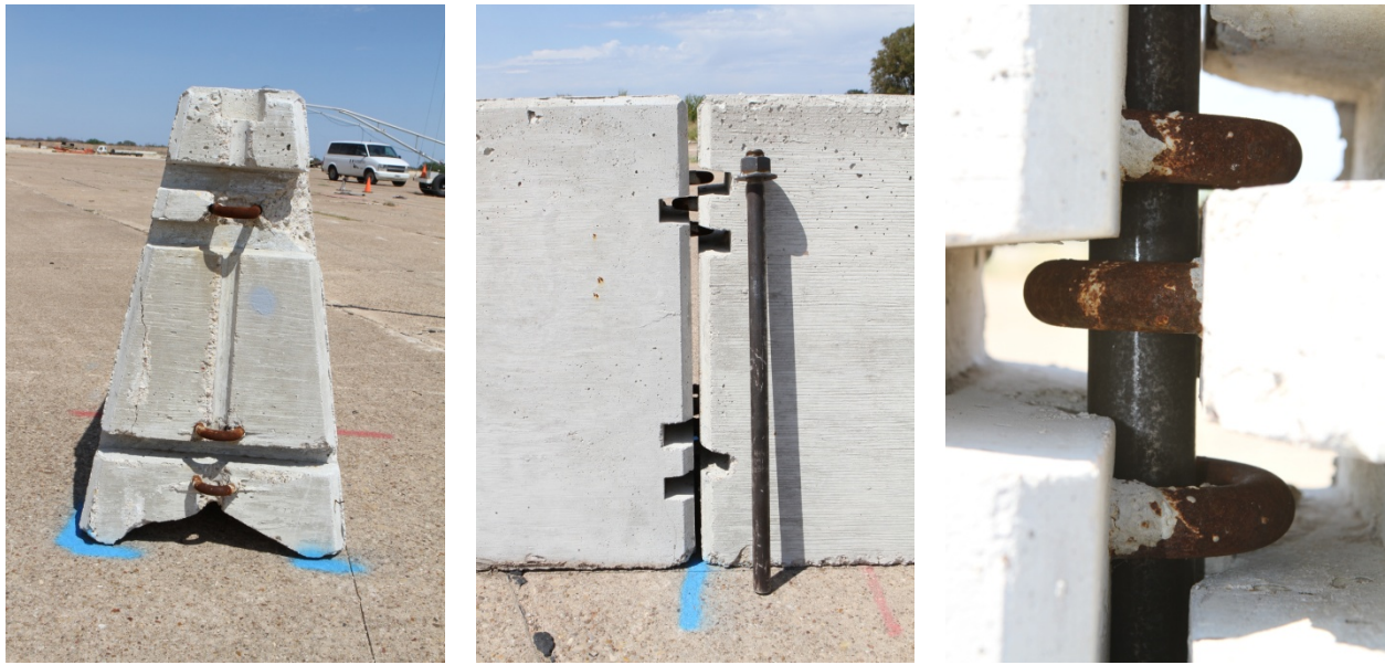
Figure 1. WSDOT pin and loop barrier with drainage slots before test 405160-30-1 (continued).
