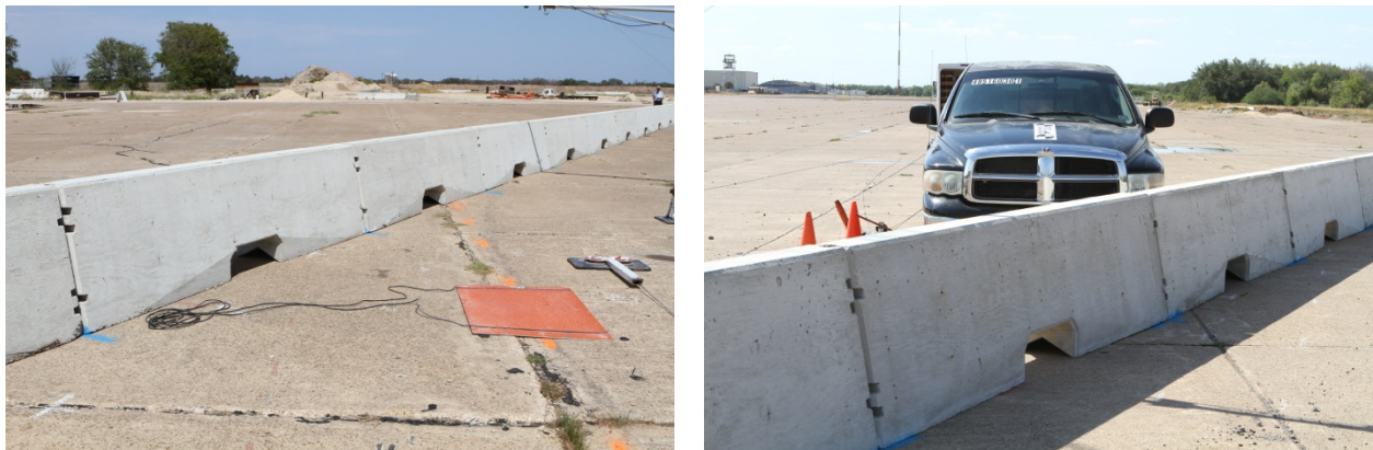
Figure 1. WSDOT pin and loop barrier with drainage slots before test 405160-30-1.
