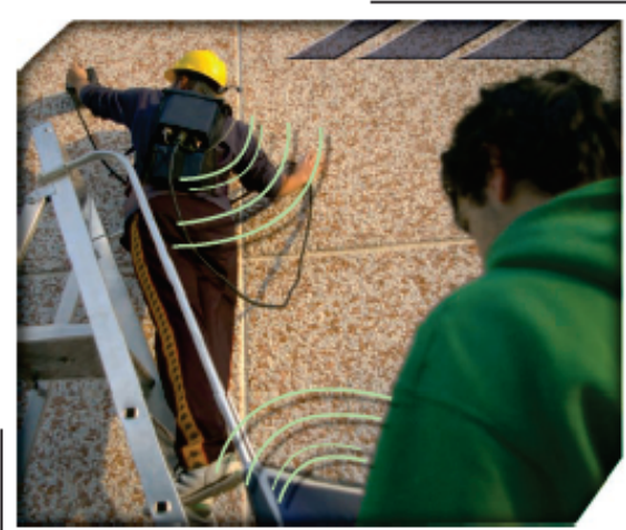
Wireless link between control unit and data logger permits easy operations in less than ideal situations
