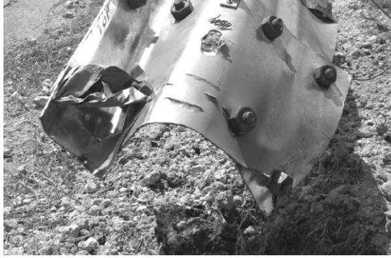
Figure 3.8: Rail rupture in TTI test with instrumented W-beam guardrail
