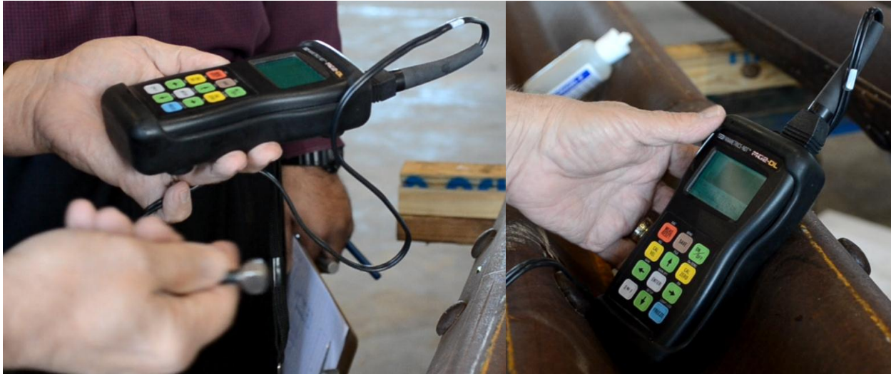
Figure 3.1 Handheld ultrasonic thickness gauge with probe.
