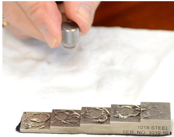
Figure 3.2 Calibration steel block.
