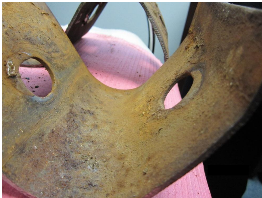
Figure 3.7 Debris and rust collected between lapped splices of the samples used.
