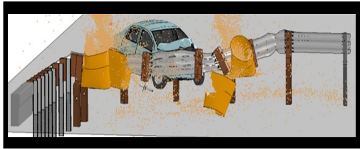
Figure 2: FE Simulation of MASH TL 3-32 Small Car Impact
