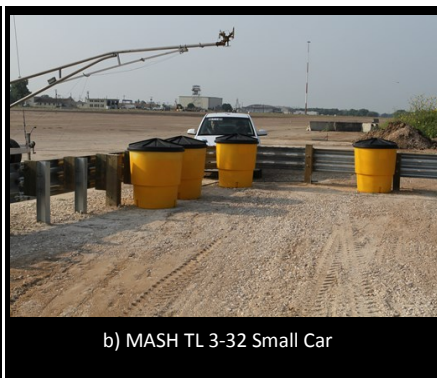
Figure 4: MASH TL-3 Full-scale Crash Test Set-ups
