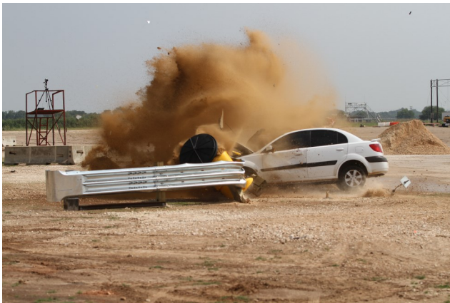
Figure 3: Full-scale Crash Test of MASH TL 3-32 Small Car at Impact
