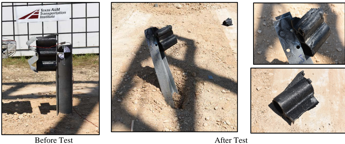
Figure 3. Plastic King™ Block B Raised 4 inches before and after Test No. 605311-P3.
