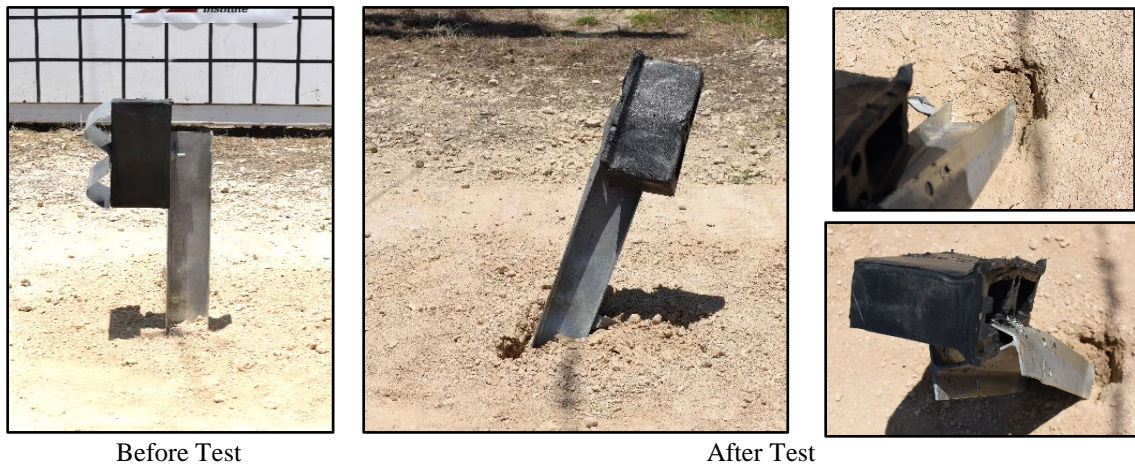
Figure 7. Mondo Plastic Block Raised 4 inches before and after Test No. 605311-P7.
