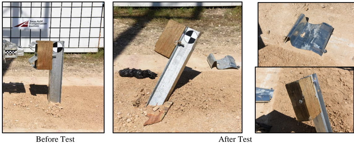
Figure 2. Wood Block A at Standard Height before and after Test No. 605311-P2.
