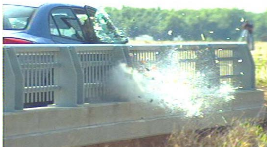
Figure C2. Sequential Photographs for Test No. 490022-2 (Rear of Bridge Rail View).
