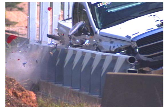
Figure D1. Sequential Photographs for Test No. 490022-3 (Overhead and Frontal Views) (continued).
