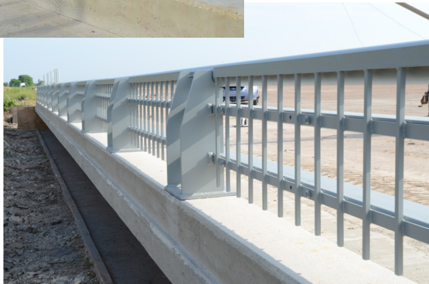
Figure 2.3. TxDOT Picket Rail before Testing.
