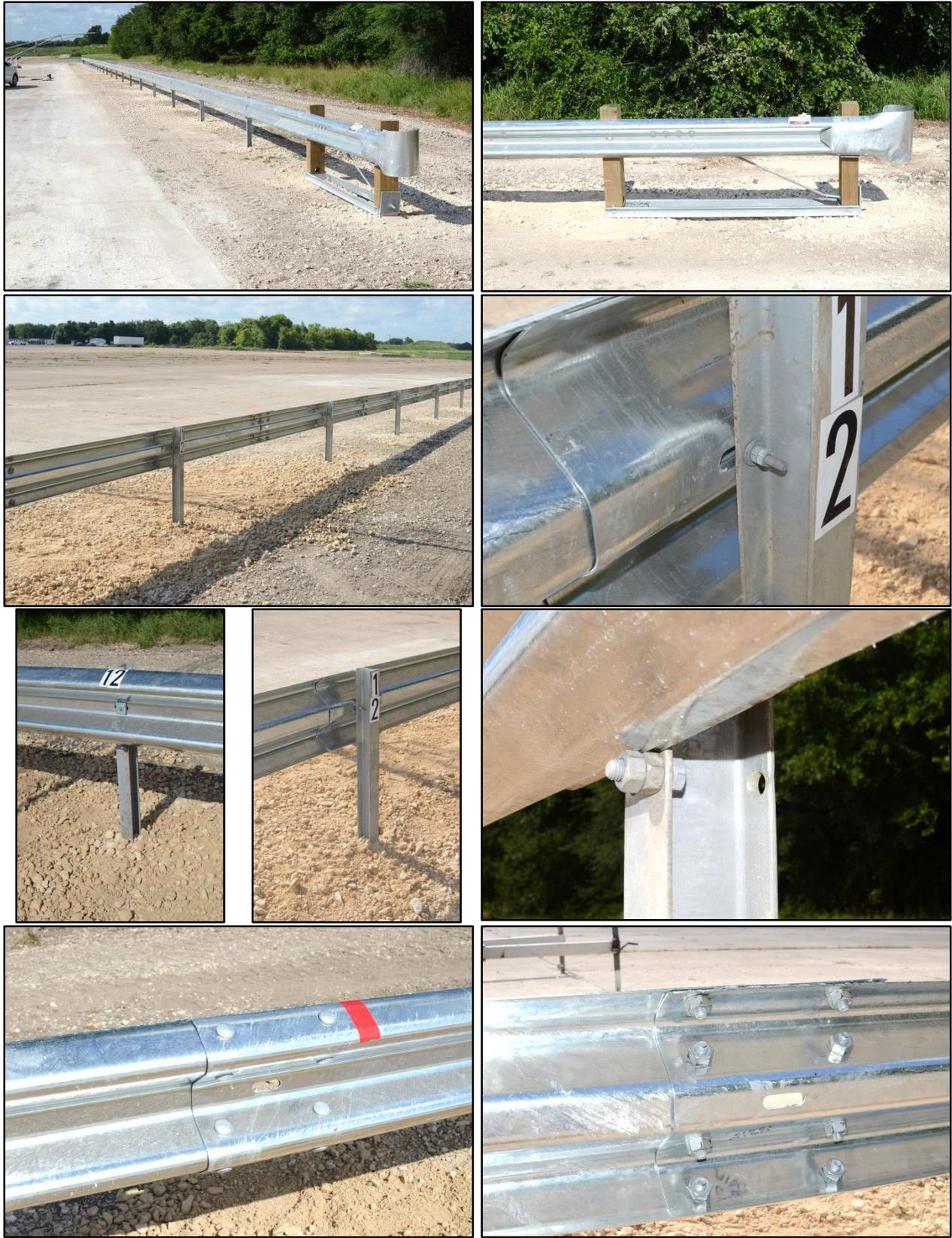
**Figure 2.2. G2 Weak Post W-Beam Guardrail System prior to Testing.**
