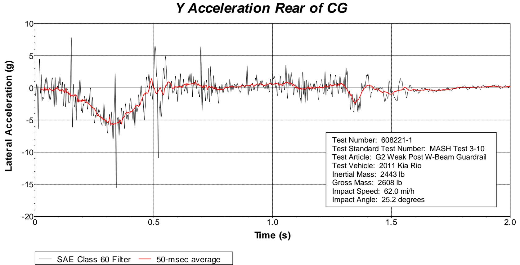
**Figure D.8. Vehicle Lateral Accelerometer Trace for Test No. 608221-1
