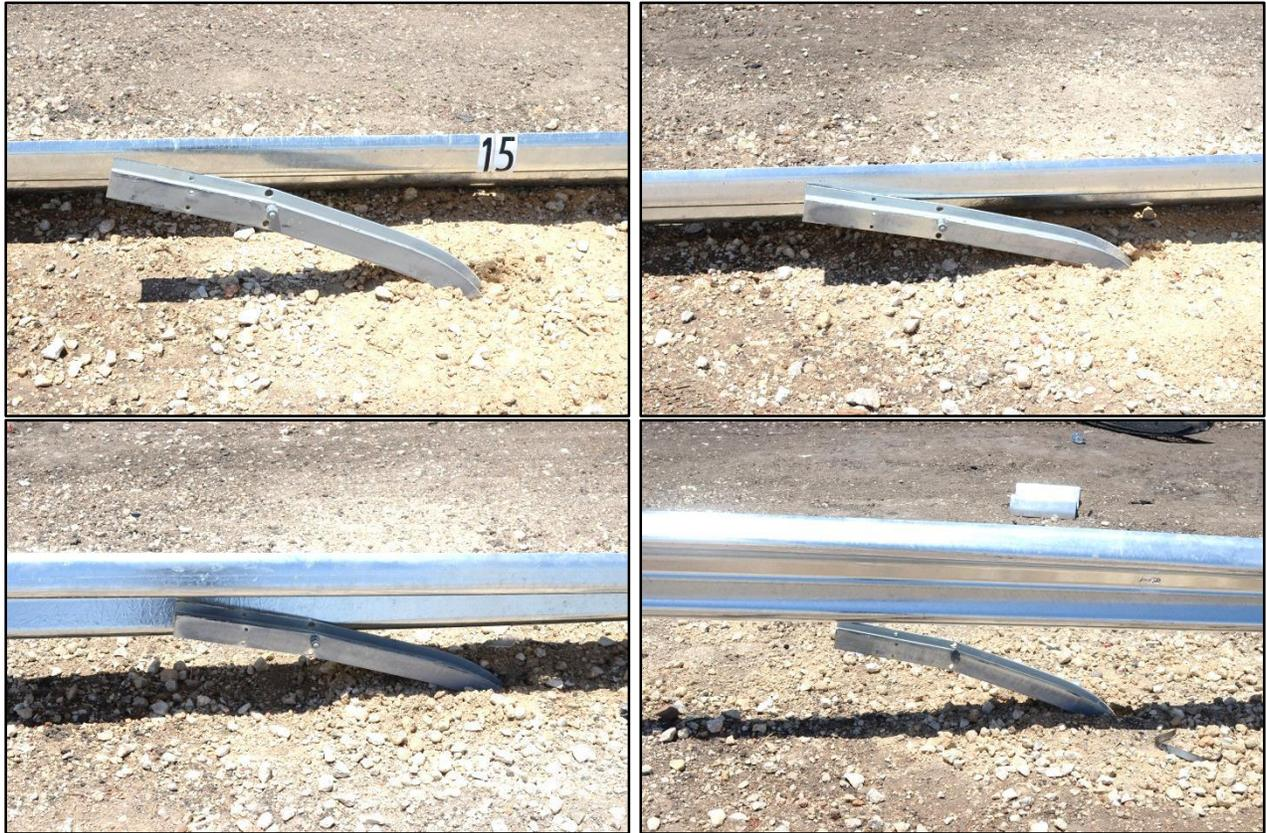
**Figure 5.6. Posts 15 through 18 after Test No. 608221-1.**
