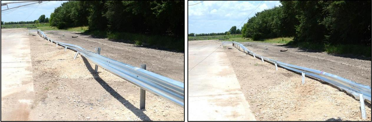
**Figure 5.4. G2 Weak Post W-Beam Guardrail System after Test No. 608221-1.**
