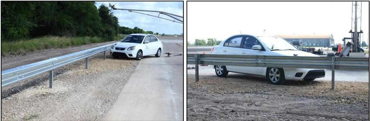
**Figure 5.1. G2 Weak Post W-Beam Guardrail System/Test Vehicle Geometrics for Test No. 608221-1.**
