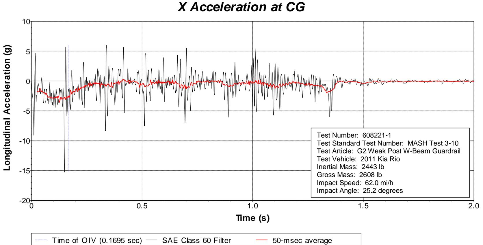
**Figure D.4. Vehicle Longitudinal Accelerometer Trace for Test No. 608221-1 (Accelerometer Located at Center of Gravity).**
