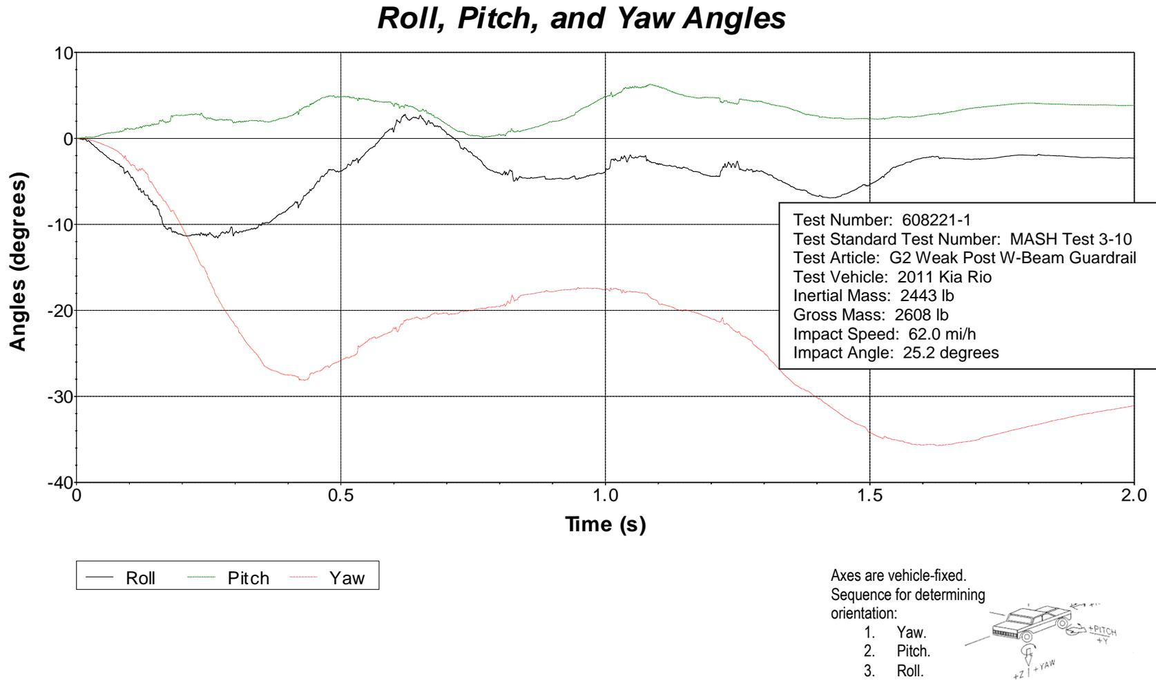
Figure D.3. Vehicle Angular Displacements for Test No. 608221-1.
