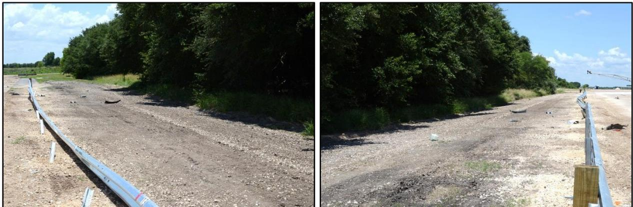
**Figure 5.7. Field Side of G2 Weak Post W-Beam Guardrail System after Test No. 608221-1.**
