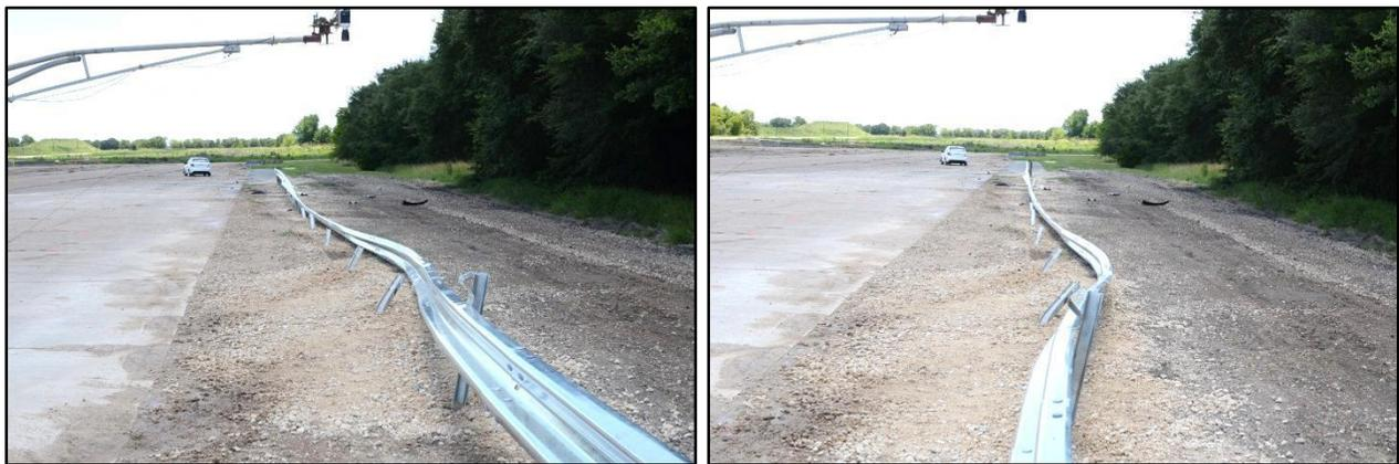
**Figure 5.3. G2 Weak Post W-Beam Guardrail System and Test Vehicle after Test No. 608221-1.**
