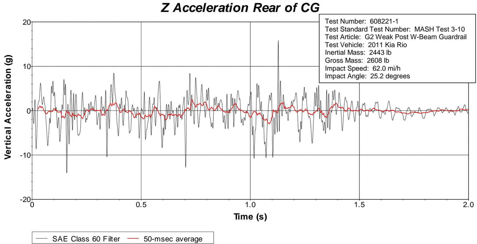
**Figure D.9. Vehicle Vertical Accelerometer Trace for Test No. 608221-1
