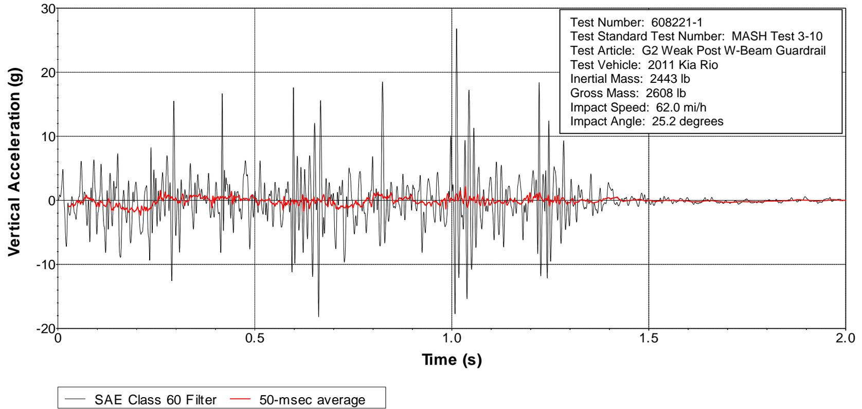
**Figure D.6. Vehicle Vertical Accelerometer Trace for Test No. 608221-1 (Accelerometer Located at Center of Gravity).**
