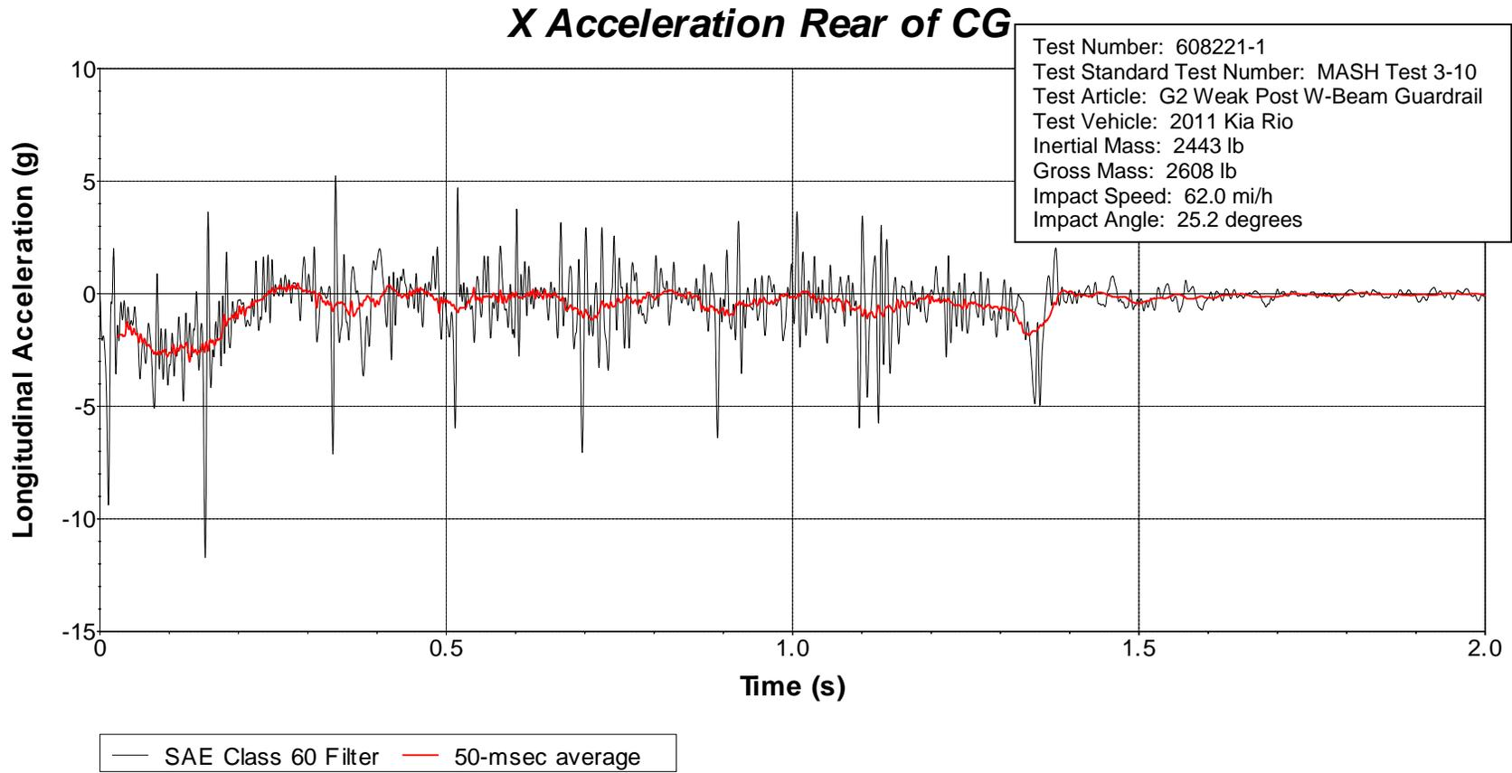
**Figure D.7. Vehicle Longitudinal Accelerometer Trace for Test No. 608221-1
