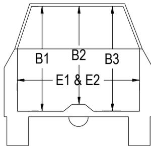
**OCCUPANT COMPARTMENT DEFORMATION MEASUREMENT**
