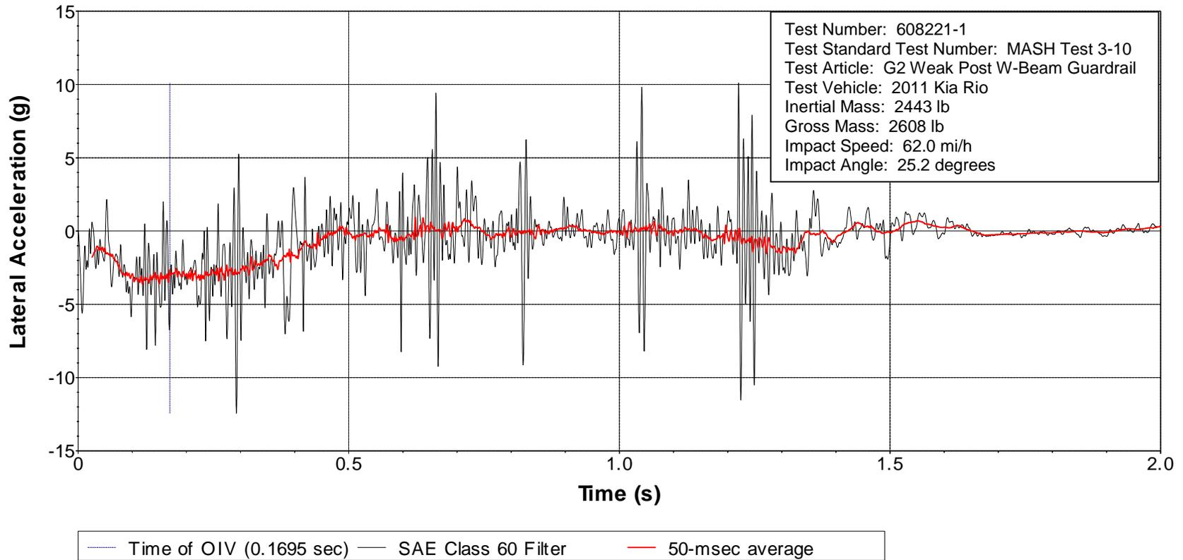
**Figure D.5. Vehicle Lateral Accelerometer Trace for Test No. 608221-1 (Accelerometer Located at Center of Gravity).**
