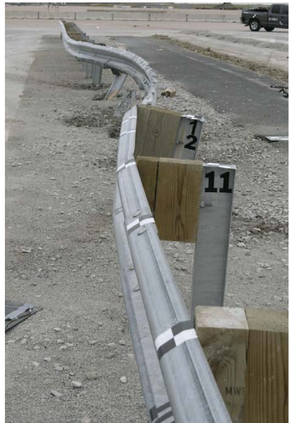
Figure 23. Midwest Guardrail System Barrier Damage, Test 2214MG-2
