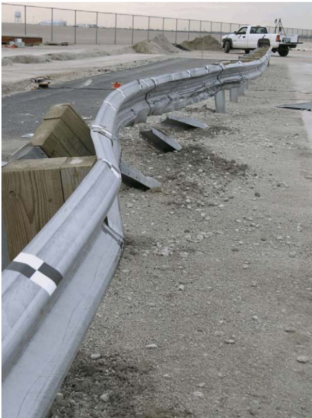
Figure 23. Midwest Guardrail System Barrier Damage, Test 2214MG-2
