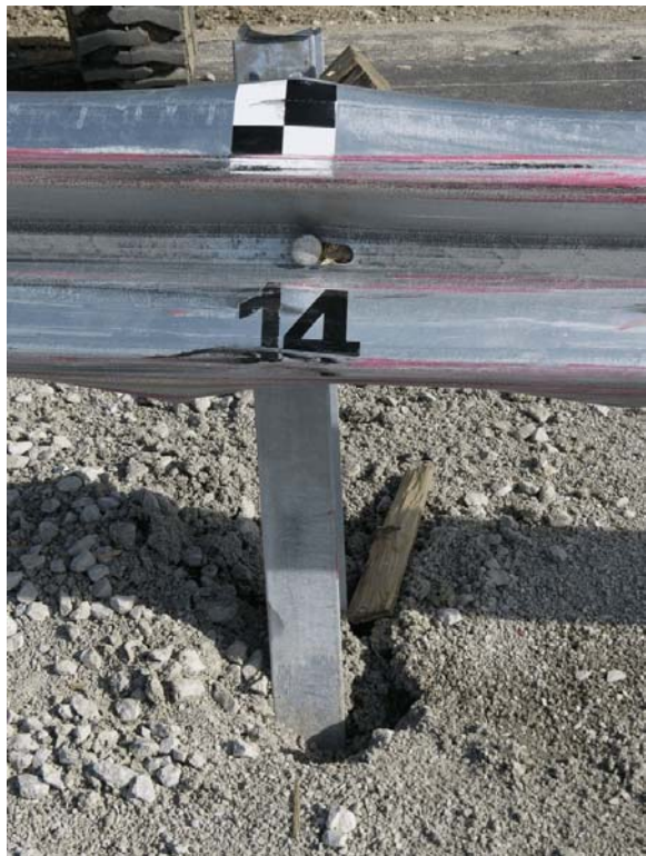
Figure 22. System Damage - Post Nos. 13 and 14, Test 2214MG-3
