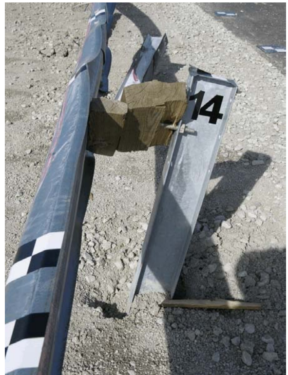
Figure 22. System Damage - Post Nos. 13 and 14, Test 2214MG-3
